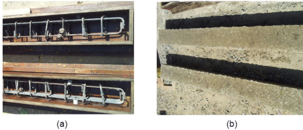
Figure 5.8: Formwork and Reinforcement Cage of RC Specimens.
