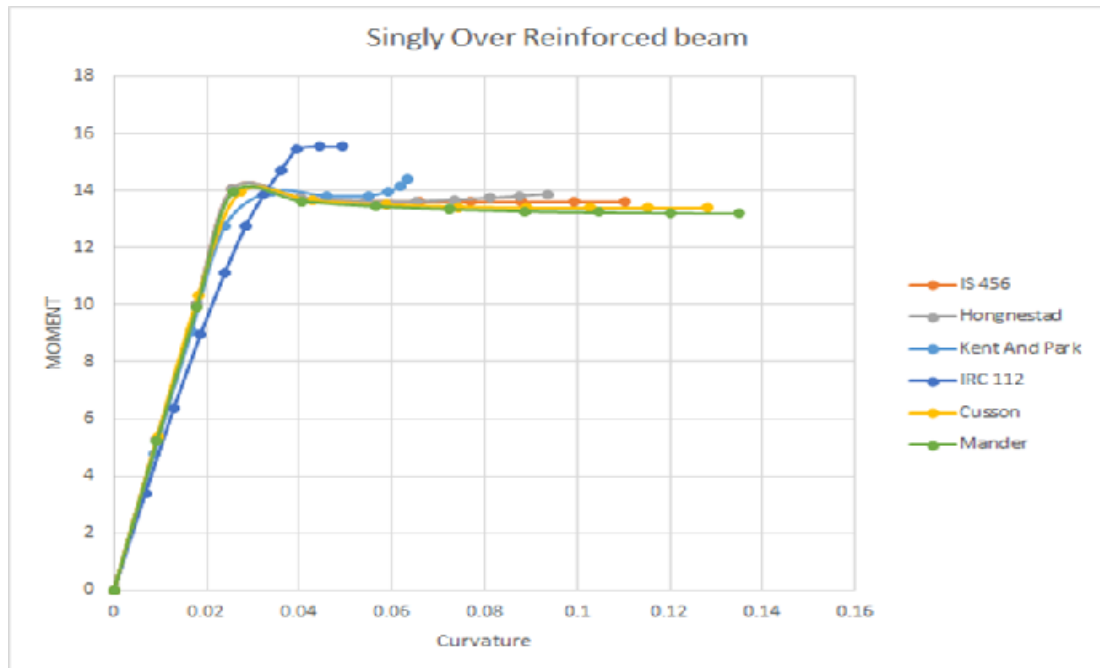
Figure 4.7: Moment-Curvature for Singly Over Reinforced Beam
