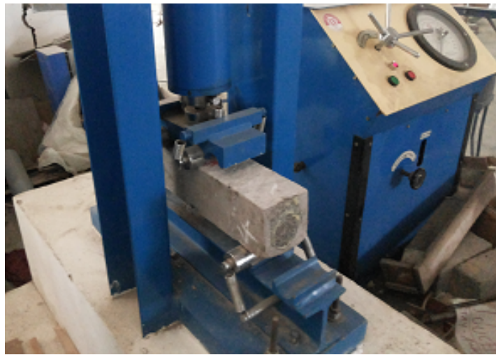
Figure 3.6: Testing of Flexural strength
