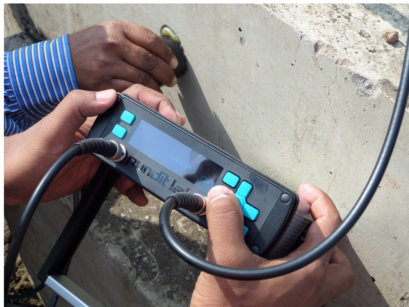
Figure 3.16: UPV testing of RCC members in Laboratory
