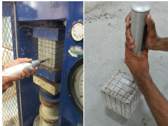
Figure 3.9: Rebound hammer in horizontal and Horizontal position for cube
