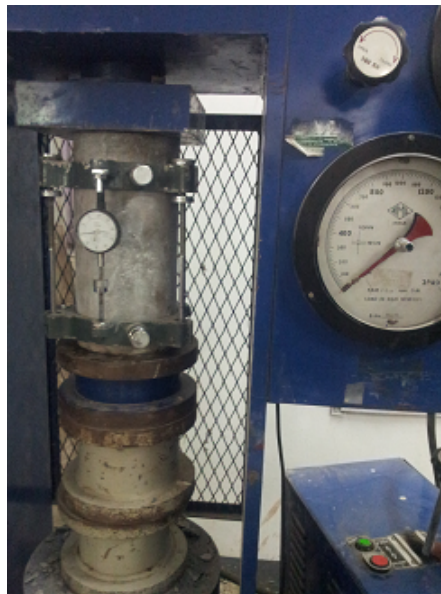
Figure 3.8: Testing of Modulus of Elasticity
