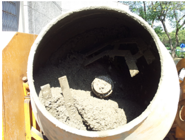
Figure 3.1: Drum mixture for mixing of concrete
