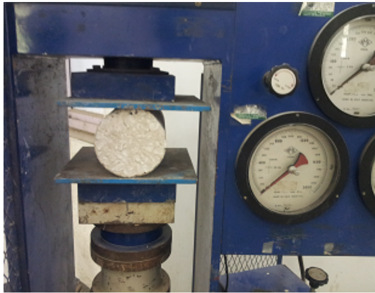
Figure 3.7: Testing of Split tensile strength
