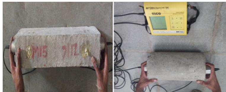
Figure 3.12: UPV testing of Beam and cylinder specimen by Direct method
