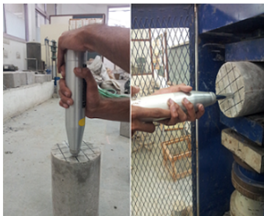
Figure 3.10: Rebound hammer in Vertical and Horizontal position for cylinder
