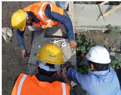
Figure 3.14: UPV testing of RCC members on site
