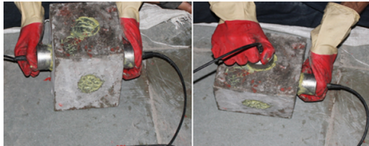
Figure 3.11: UPV testing of cube specimen by Direct and Semi direct method
