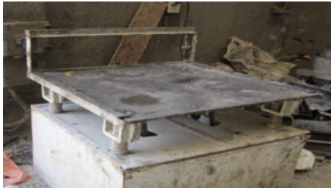
Figure 3.2: Table vibrator for compacting concrete mix
