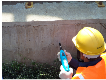
Figure 3.13: Surface hardness testing of RCC members on site
