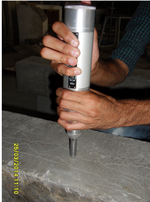
Figure 3.15: Surface hardness testing of RCC members in Laboratory
