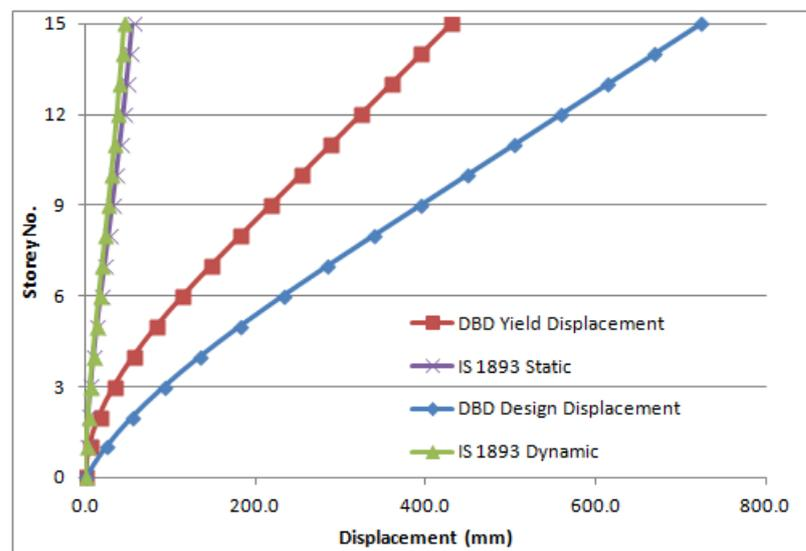
Figure 5.28: Displacement Comparison among FBD and DBD - X Direction -  $\beta_F = 0.4$
