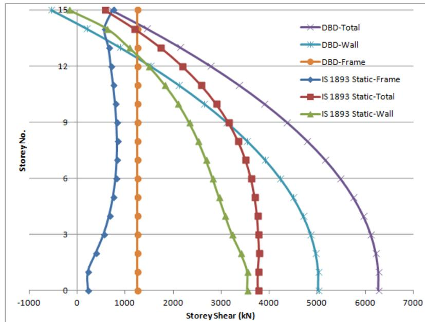
Figure 5.9: Storey Shear Distribution between Frames and Walls by FBD and DBD - X Direction  $-\beta_F = 0.2$
