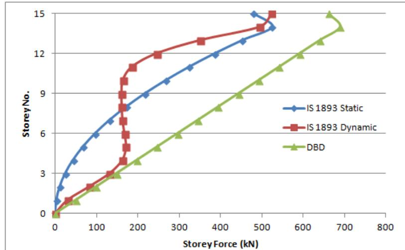
Figure 5.12: Lateral Forces Comparison among FBD and DBD- Y Direction -  $\beta_F = 0.2$
