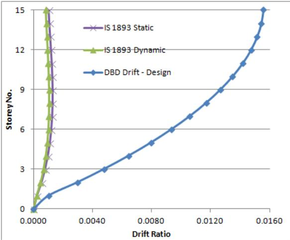
Figure 4.4: Drift Variation by FBD and DBD - X -Direction
