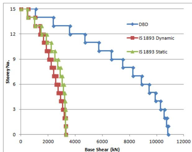
Figure 4.11: Variation of the Storey Shear across the height- Y -Direction
