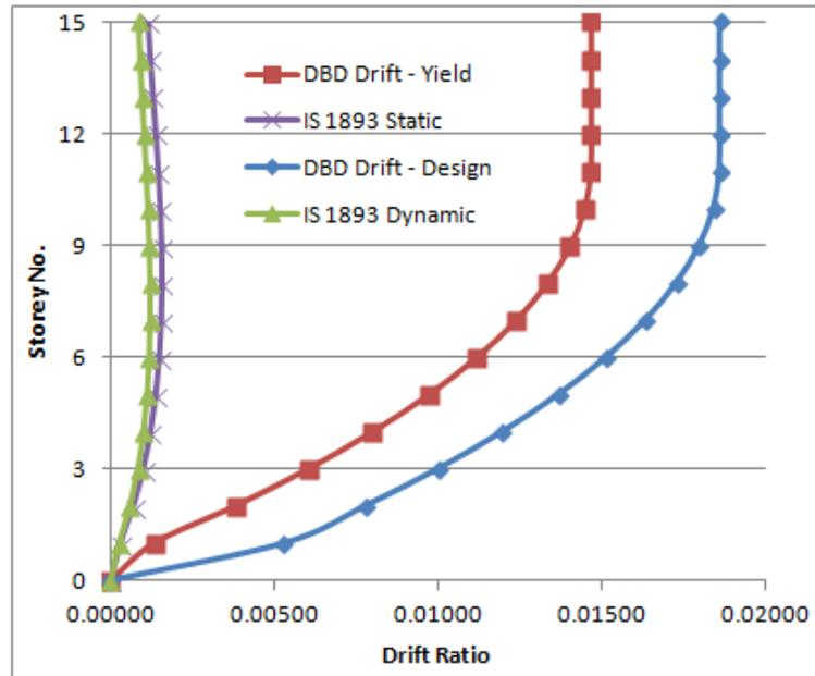
Figure 5.17: Drift Comparison among FBD and DBD - X Direction  $-\beta_F = 0.3$
