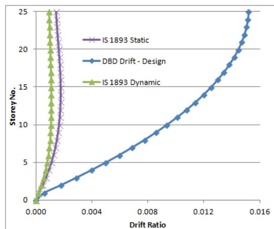
Figure 4.19: Drift Variation by FBD and DBD - Y -Direction
