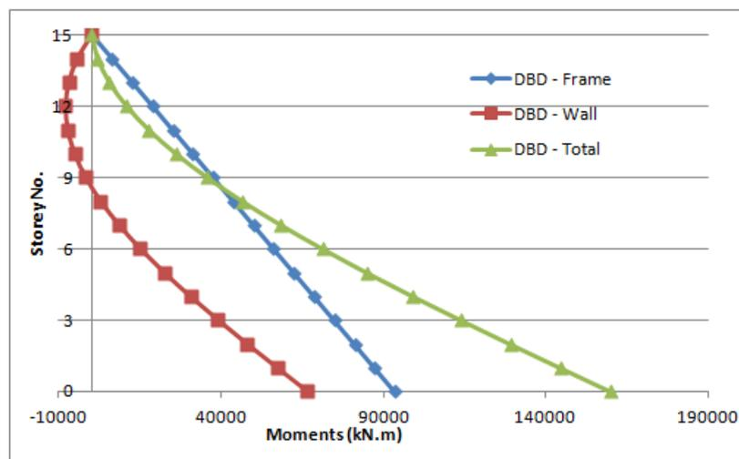
Figure 5.32: Overturning Moment Distribution for DBD - X Direction -  $\beta_F = 0.4$
