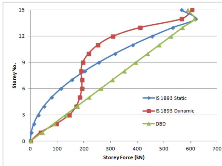
Figure 5.30: Lateral Forces Comparison among FBD and DBD- X Direction -  $\beta_F = 0.4$
