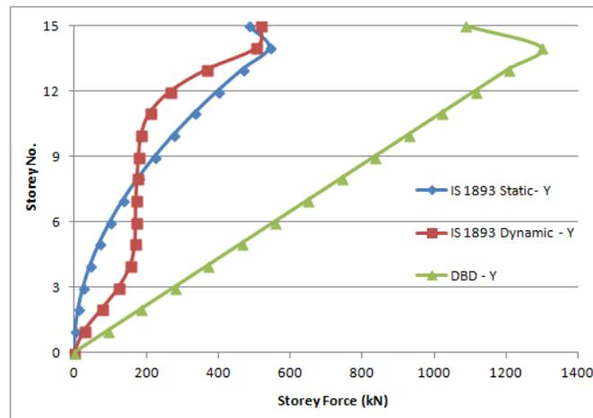
Figure 4.10: Lateral Forces Comparison by FBD and DBD - Y -Direction
