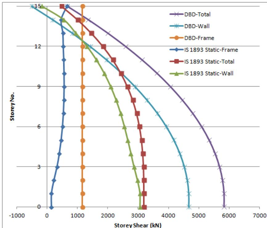
Figure 5.15: Storey Shear Distribution between Frames and Walls by FBD and DBD - Y Direction -  $\beta_F = 0.2$
