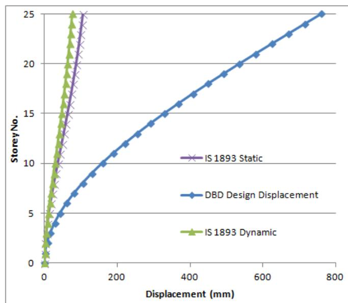
Figure 4.13: Displacement Comparison by FBD and DBD- X -Direction
