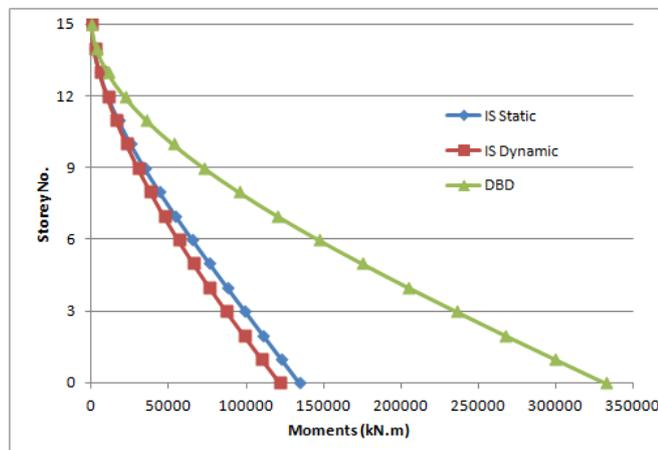
Figure 4.7: Overturning Moment Comparison - X -Direction
