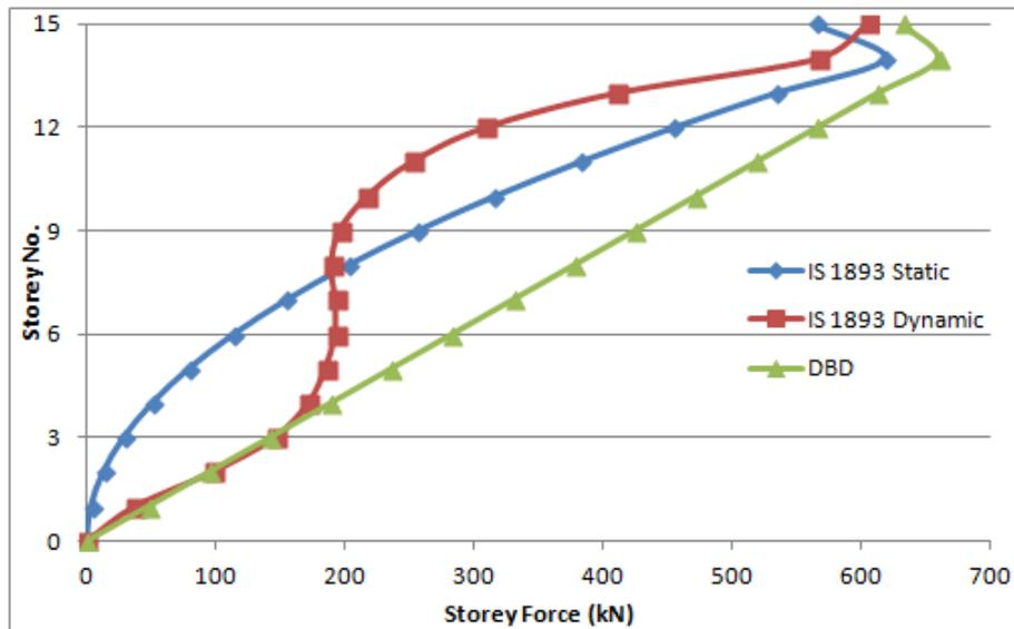
Figure 5.18: Lateral Forces Comparison among FBD and DBD- X Direction -  $\beta_F = 0.3$
