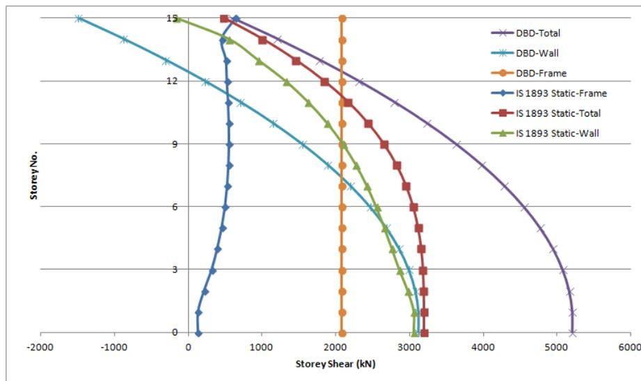
Figure 5.39: Storey Shear Distribution between Frames and Walls by FBD and DBD - Y Direction -  $\beta_F = 0.4$
