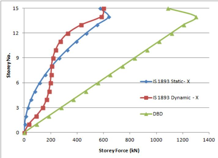
Figure 4.5: Lateral Forces Comparison by FBD and DBD - X -Direction
