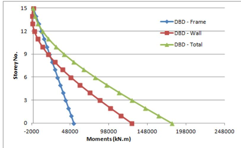
Figure 5.14: Overturning Moment Distribution for DBD - Y Direction -  $\beta_F = 0.2$
