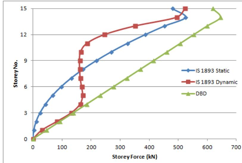
Figure 5.24: Lateral Forces Comparison among FBD and DBD- Y Direction -  $\beta_F = 0.3$
