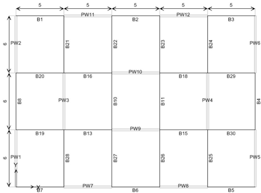
Figure 4.1: Plan of the Shear-Wall Building
