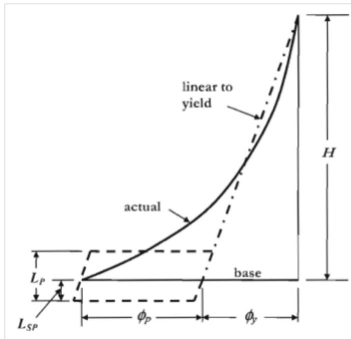
Figure 3.4: Idealization of Moment Curvature Distribution
