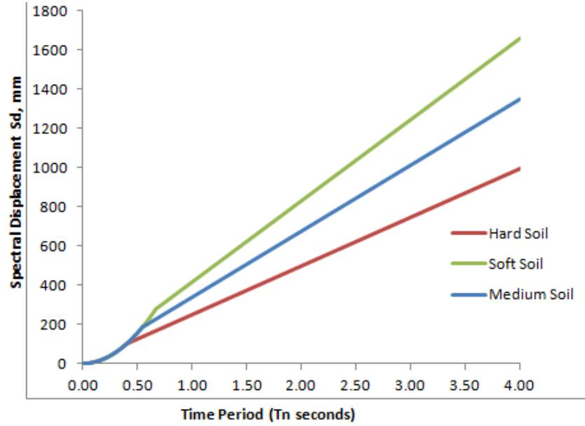
Figure 3.5: IS Code Design Displacement Spectra
