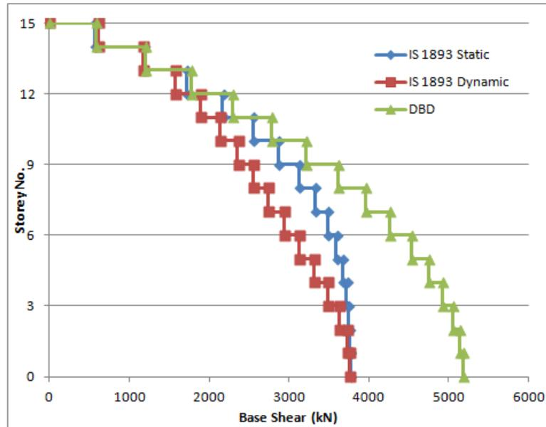
Figure 5.31: Storey Shear Comparison among FBD and DBD - X Direction -  $\beta_F = 0.4$
