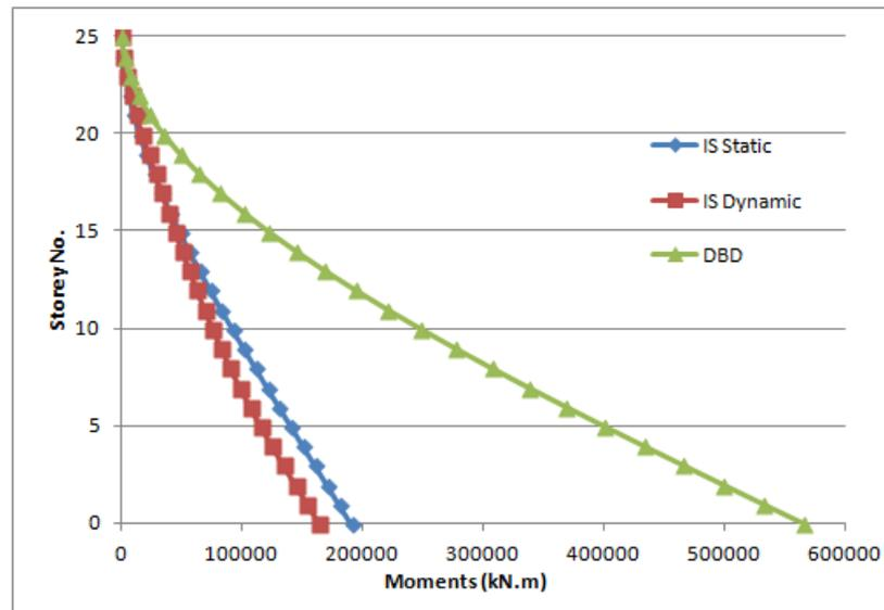
Figure 4.22: Overturning Moment Comparison - Y -Direction
