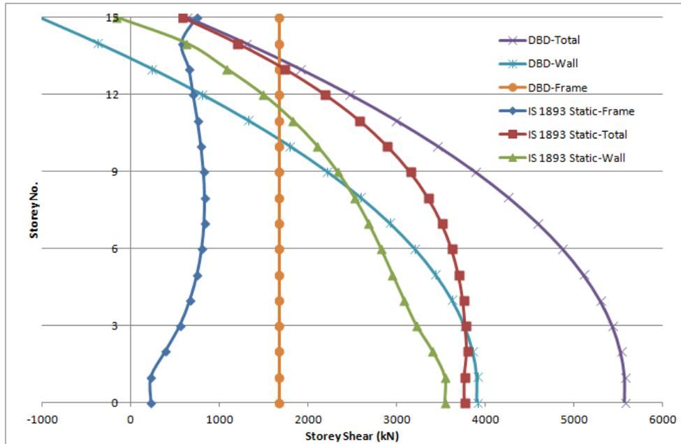
Figure 5.21: Storey Shear Distribution between Frames and Walls by FBD and DBD
