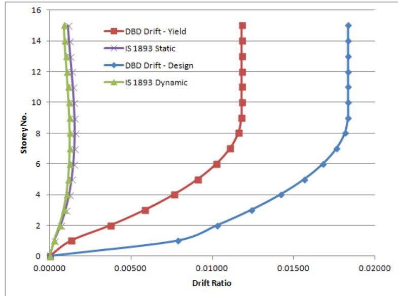
Figure 5.29: Drift Comparison among FBD and DBD - X Direction  $-\beta_F = 0.4$
