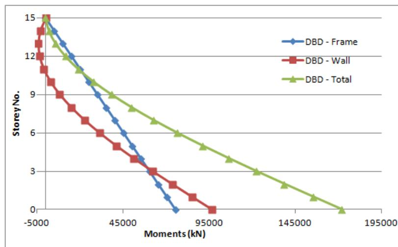
Figure 5.20: Overturning Moment Distribution for DBD - X -  $\beta_F = 0.3$
