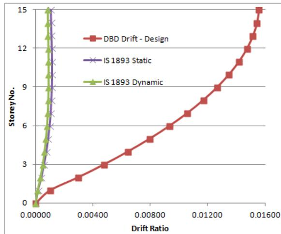
Figure 4.9: Drift Variation by FBD and DBD - Y -Direction
