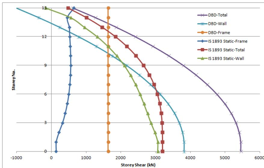
Figure 5.27: Storey Shear Distribution between Frames and Walls by FBD and DBD - Y Direction -  $\beta_F = 0.3$
