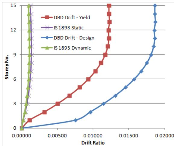
Figure 5.23: Drift Comparison among FBD and DBD - Y Direction - $\beta_F = 0.3$
