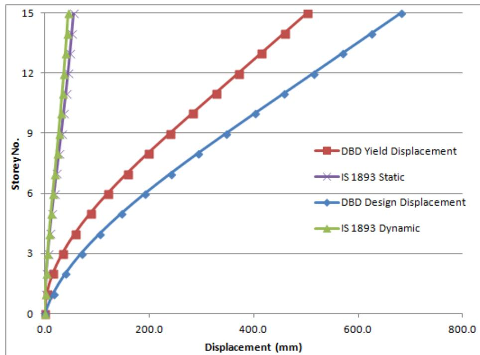
Figure 5.16: Displacement Comparison among FBD and DBD - X Direction -  $\beta_F = 0.3$
