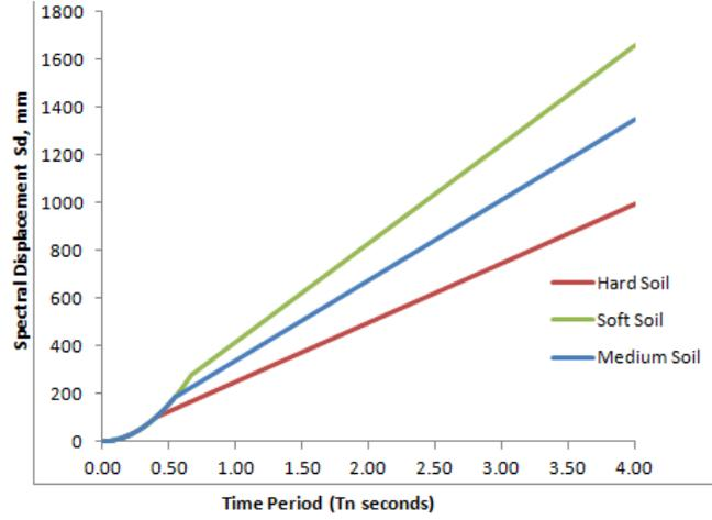
Figure 3.2: IS Design Displacement Spectrum
