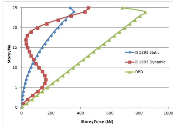
Figure 4.20: Lateral Forces Comparison by FBD and DBD - Y -Direction
