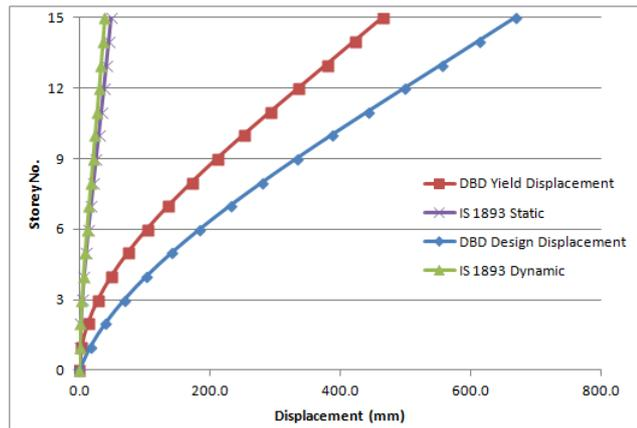
Figure 5.10: Displacement Comparison among FBD and DBD- Y-Direction- $\beta_F = 0.2$
