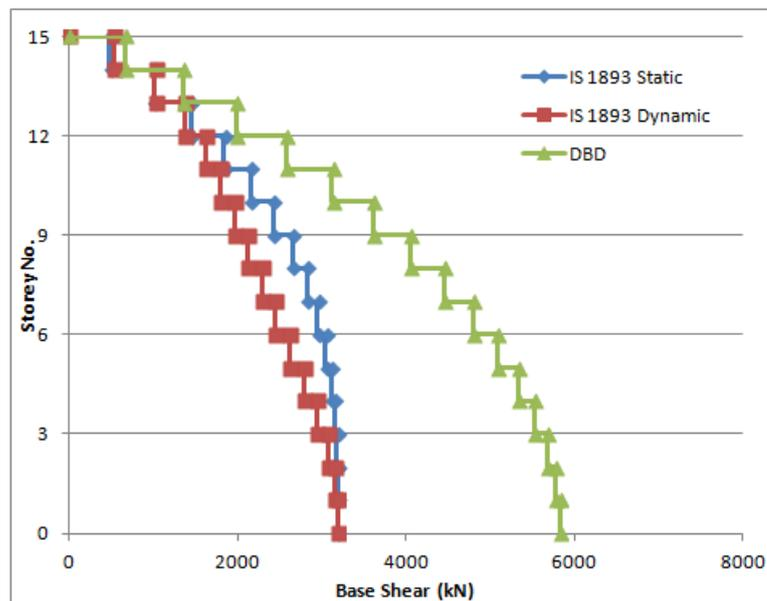
Figure 5.13: Storey Shear Comparison among FBD and DBD - Y Direction -  $\beta_F = 0.2$
