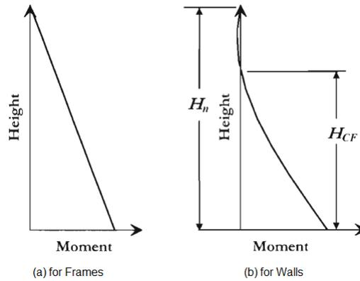
Figure 5.3: Moment Profile for (a) Frame and (b) Walls
