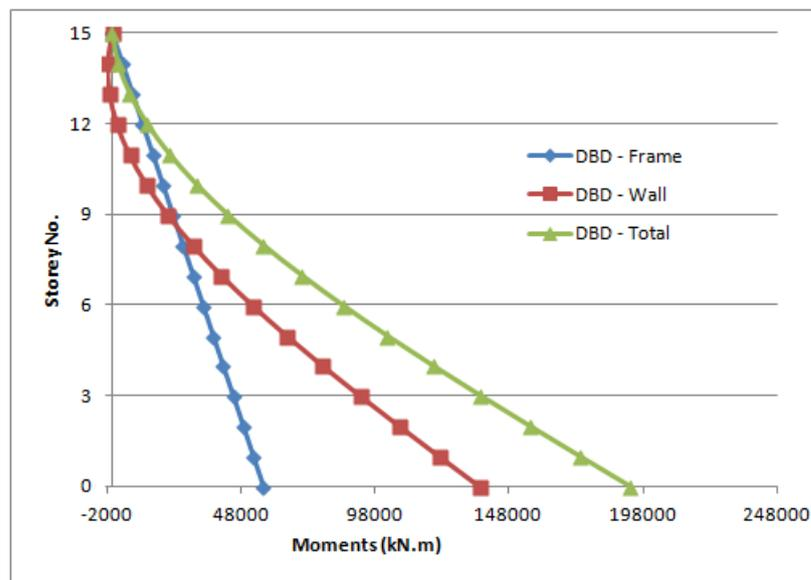
Figure 5.8: Overturning Moment Distribution for DBD - X Direction -  $\beta_F = 0.2$
