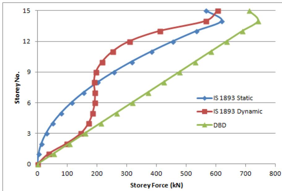
Figure 5.6: Lateral Forces Comparison among FBD and DBD- X Direction -  $\beta_F = 0.2$
