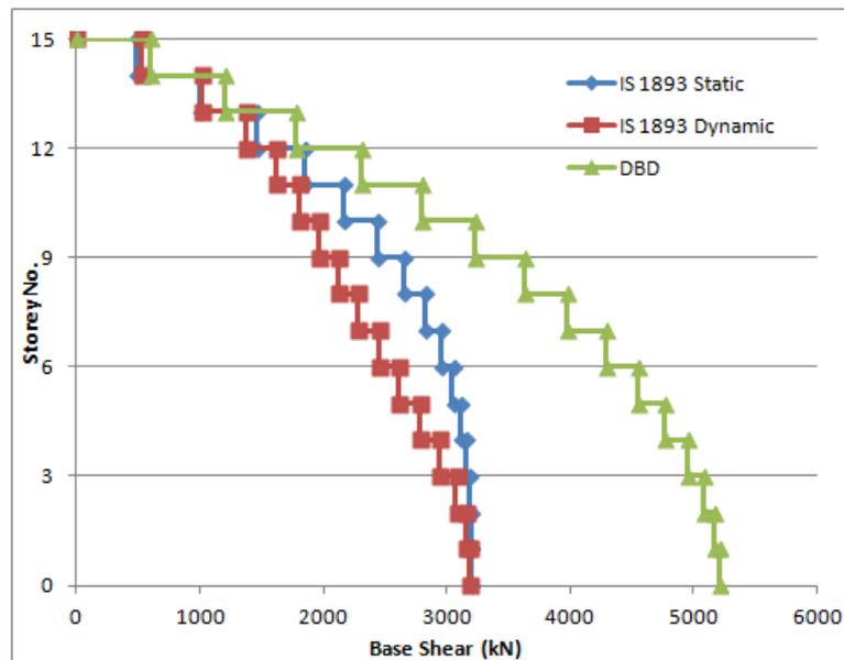
Figure 5.37: Storey Shear Comparison among FBD and DBD - Y Direction -  $\beta_F = 0.4$
