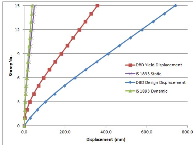
Figure 5.34: Displacement Comparison among FBD and DBD - Y-Direction  $-\beta_F=0.4$
