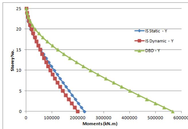
Figure 4.17: Overturning Moment Comparison - X -Direction
