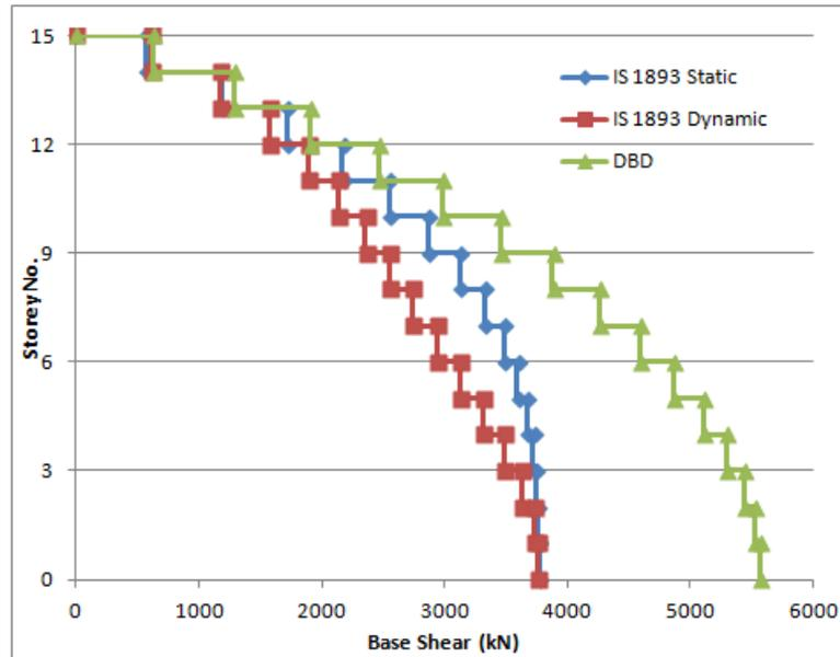
Figure 5.19: Storey Shear Comparison among FBD and DBD - X Direction -  $\beta_F = 0.3$
