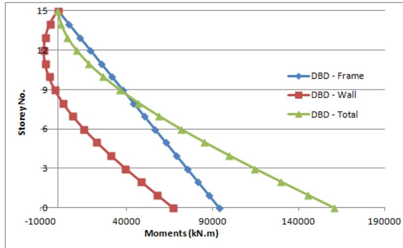
Figure 5.38: Overturning Moment Distribution for DBD - Y Direction -  $\beta_F = 0.4$
