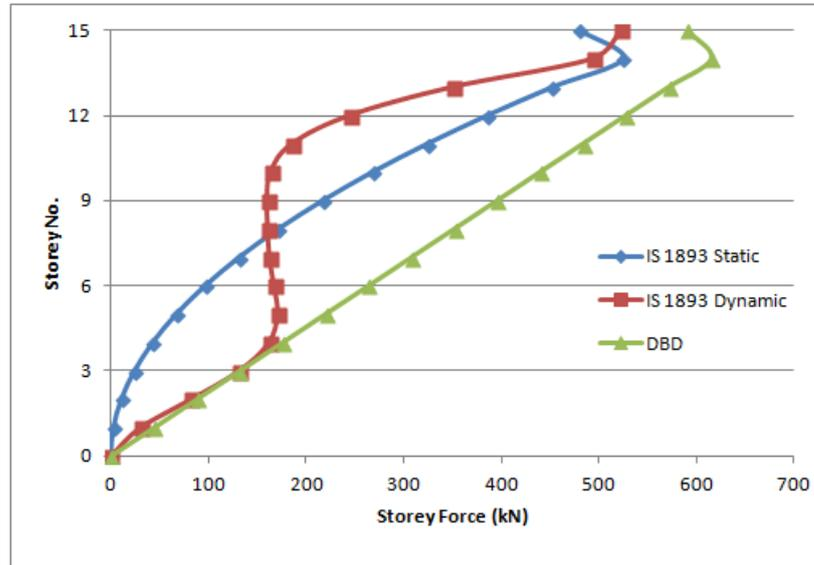
Figure 5.36: Lateral Forces Comparison among FBD and DBD- Y Direction -  $\beta_F = 0.4$
