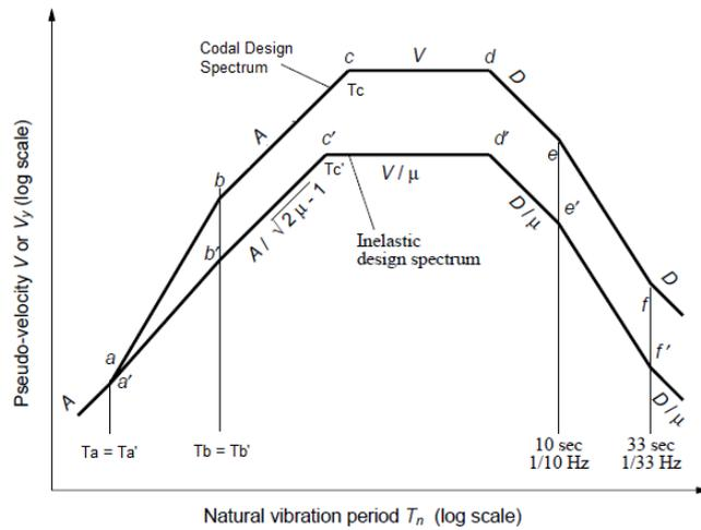
Figure 6.1: Construction of Inelastic Design Spectrum by Newmark-Hall Procedure
