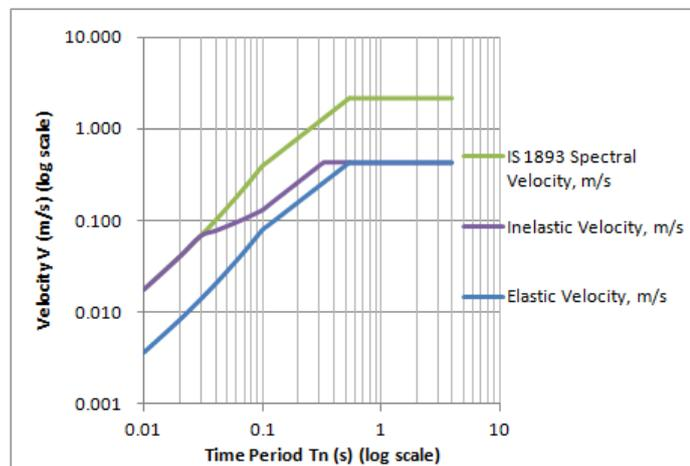
Figure 6.4: Log Velocity  $v/s$  Log Time Period - IS 1893, Elastic and Inelastic
