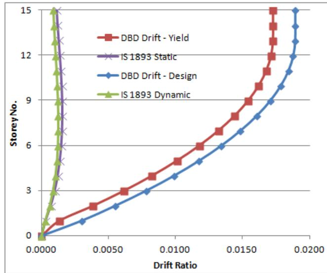
Figure 5.5: Drift Comparison among FBD and DBD - X Direction -  $\beta_F = 0.2$
