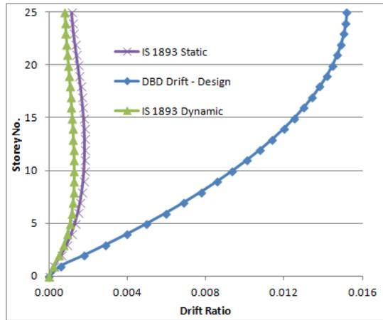
Figure 4.14: Drift Variation by FBD and DBD - X -Direction
