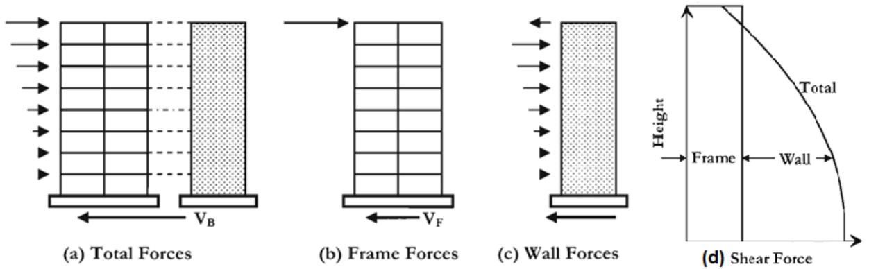
Figure 5.2: Distribution of Base shear force between Wall and Frame
