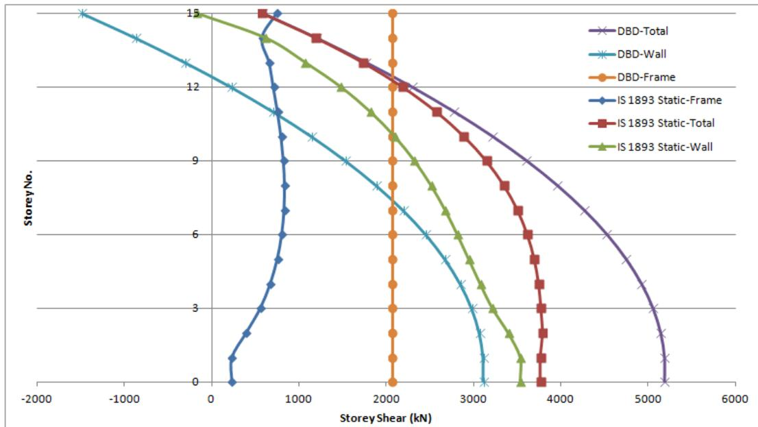
Figure 5.33: Storey Shear Distribution between Frames and Walls by FBD and DBD - X Direction  $-\beta_F = 0.4$
