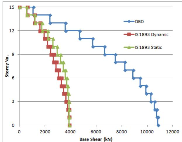
Figure 4.6: Variation of the Storey Shear across the height- X -Direction
