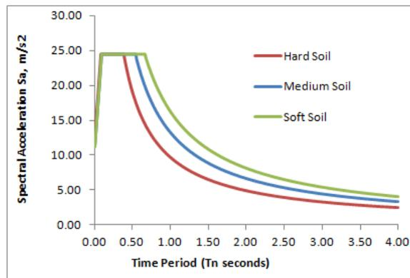
Figure 3.1: IS Design Acceleration Spectrum
