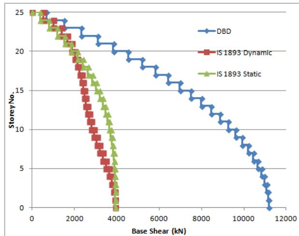
Figure 4.16: Variation of the Storey Shear across the height- X -Direction
