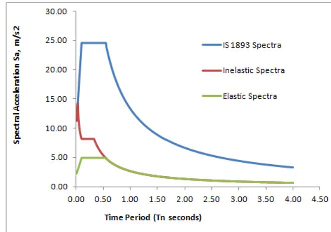
Figure 6.3: Acceleration spectrum - IS 1893, Elastic and Inelastic
