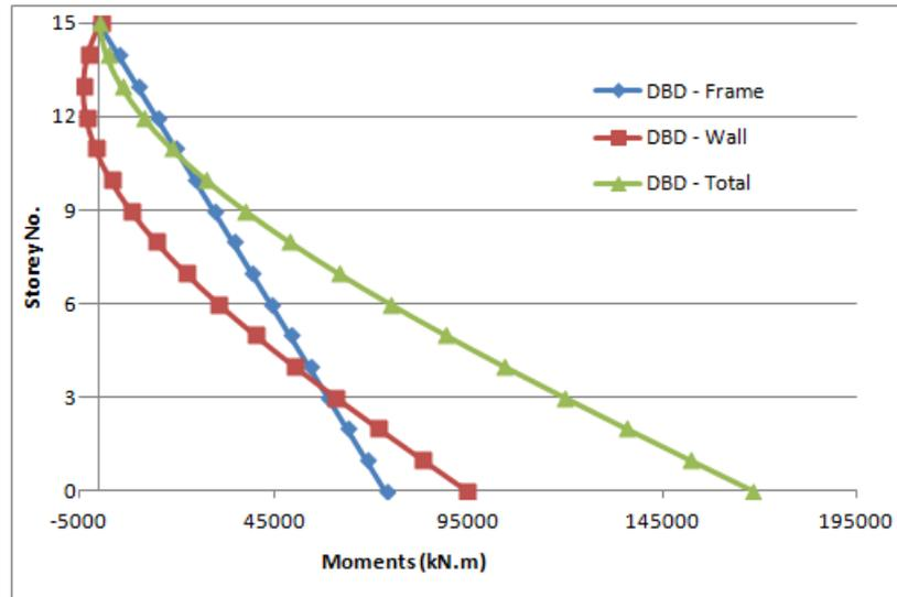
Figure 5.26: Overturning Moment Distribution for DBD - Y Direction -  $\beta_F = 0.3$
