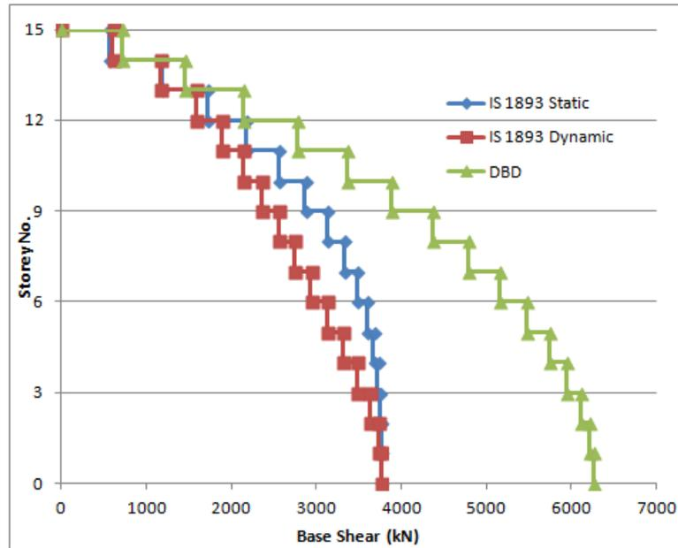
Figure 5.7: Storey Shear Comparison among FBD and DBD - X Direction -  $\beta_F = 0.2$
