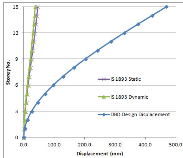
Figure 4.3: Displacement Comparison by FBD and DBD- X -Direction
