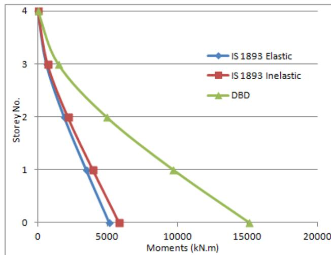
Figure 6.11: Overturning Moment Comparison
