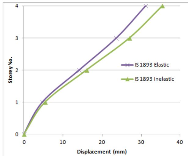
Figure 6.6: Displacement Comparison between FBD - Elastic and Inelastic spectra
