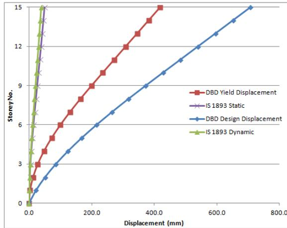
Figure 5.22: Displacement Comparison among FBD and DBD - Y-Direction- $\beta_F=0.3$
