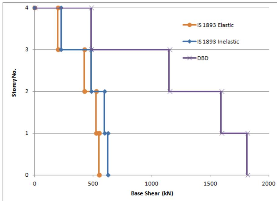
Figure 6.9: Storey Shear
