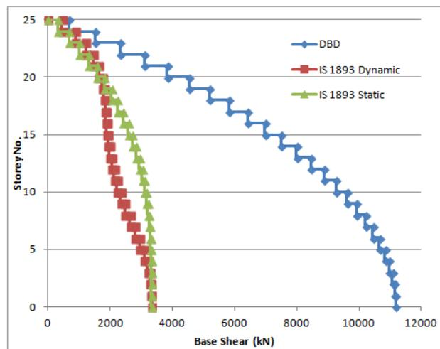
Figure 4.21: Variation of the Storey Shear across the height- Y - Direction
