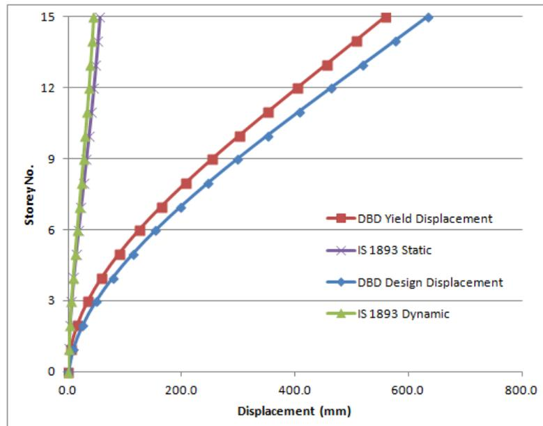
Figure 5.4: Displacement Comparison among FBD and DBD - X Direction -  $\beta_F = 0.2$
