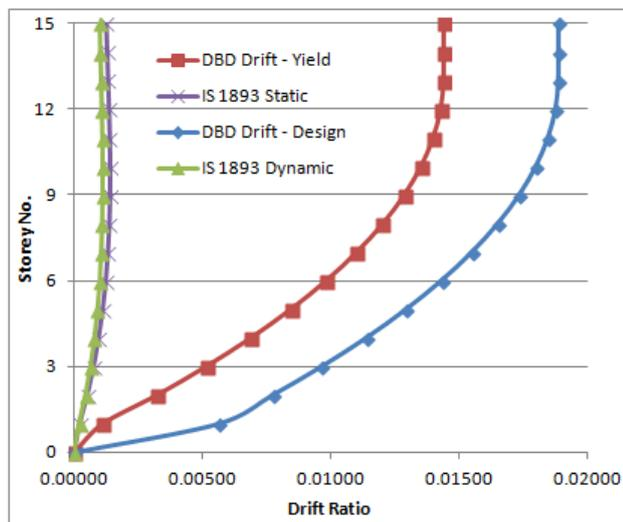
Figure 5.11: Drift Comparison among FBD and DBD - Y Direction - $\beta_F = 0.2$
