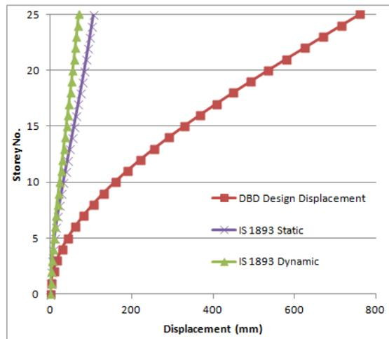
Figure 4.18: Displacement Comparison by FBD and DBD- Y -Direction
