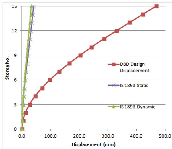
Figure 4.8: Displacement Comparison by FBD and DBD- Y -Direction
