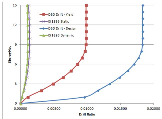
Figure 5.35: Drift Comparison among FBD and DBD - Y Direction  $-\beta_F = 0.4$
