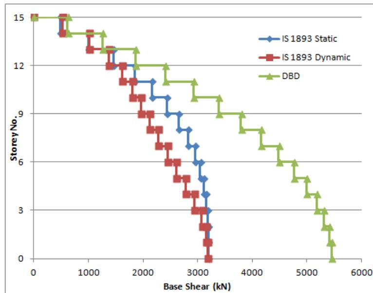
Figure 5.25: Storey Shear Comparison among FBD and DBD - Y Direction -  $\beta_F = 0.3$
