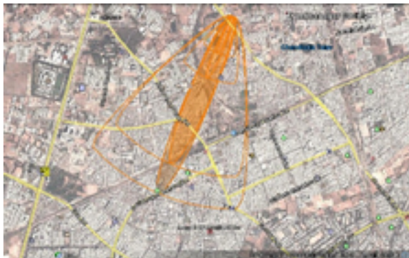
Figure 6: Toxic threat zone for AEGL concentration of 2.0 ppm for all the considered releases of liquefied chlorine gas.
