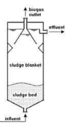
Figure 1: Schematic of UASB reactor
