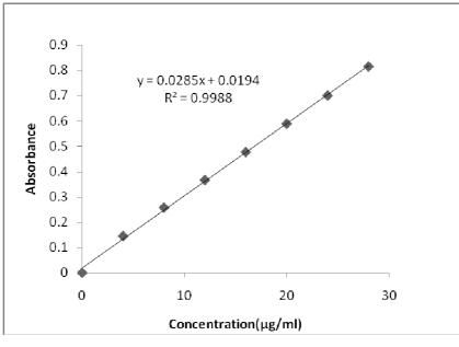
Figure: 4 Calibration Curve of PM (4-28µg/ml) at 206.8 nm
