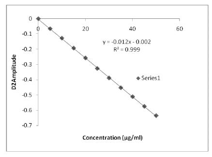
Figure: 3 Calibration Curve of CT (5-50µg/ml) at 274.60 nm
