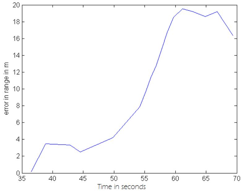
Figure 4.2: Slant range errors for SRP time delays
