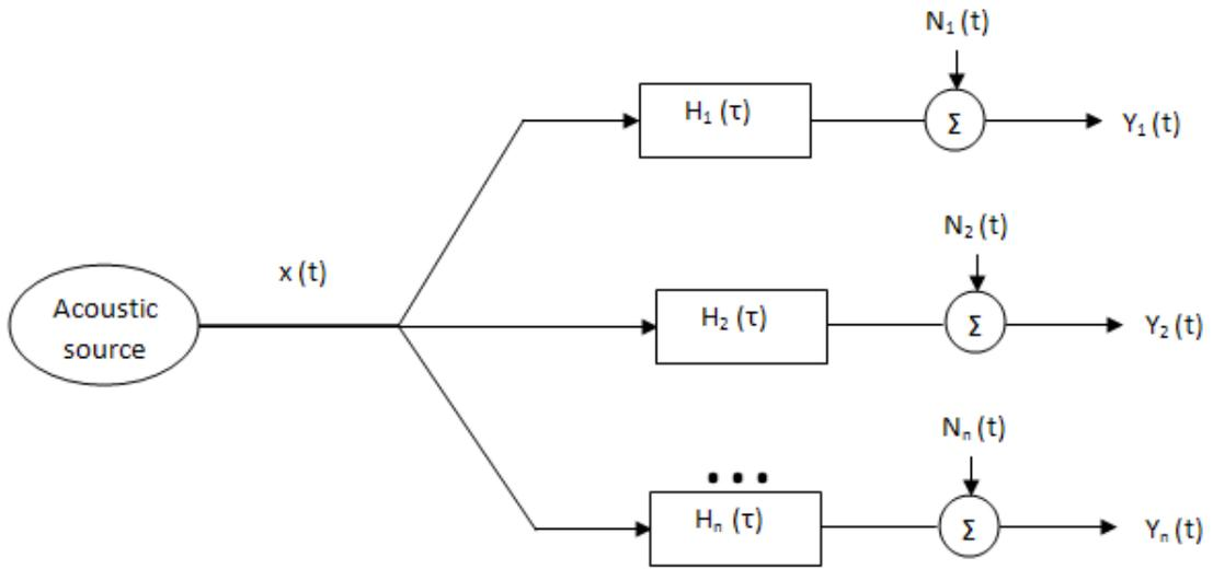
Figure 2.1: Multipath model of communication channel
