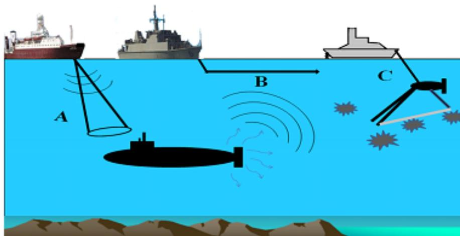
Figure 1.4: Schematic depiction of three types of sonars
