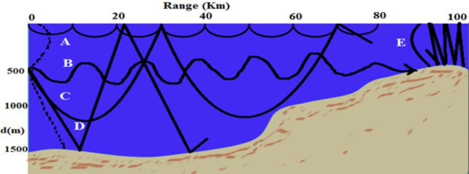
Figure 3.5: Schematic of ray paths in the ocean.
