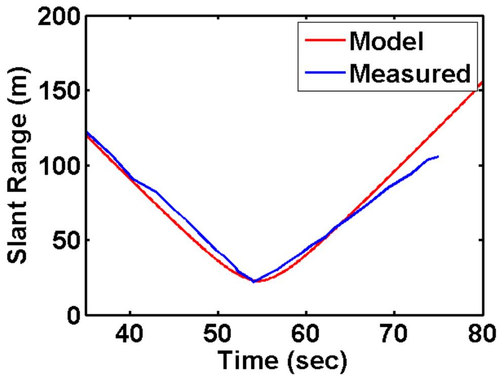
Figure 3.9: Comparison of slant ranges obtained from modelled and estimated time delays
