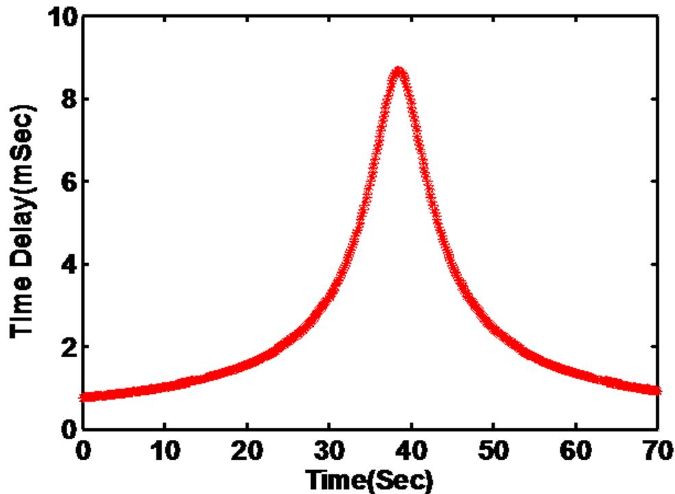
Figure 3.7: Time delay estimates from bellhop ray model
