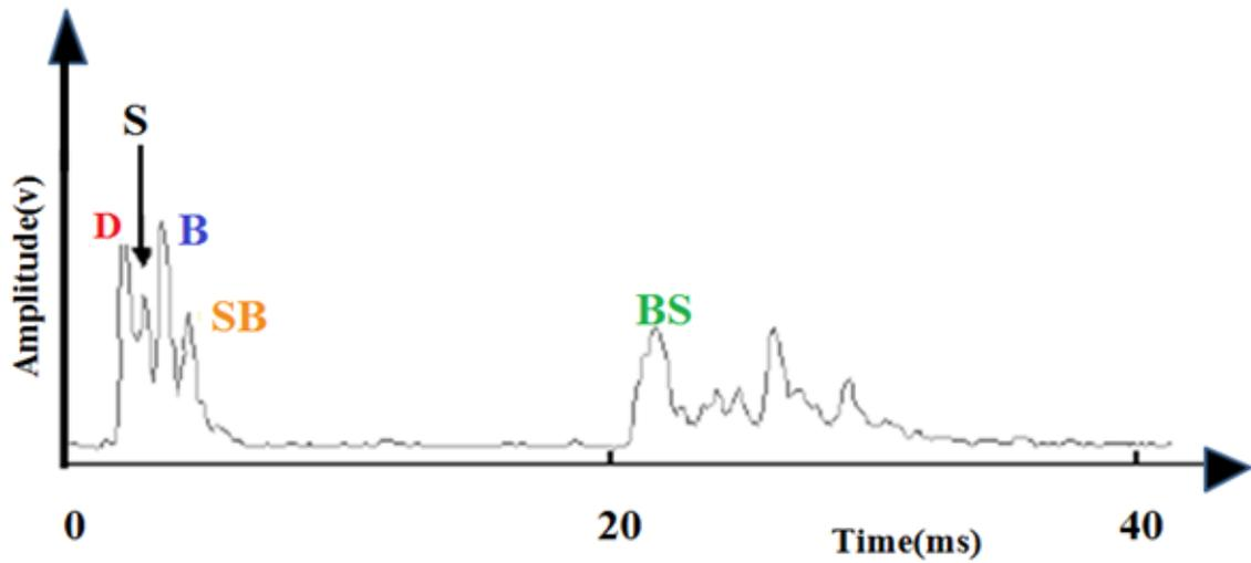
Figure 2.3: Received time series due to multipath effect
