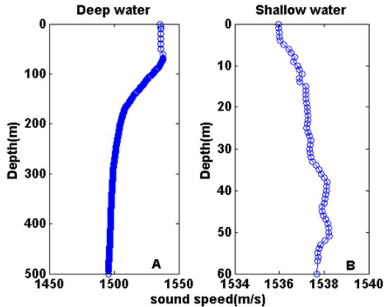
Figure 1.3: Sound speed profiles for deep and shallow water environments off vizag coast
