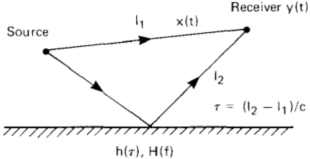
Figure 2.6: signal with improper reflection
