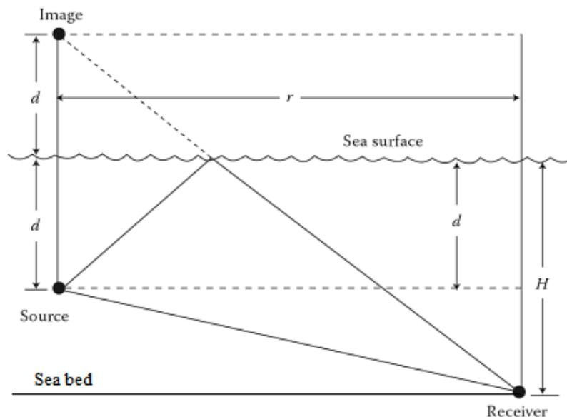
Figure 2.4: Geometry of image interference
