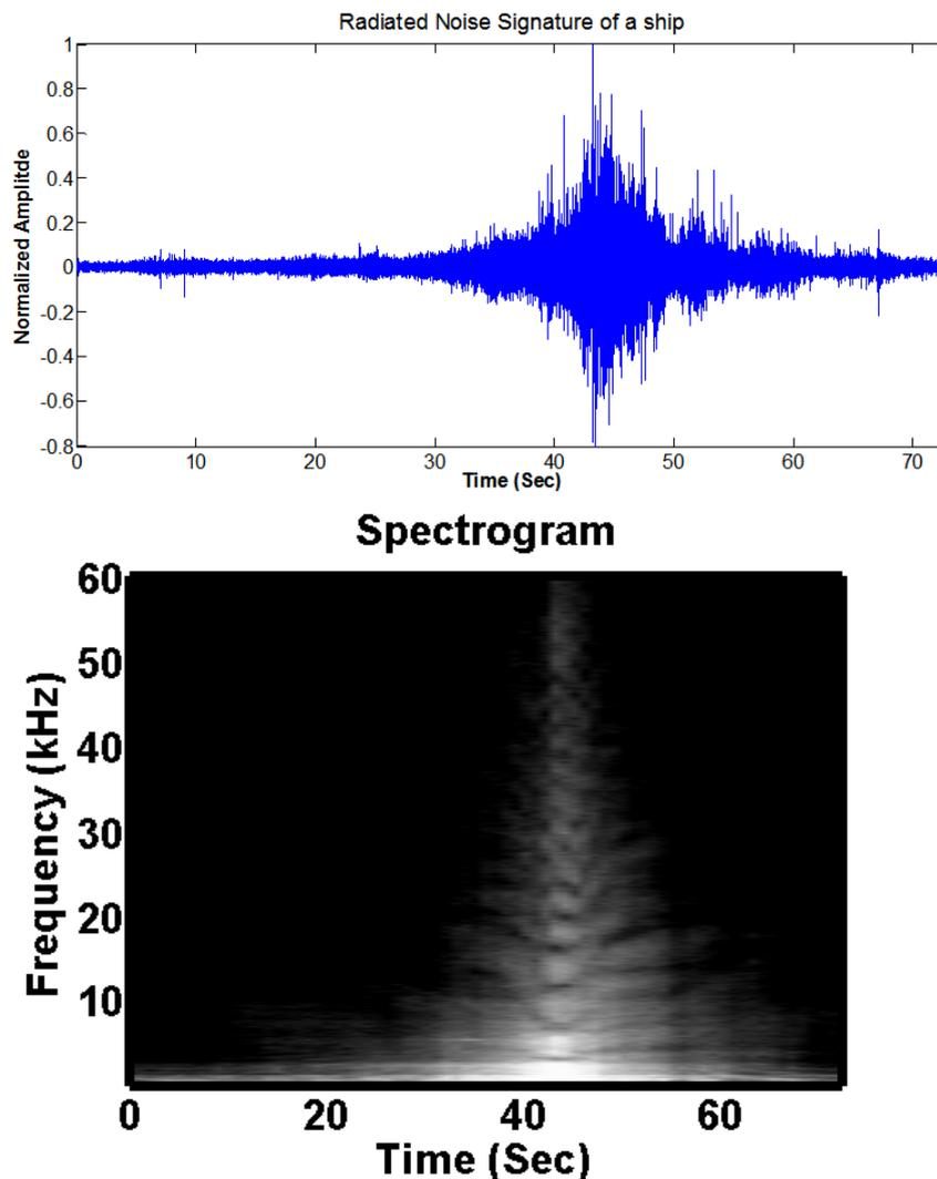
Figure 3.2: Power spectrum showing lloyd mirror pattern
