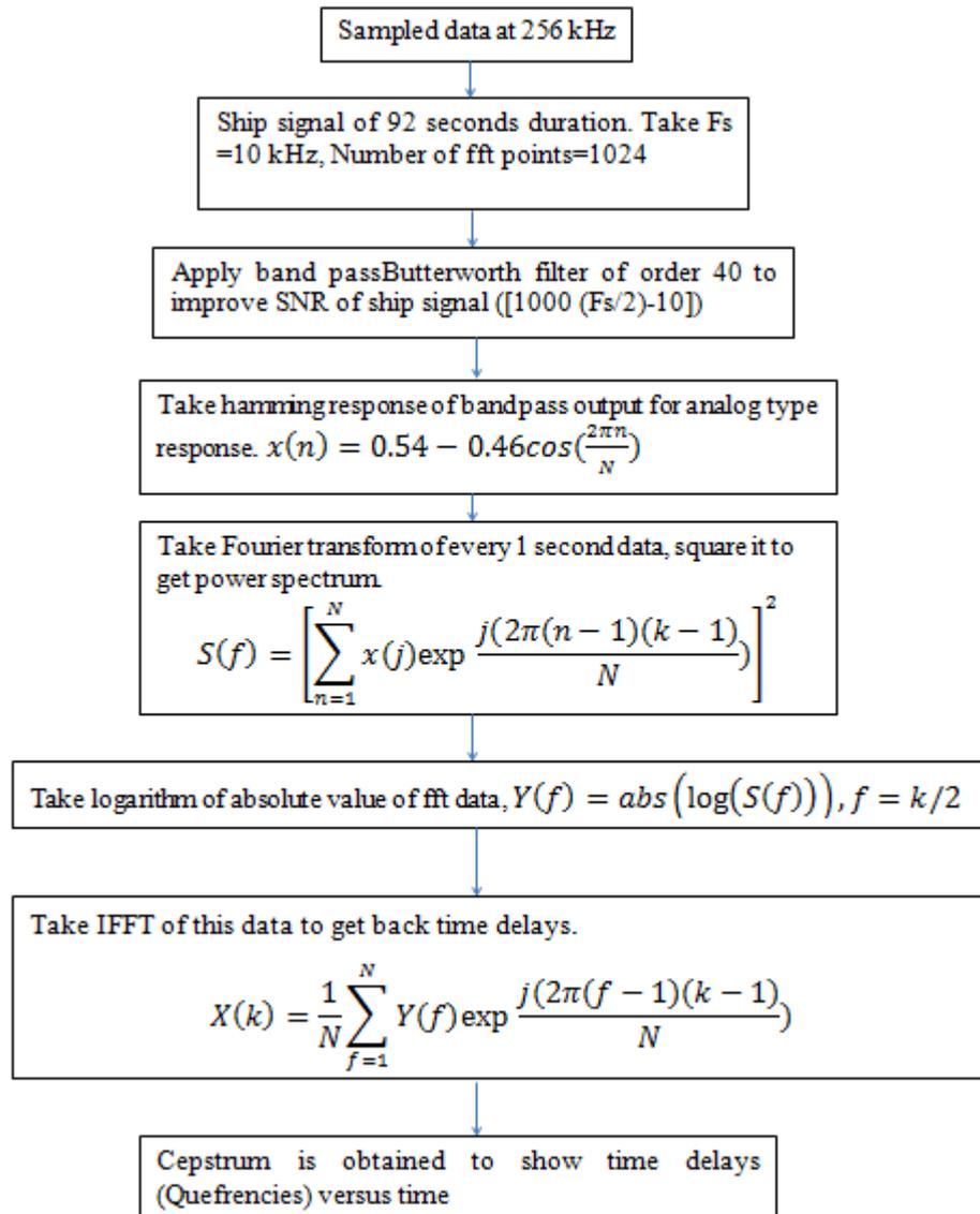
Figure 3.3: Block diagram showing TDE from power cepstrum
