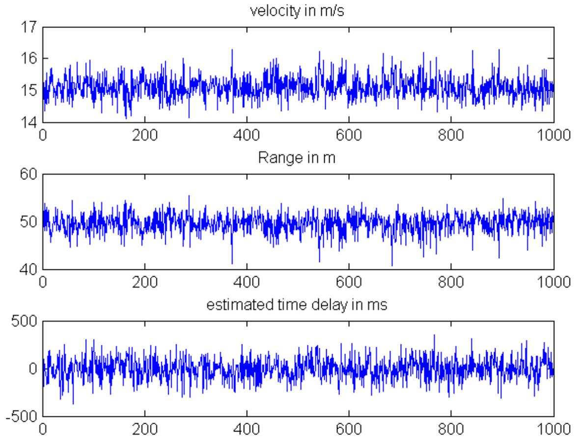
Figure 4.4: Simulation results with 50 us standard deviation
