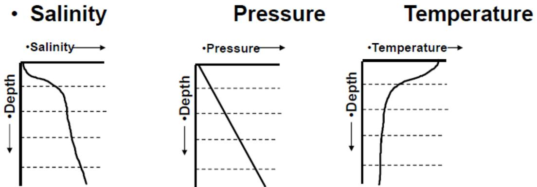
Figure 1.2: Effect of salinity, temperature and pressure on sound speed profile with respect to depth
