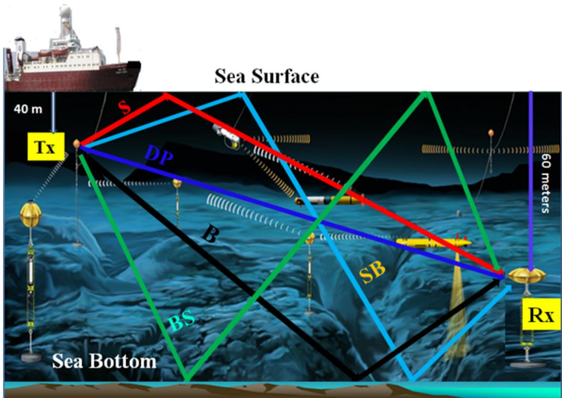
Figure 2.2: Multipath model of the underwater communication channel
