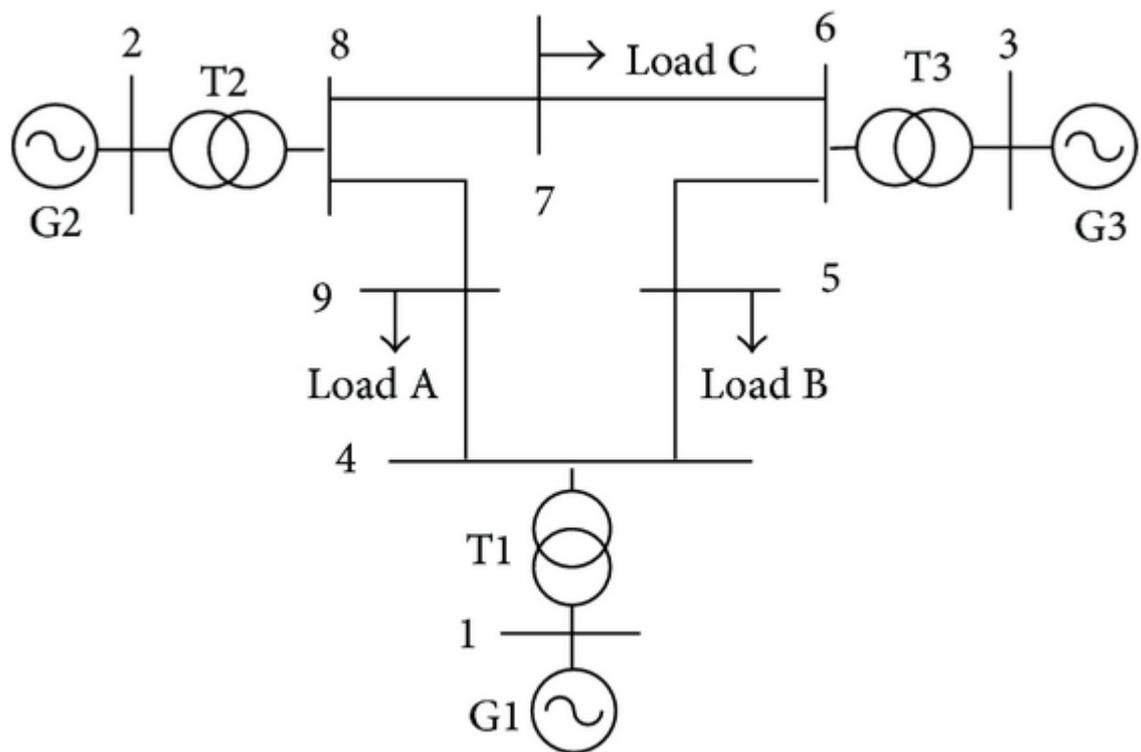
Figure A.1: WSCC 3-generators 9-bus system
