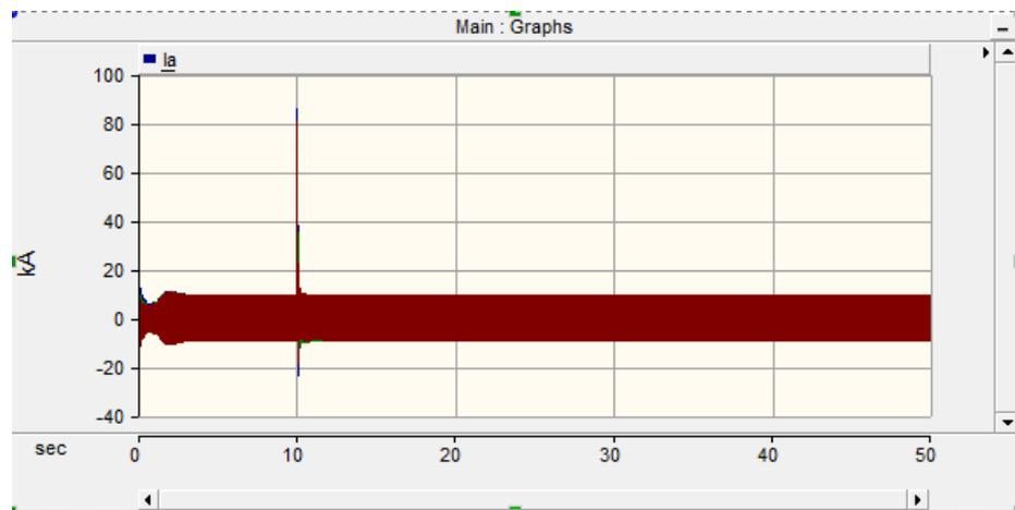
Figure 5.12: Three phase to ground fault(LLL-G) at bus-2
