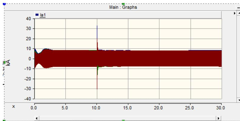
Figure 4.10: Phase to ground fault(L-G) at bus-2
