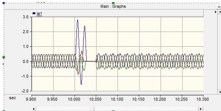
Figure 4.16: Phase to ground fault(L-G) at load-1
