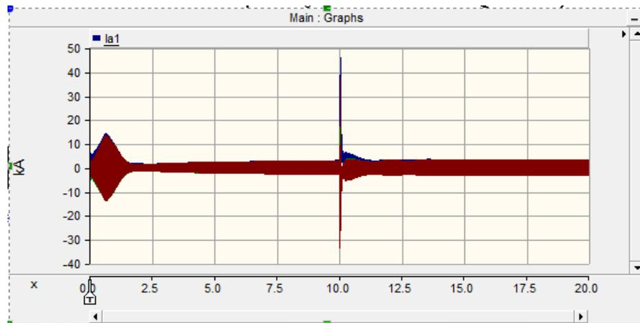
Figure 4.12: Phase to ground fault(L-G) at bus-1
