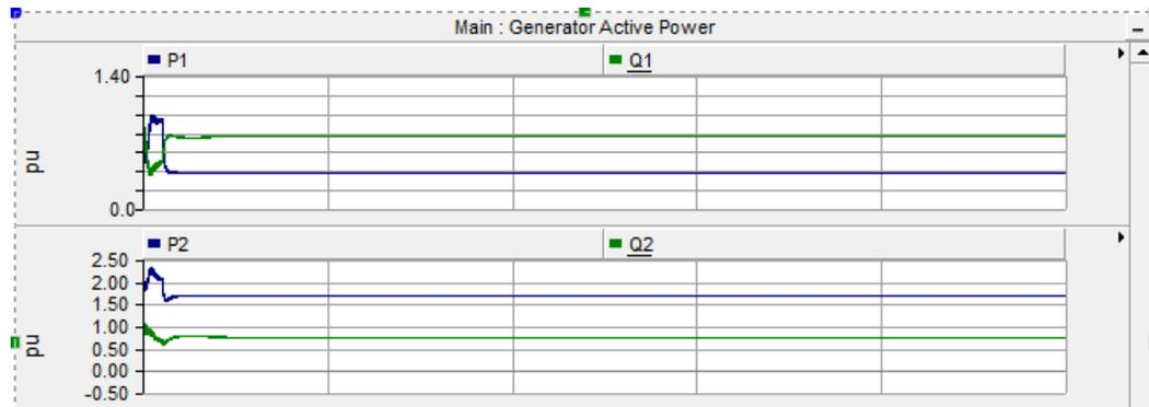
Figure 5.2: Active and Reactive Power of wind generator
