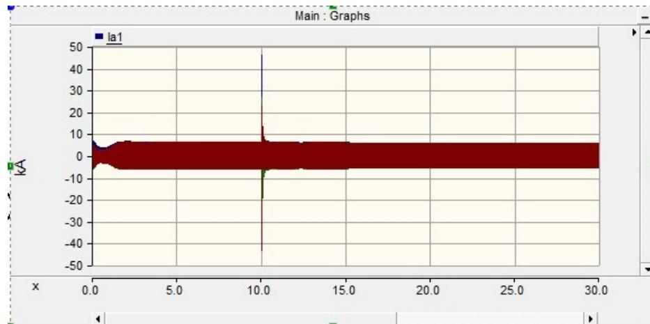
Figure 4.8: Phase to ground fault(L-G) at bus-3
