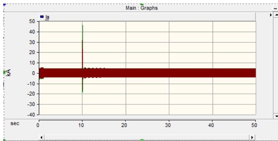
Figure 5.13: Phase to ground fault(L-G) at bus-1
