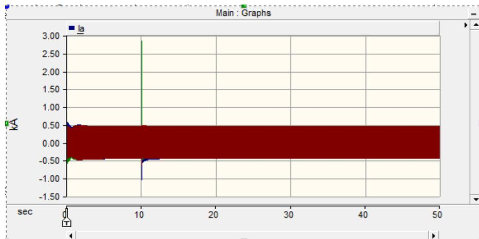
Figure 5.17: Phase to ground fault(L-G) at load-1
