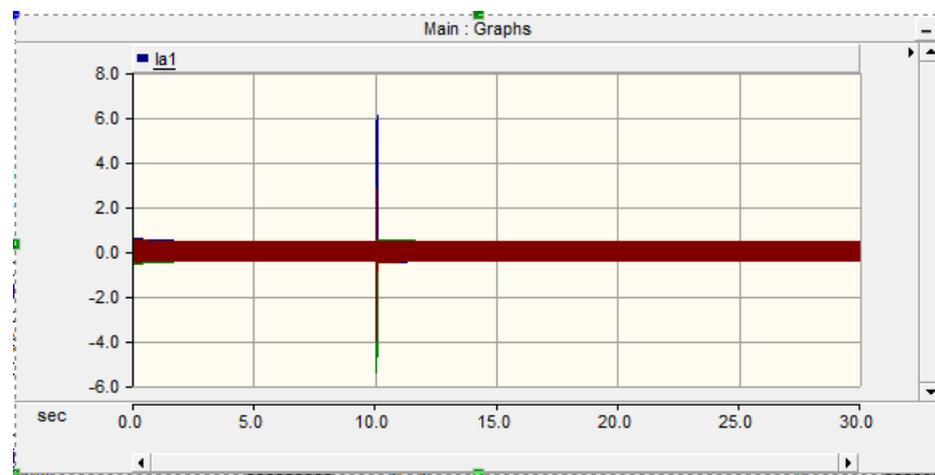
Figure 4.17: Three phase to ground fault(LLL-G) at load-1
