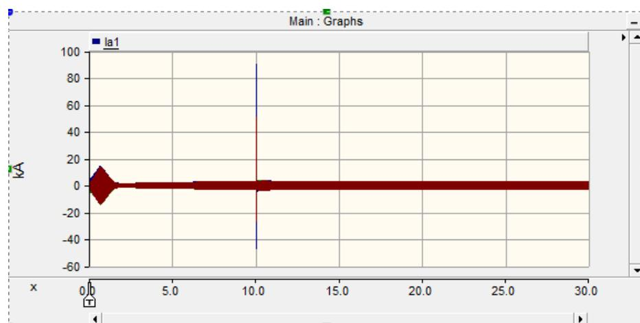
Figure 4.13: Three phase to ground fault(LLL-G) at bus-1
