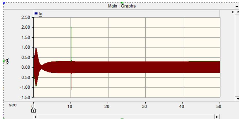
Figure 5.15: Phase to ground fault(L-G) at bus-4
