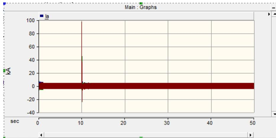
Figure 5.14: Three phase to ground fault(LLL-G) at bus-1
