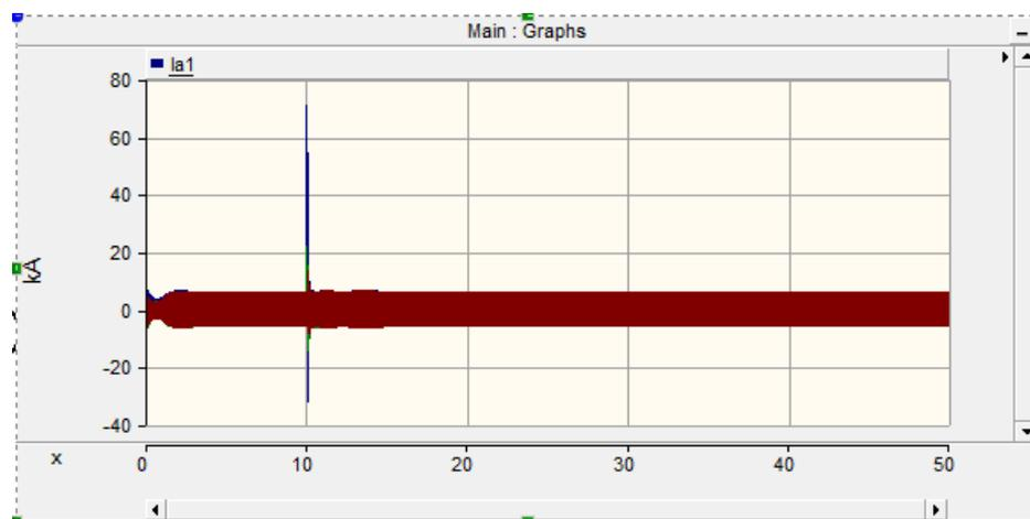
Figure 4.9: Three phase to ground fault(LLL-G) at bus-3
