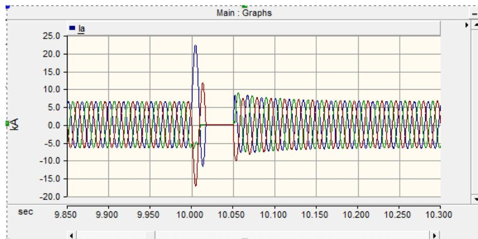
Figure 5.9: Zoomed view of phase to ground fault(L-G) at bus-3
