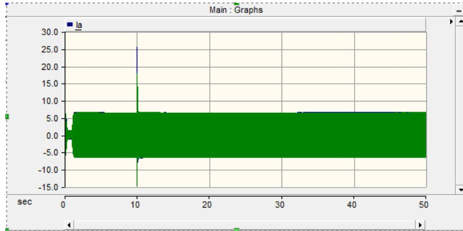
Figure 5.10: Three phase to ground fault(LLL-G) at bus-3
