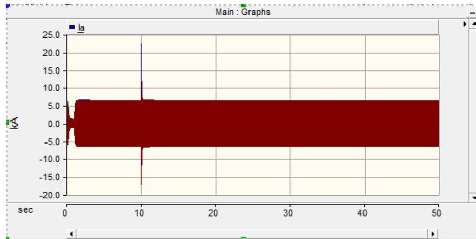
Figure 5.8: Phase to ground fault(L-G) at bus-3
