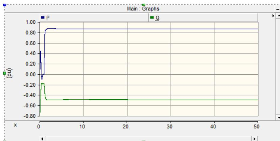
Figure 5.3: Active and Reactive Power of generator 1 and 2
