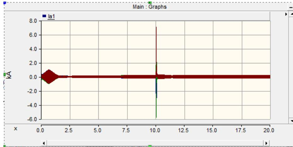
Figure 4.15: Three phase to ground fault (LLL-G) at bus-4
