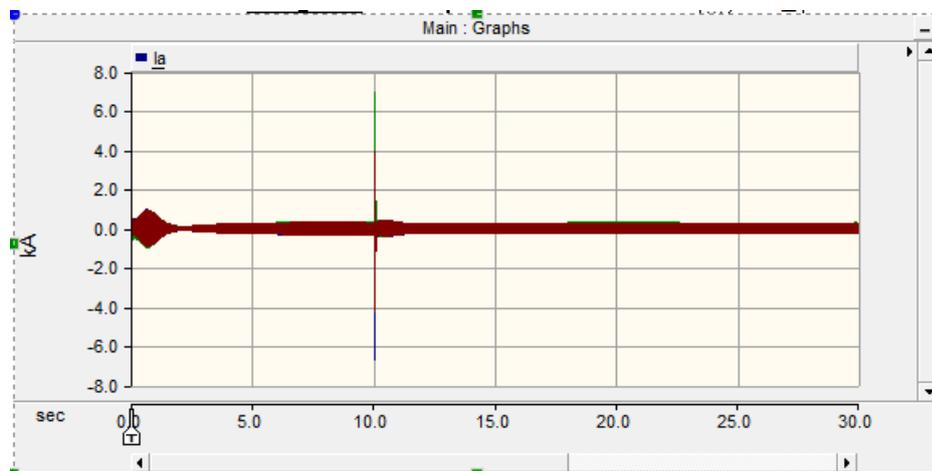
Figure 5.16: Three phase to ground fault(LLL-G) at bus-4
