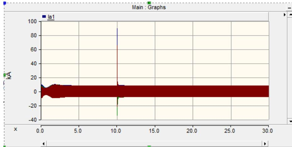
Figure 4.11: Three phase to ground fault(LL-L-G) at bus-2
