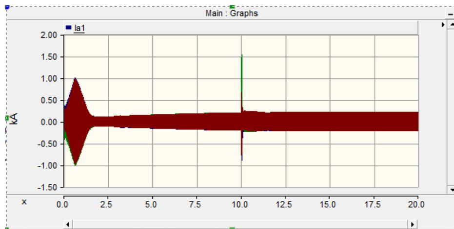
Figure 4.14: Phase to ground fault(L-G) at bus-4
