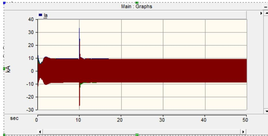
Figure 5.11: Three phase to ground fault(L-G) at bus-2
