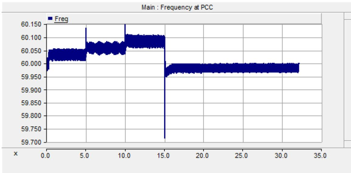
Figure 4.20: Frequency ( $Hz$ ) at PCC for changing load
