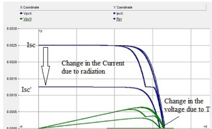
Figure 2.1: Effect of temperature and radiation on solar PV characteristics
