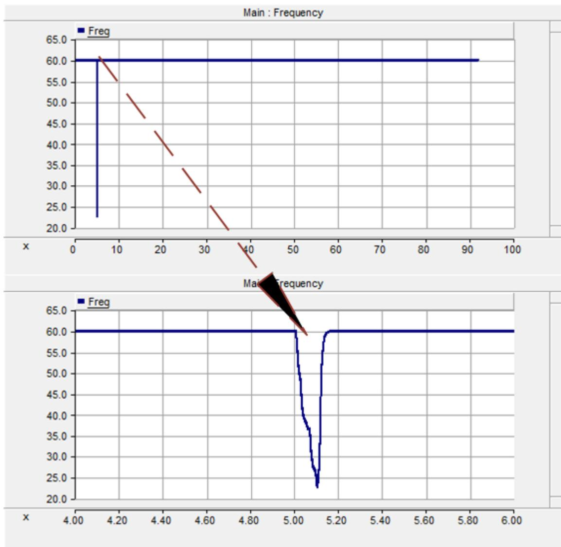
Figure 4.22: Frequency at PCC without solar PV SLG fault
