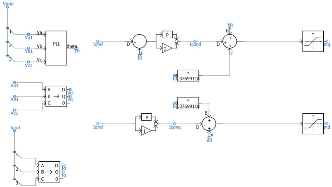
Figure 3.8: Generation of modulated signal after inclusion of voltage drop across filter impedance
