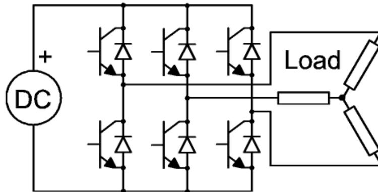
Figure 3.4: Layout of  $3\phi$  inverter
