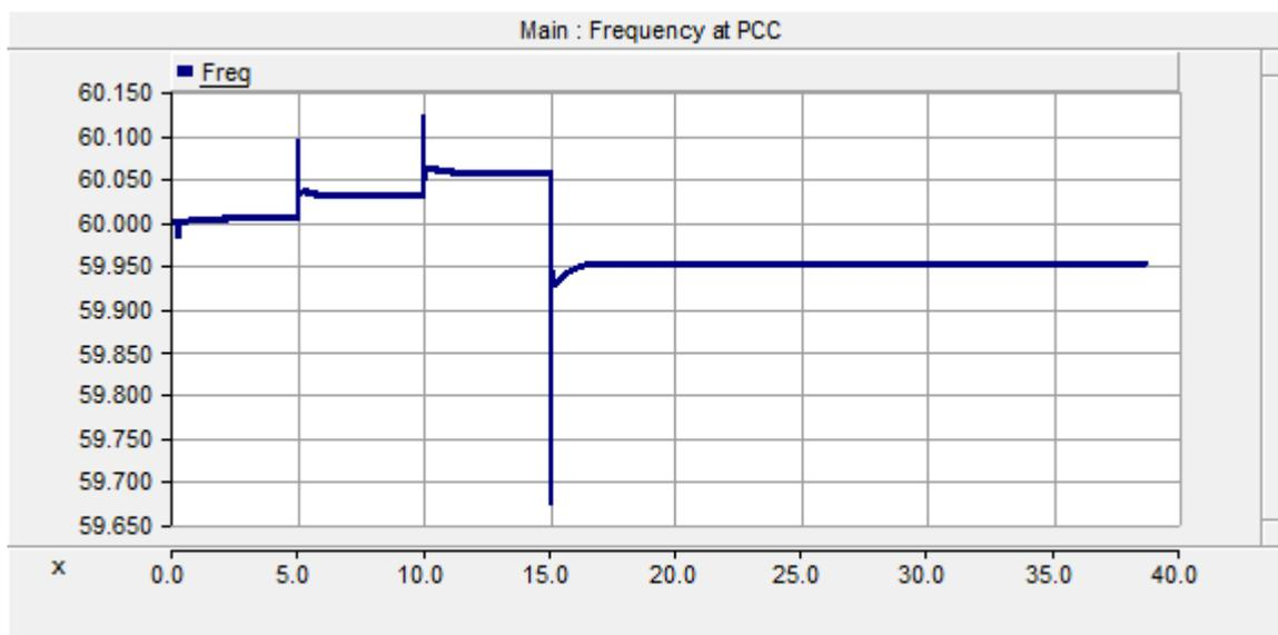
Figure 4.16: Frequency at PCC when load is variable
