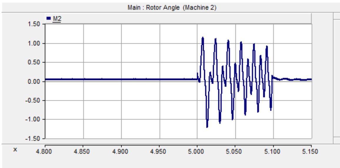
Figure 4.28: Rotor angle of machine 2 at SLG fault with solar PV
