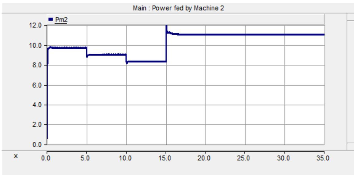
Figure 4.13: Power generated by machine 2
