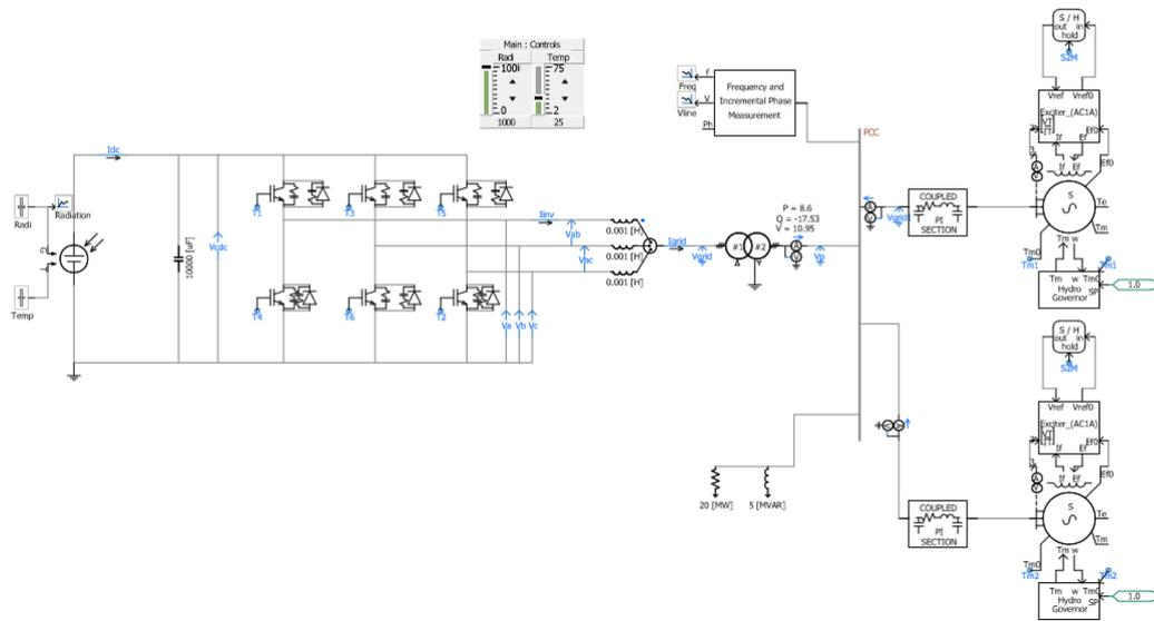
Figure 1: PSCAD model of system under study
