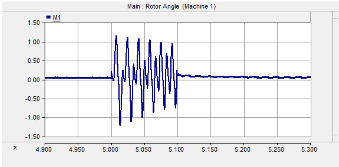
Figure 4.27: Rotor angle machine 1 at SLG fault with solar PV
