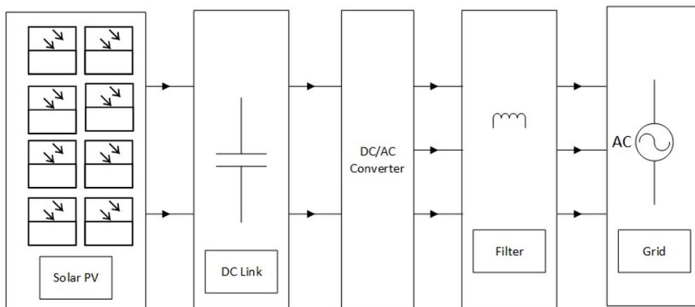
Figure 3.3: Layout of the grid connected solar PV
