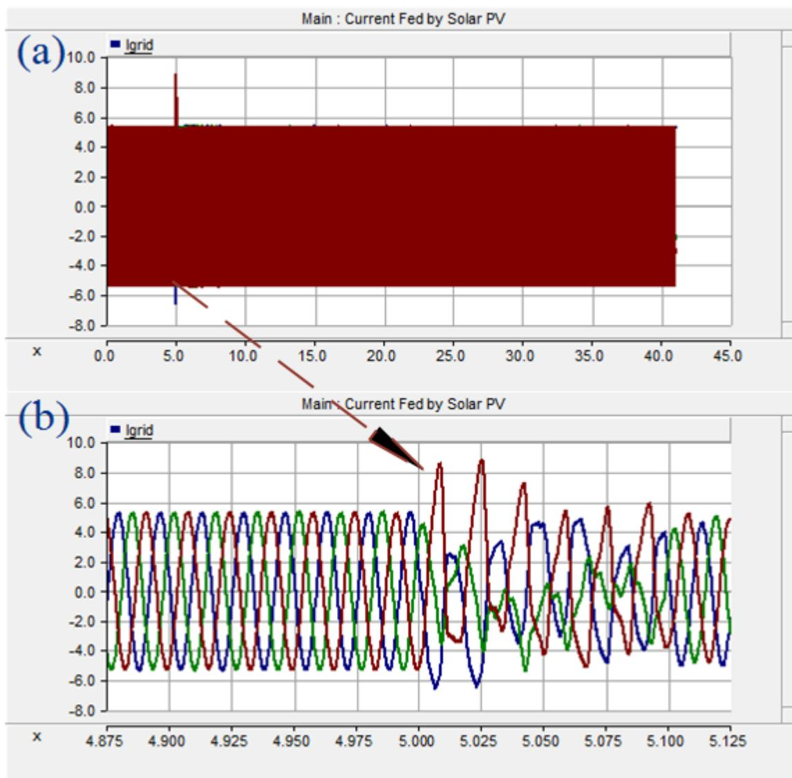
Figure 4.25: Current fed by solar PV at SLG fault
