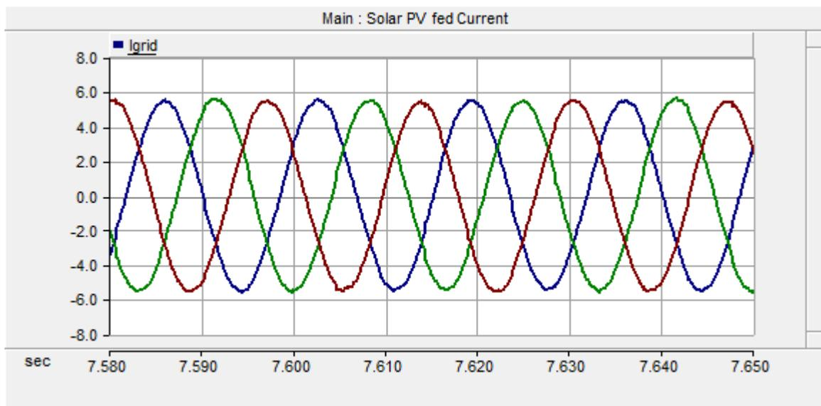
Figure 3.15: Output current of inverter
