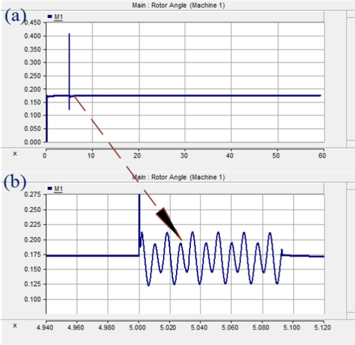
Figure 4.23: Rotor angle oscillations of machine 1 at SLG fault
