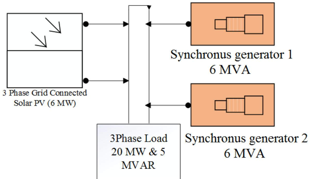
Figure 4.1: Layout of Test System
