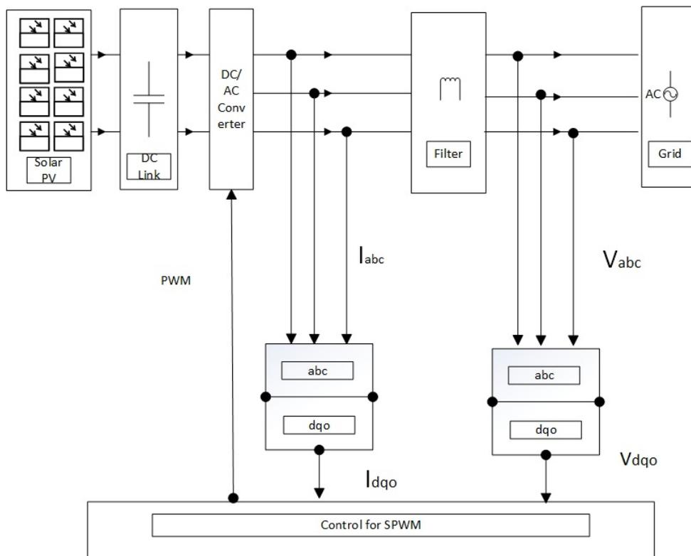
Figure 3.5: Control structure for generating PWM pulses for CR-VSI
