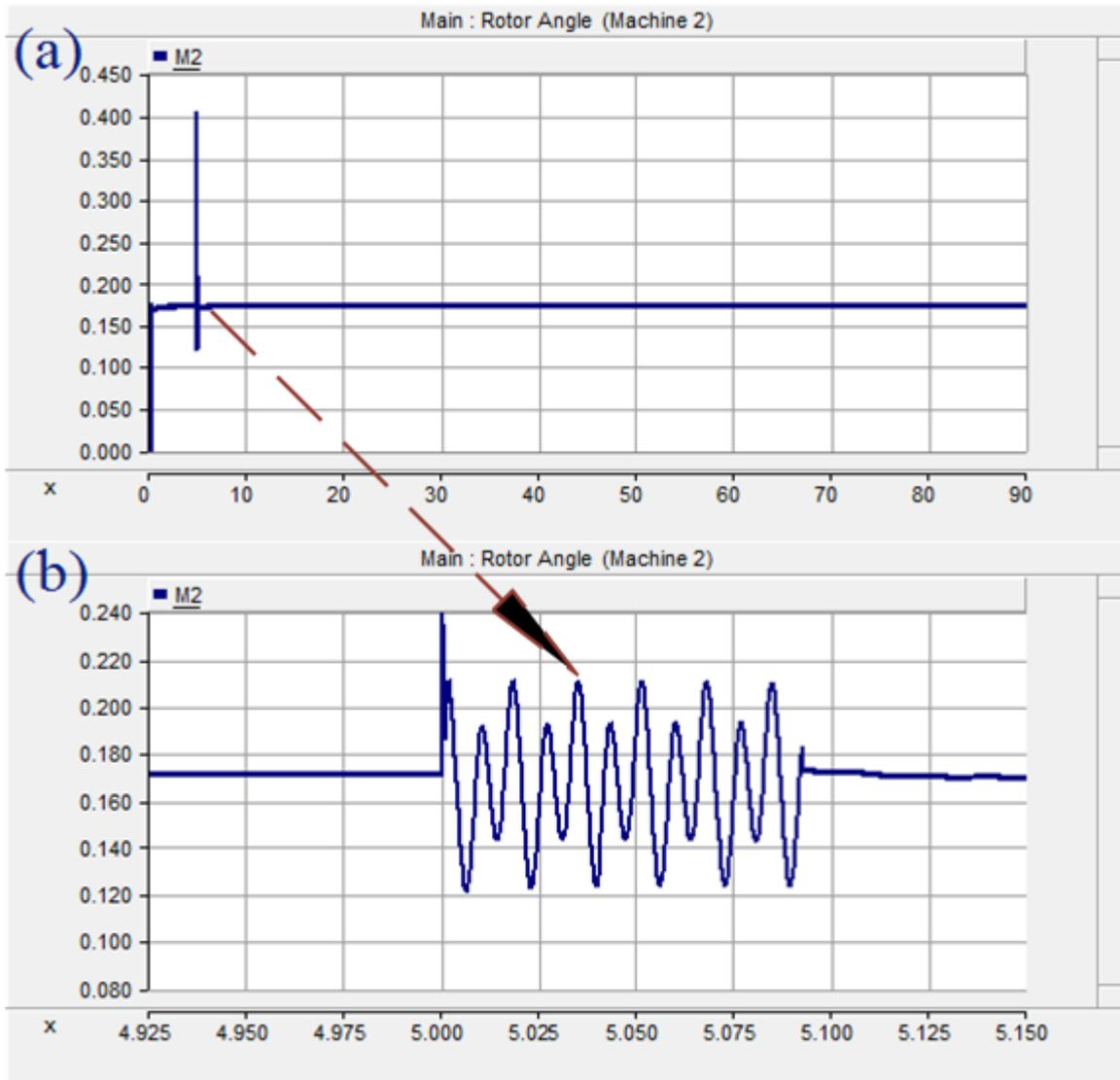
Figure 4.24: Rotor angle oscillations of machine 2 at SLG fault
