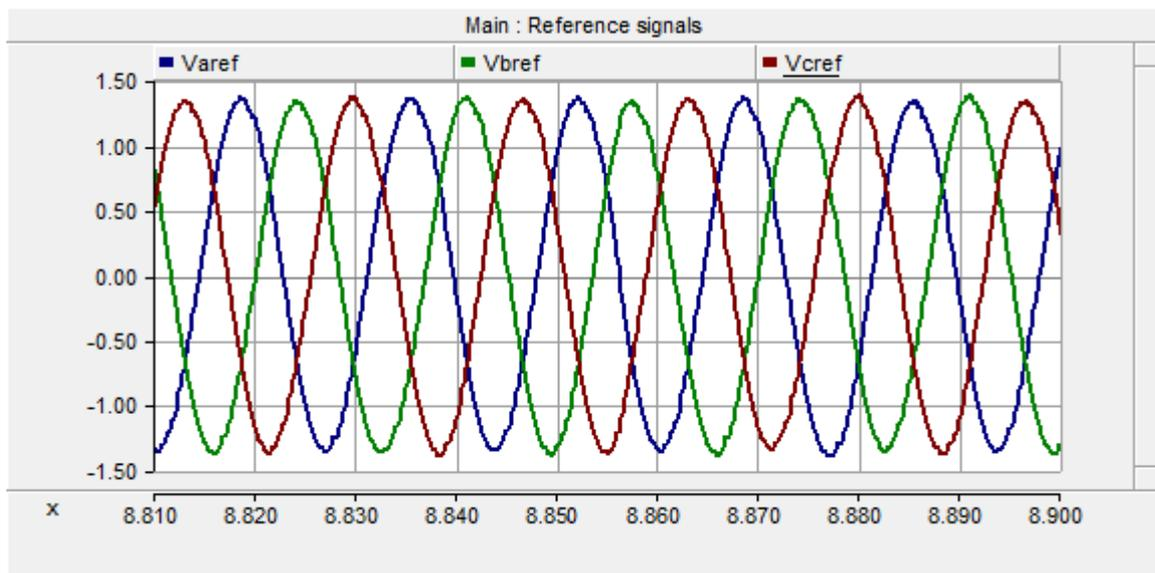
Figure 3.12: Modulated reference signal  $V_{aref}$  of phase  $a$
