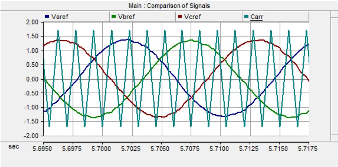
Figure 3.13: Comparison of reference wave and triangular wave
