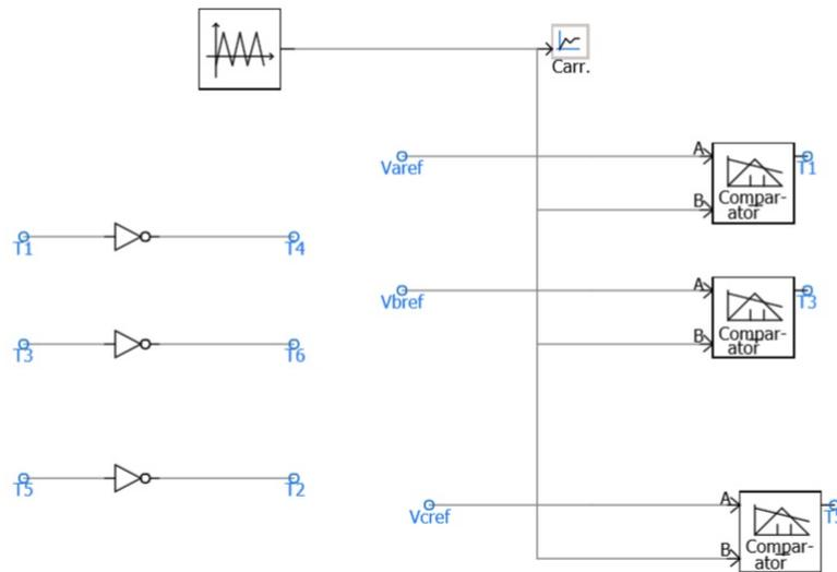
Figure 3.9: Switching signals for inverter IGBT's
