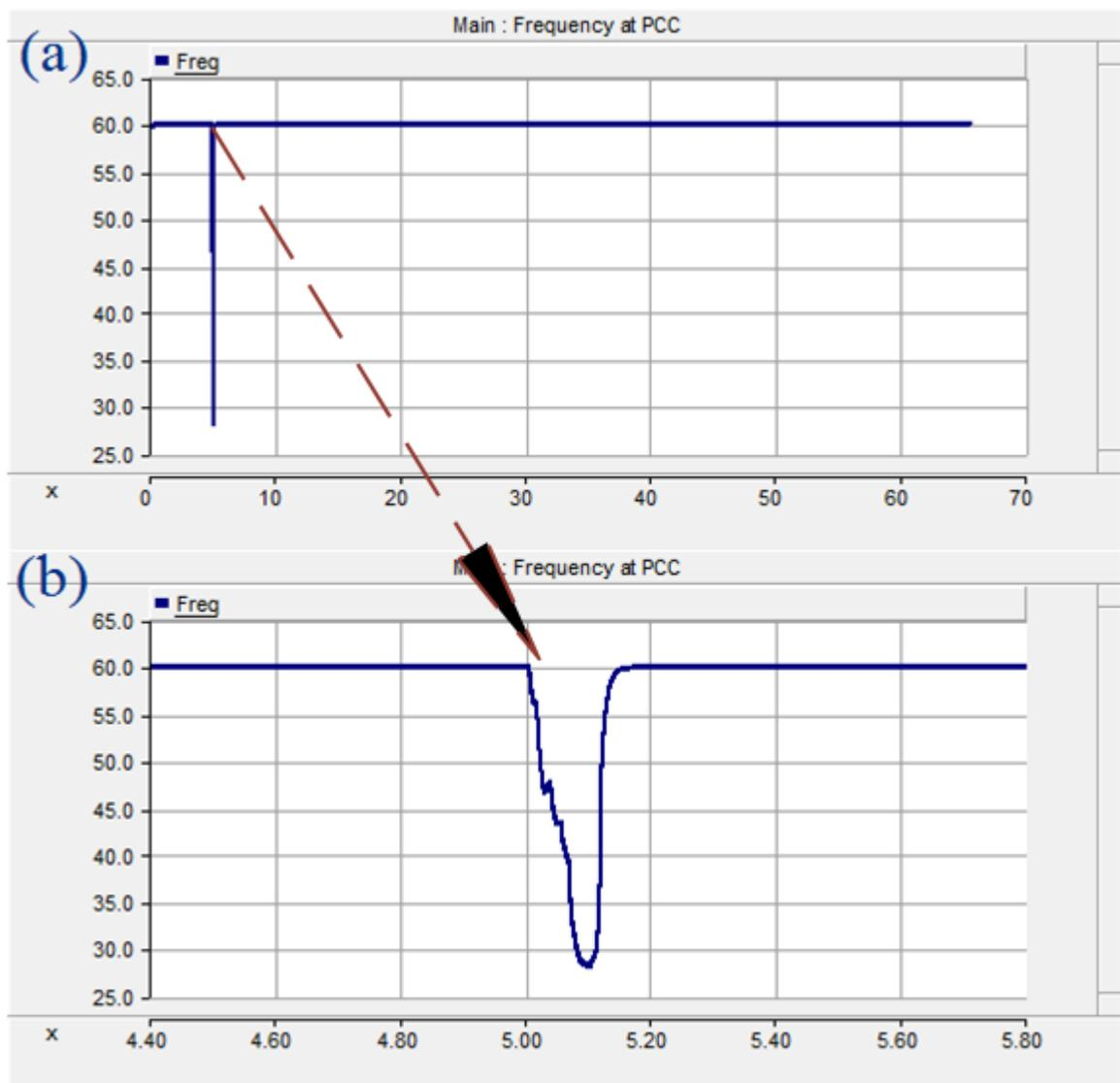
Figure 4.26: Frequency at PCC with solar PV at SLG fault
