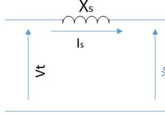
Figure 3.6: Voltage drop occurring at filter impedance
