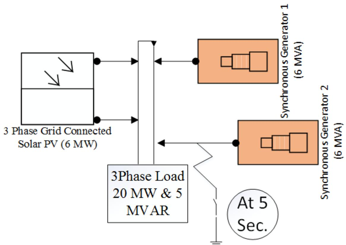
Figure 4.21: Layout of the system for SLG fault study
