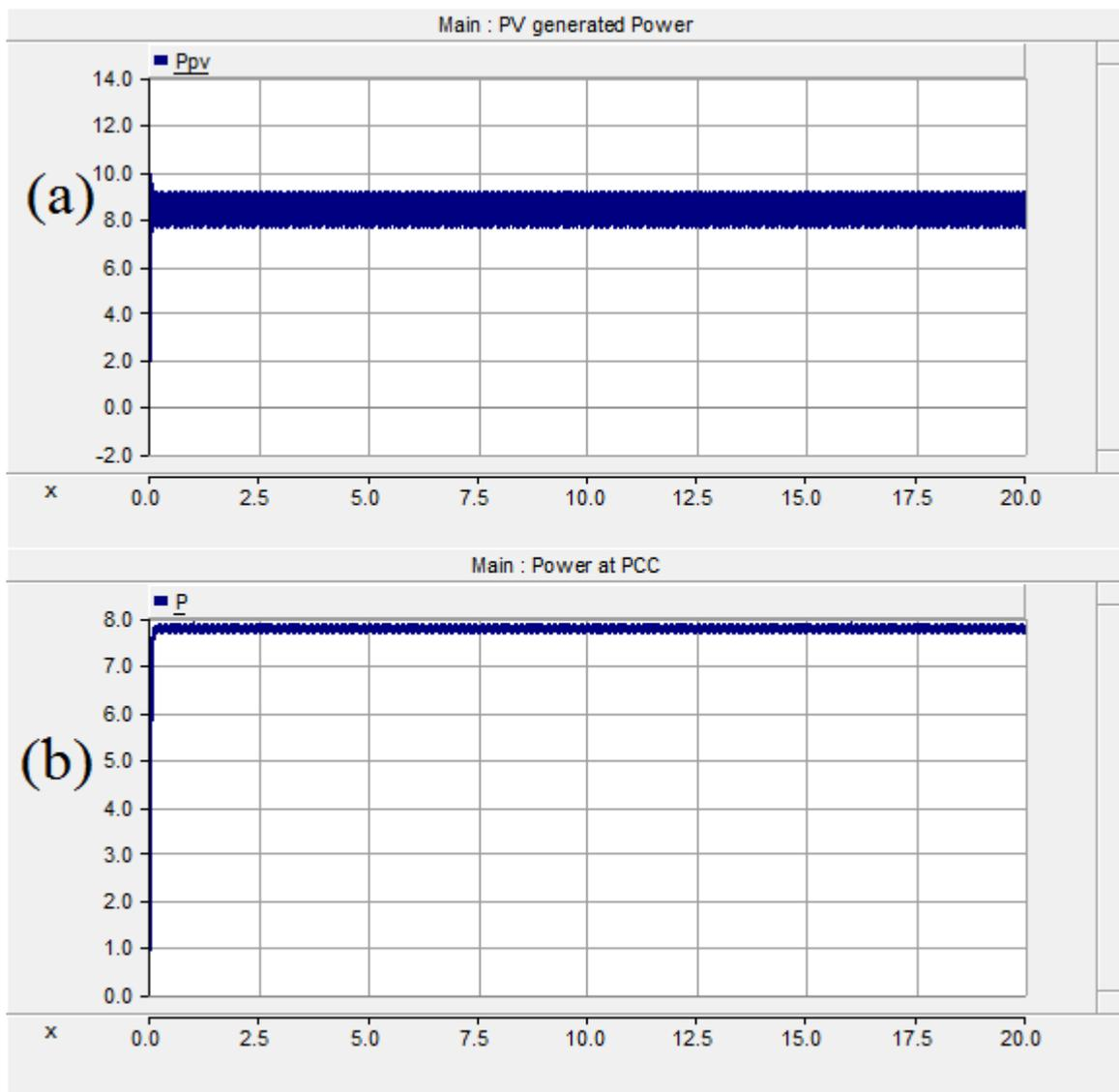
Figure 3.16: (a) Power generated by solar PV (b) Power available at PCC
