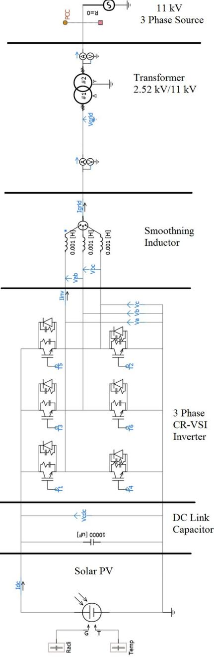
Figure 3.10: 3 phase grid connected solar PV
