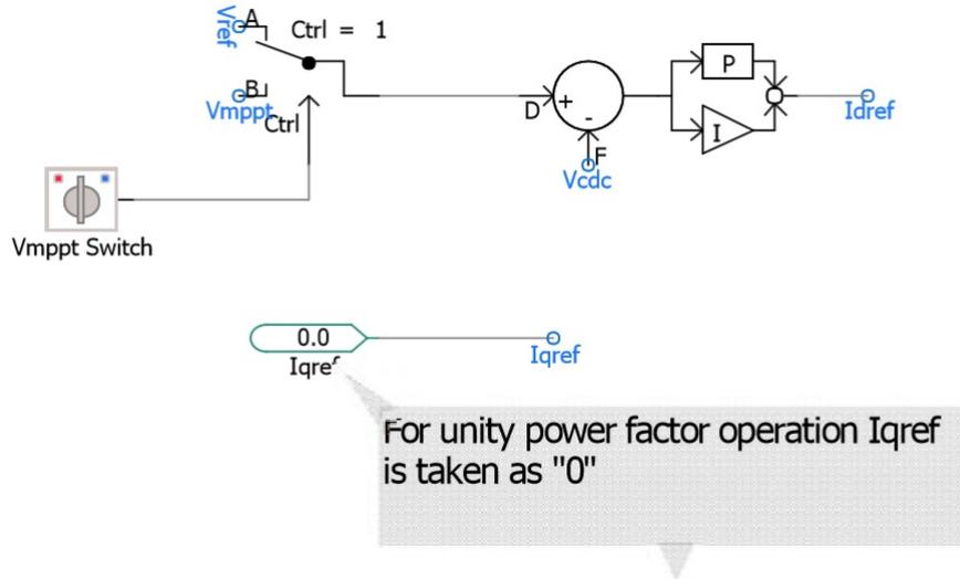
Figure 3.7:  $I_{dref}$  &  $I_{qref}$  for controlling the real and reactive power
