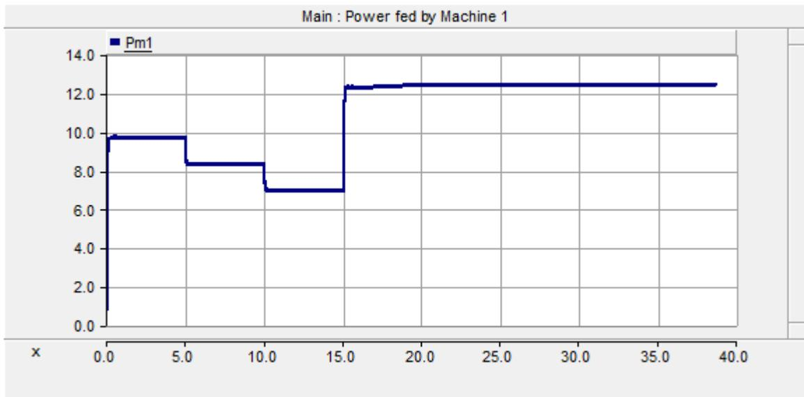
Figure 4.12: Power generated by machine 1
