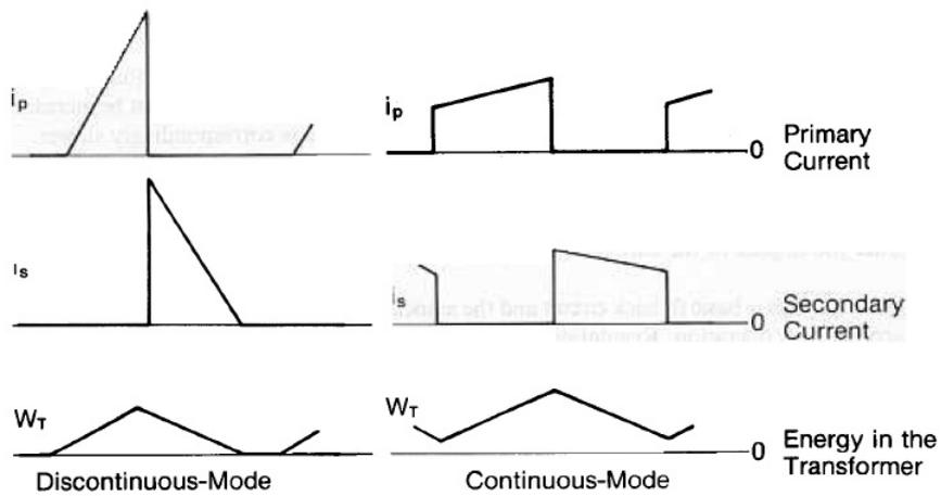
Figure 3.10: Comparison between CCM and DCM
