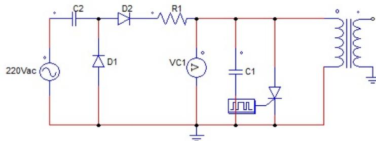
Figure 2.4: Supply circuit using conventional power supply
