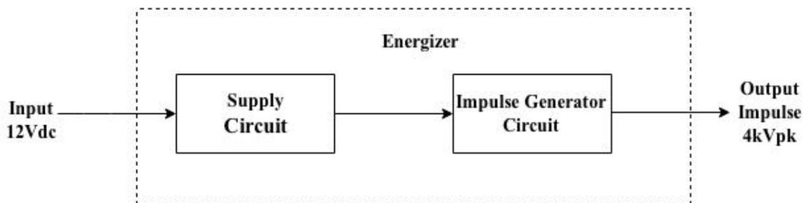
Figure 2.3: Energizer Block Diagram
