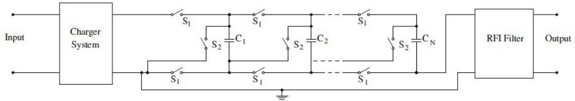
Figure 2.10: Marx generator type pulse generator
