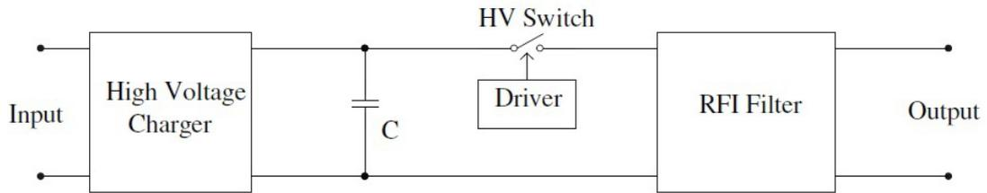
Figure 2.8: Direct discharge type pulse generator
