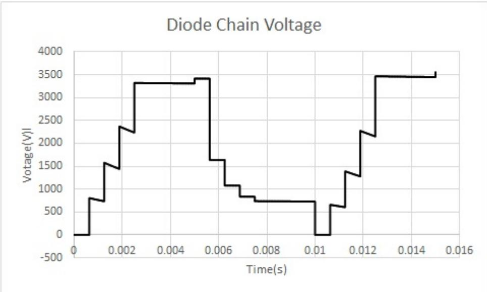
Figure 6.6: Voltage Across Diode Chain
