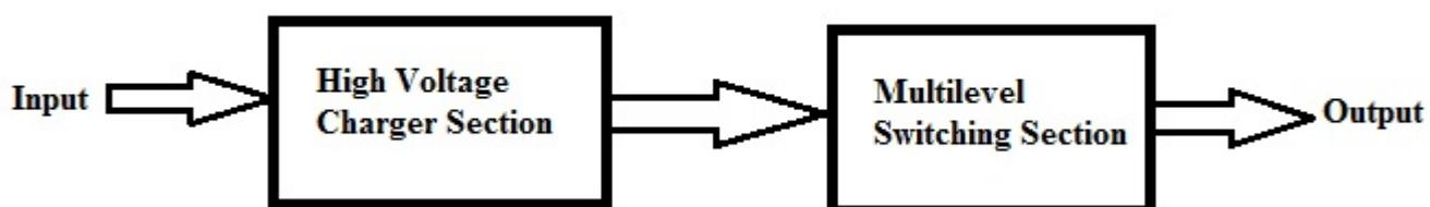
Figure 7.1: Block Diagram for Hardware Implementation
