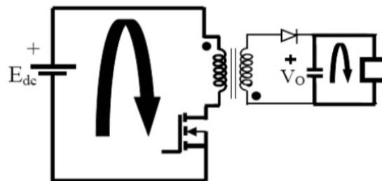
Figure 3.2: Flyback operation when switch is ON
