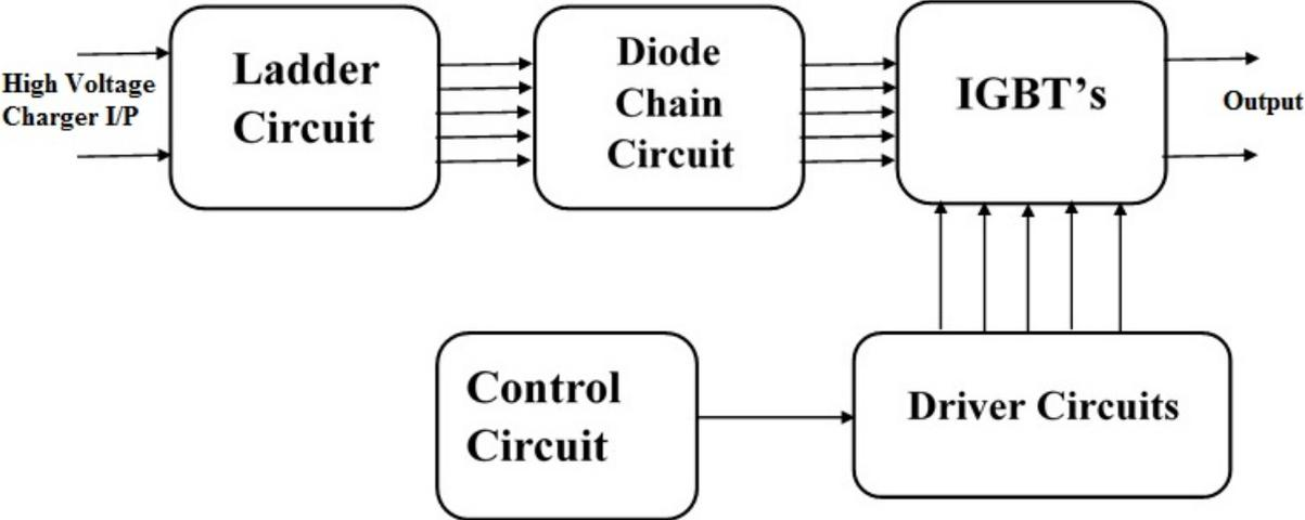
Figure 7.2: Multilevel Topology Hardware Arrangement
