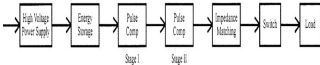
Figure 2.1: General Block Diagram of Pulsed Power Train
