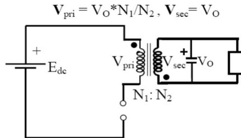
Figure 3.5: Flyback operation when switch is OFF
