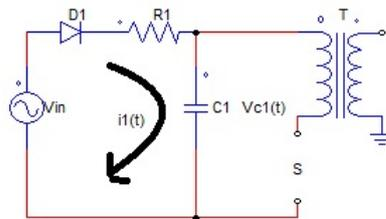
Figure 2.6: Charging of the capacitor
