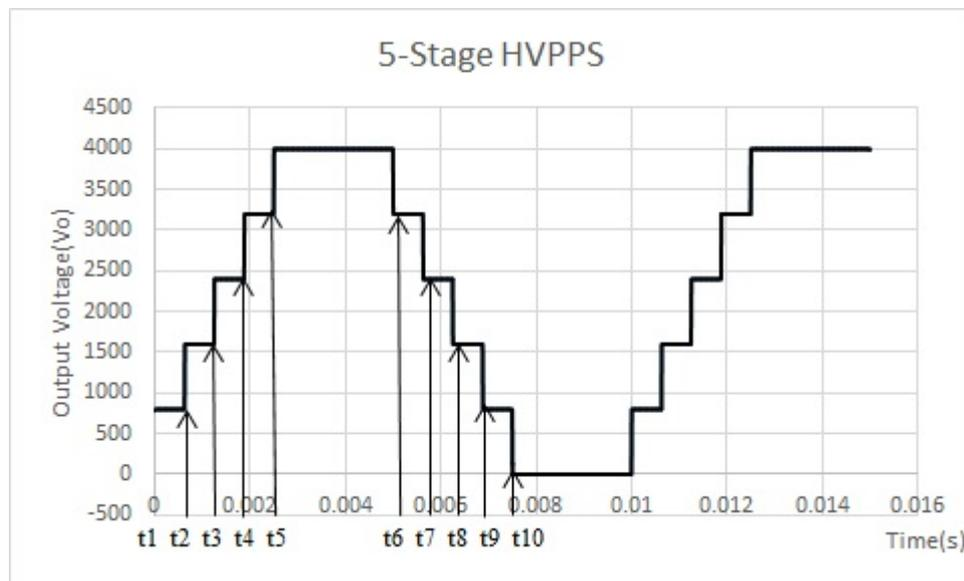
Figure 6.2: An output pulse generated by a 5-stage multi-level HVPPS
