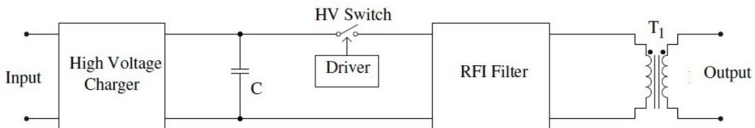
Figure 2.9: Pulse transformer type pulse generator
