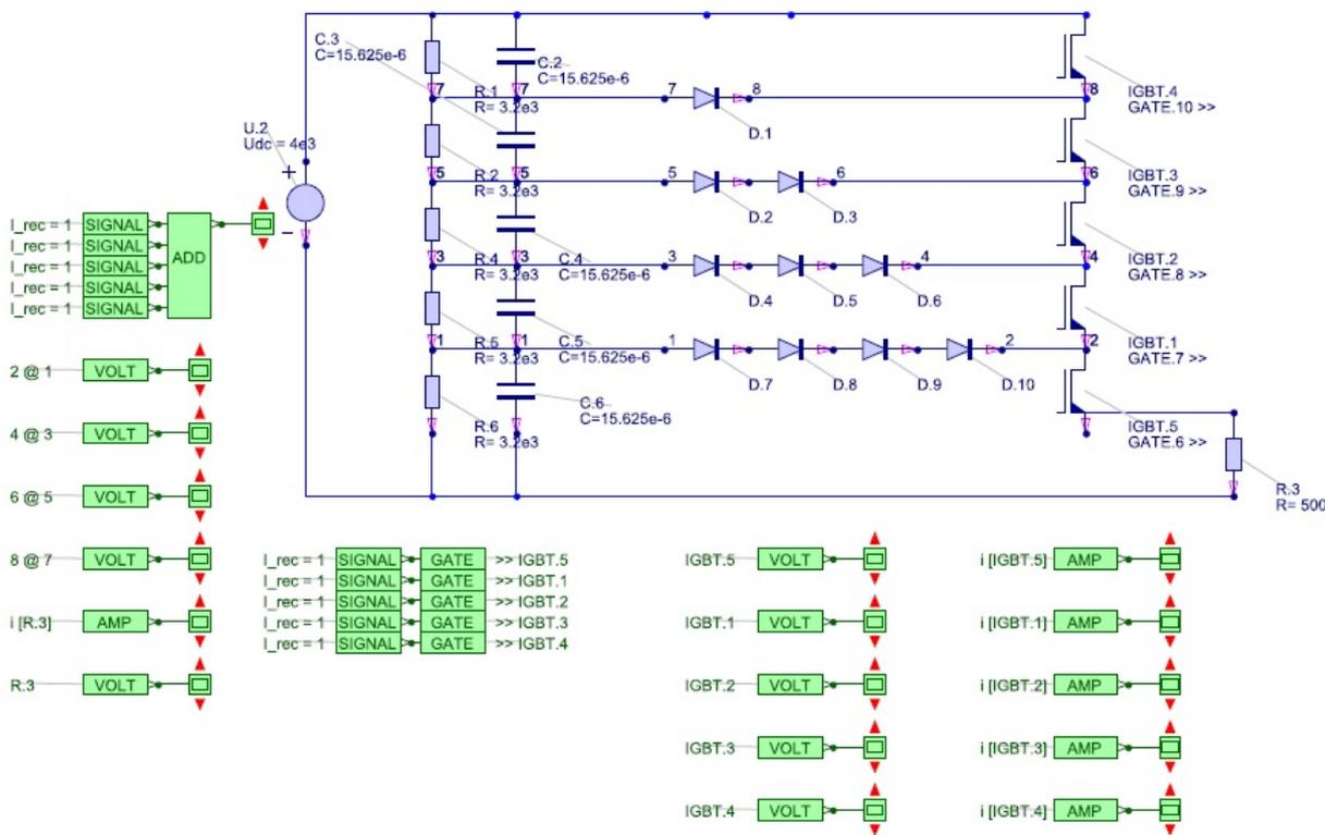
Figure 6.3: Gecko Simulation Circuit of 5 Level HVPPS
