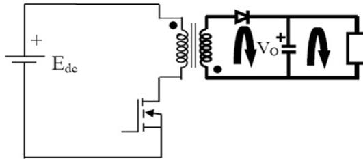
Figure 3.4: Flyback operation when switch is OFF
