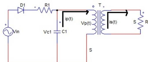
Figure 2.7: Discharge of the capacitor
