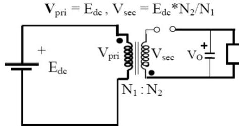
Figure 3.3: Equivalent circuit in ON condition
