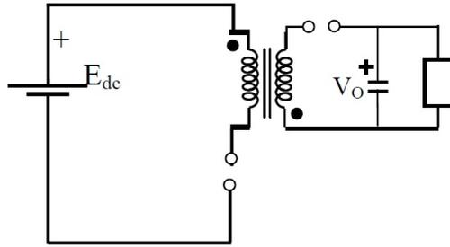
Figure 3.6: Flyback operation Mode 3(DCM)
