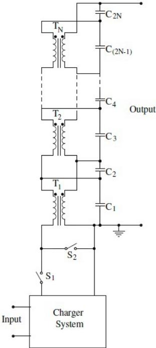
Figure 2.11: Vector inverse type pulse generator
