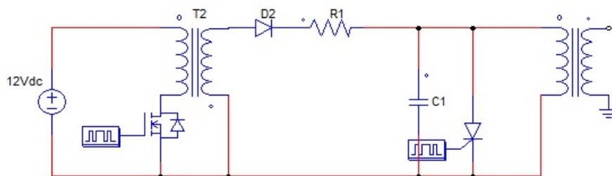
Figure 2.5: Supply circuit using flyback converter
