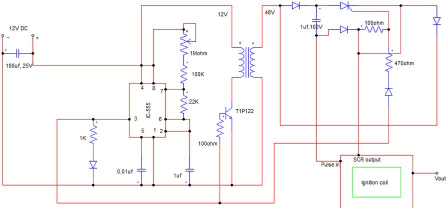
Figure 7.3: High Voltage Charger Circuit Using 555 Timer
