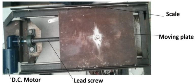
Figure 3.2 TIG welding fixture
