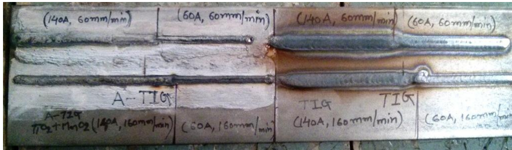
Figure 3.4 Appearance of a weld made on Stainless Steel 304L
