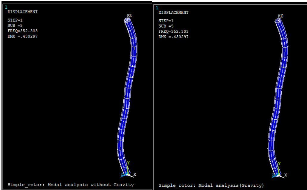
Figure 3.6: Mode 3(without spin- with/without gravity)
