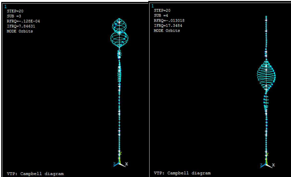
Figure 5.15: Whirl orbit for 7.8463Hz & 17.348Hz
