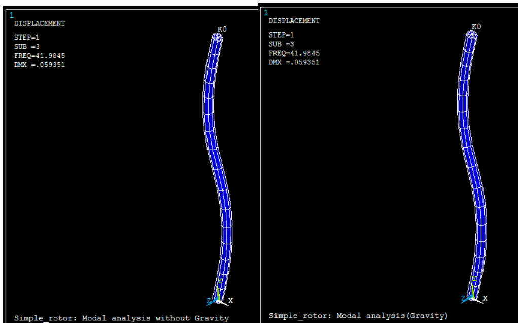
Figure 3.5: Mode 2(without spin- with/without gravity)
