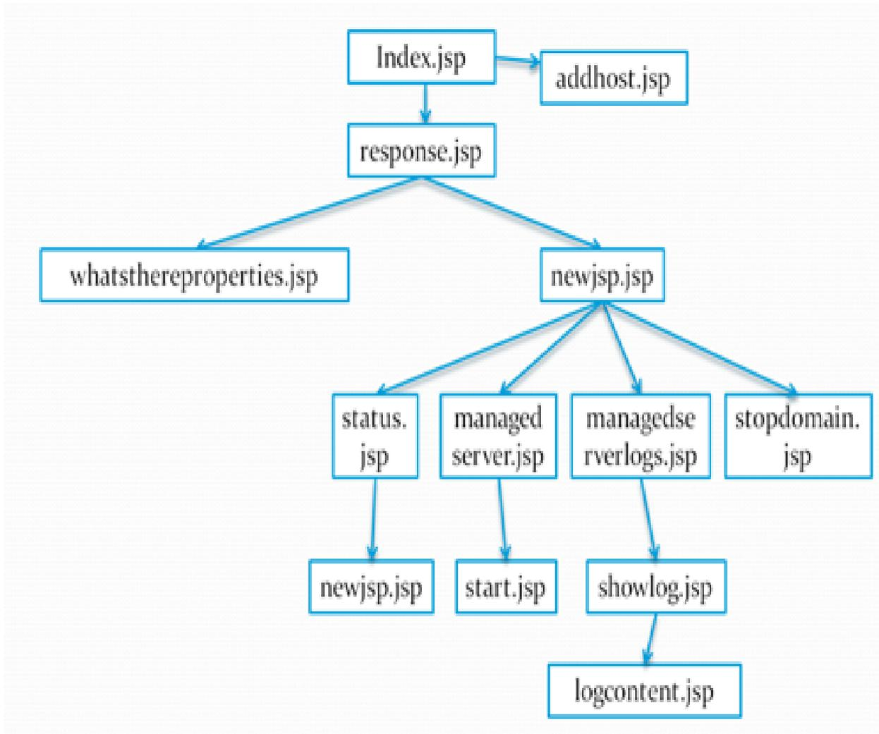
Figure 3.1: Transformation Application GUI Flow Chart
