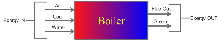
Figure 4.6: Exergy In and Out of Boiler
