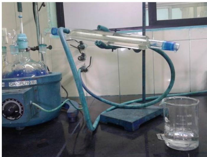
Figure 4.56: Distillation set up for [BMIm][BF 4 ]
