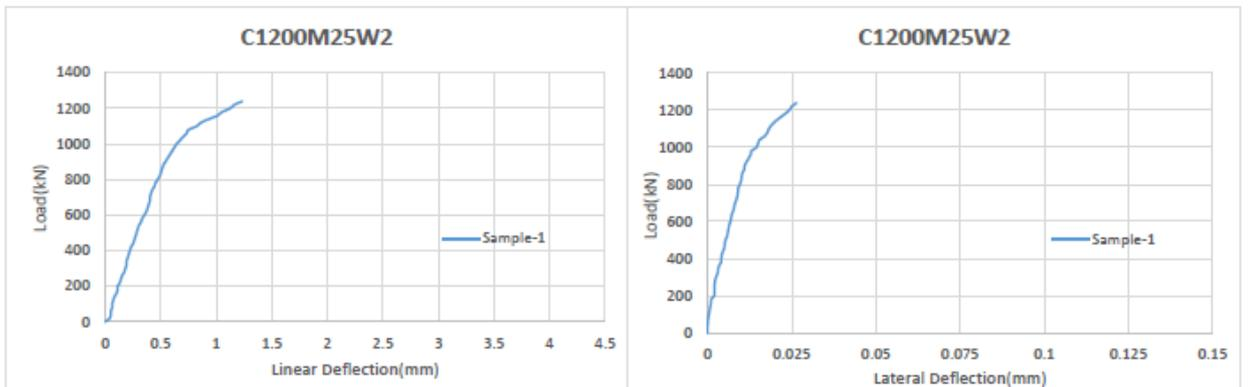
Figure 4.38: Linear and Lateral Deflection of column C1200M25W2
