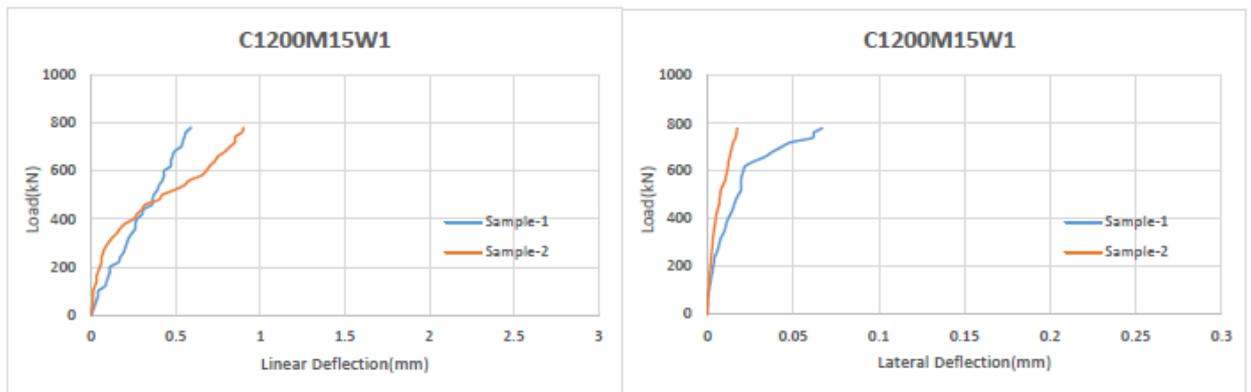
Figure 4.13: Linear and Lateral Deflection of column C1200M15W1
