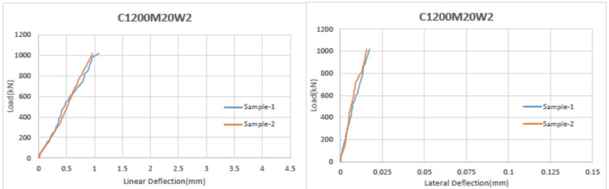
Figure 4.27: Linear and Lateral Deflection of column C1200M20W2
