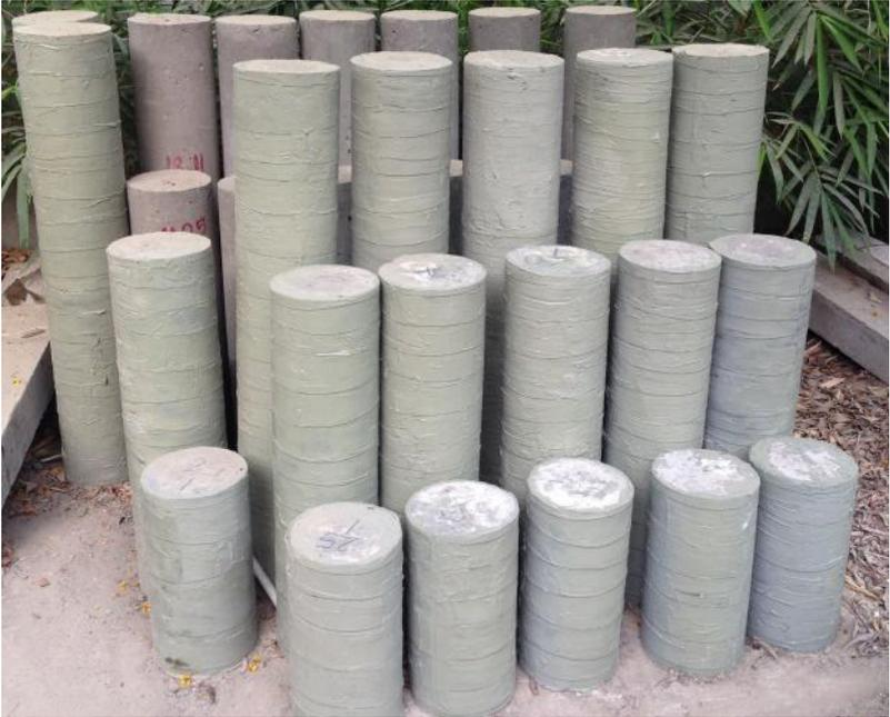
Figure 3.30: Wrapped Column Specimens
