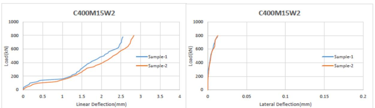
Figure 4.14: Linear and Lateral Deflection of column C400M15W2
