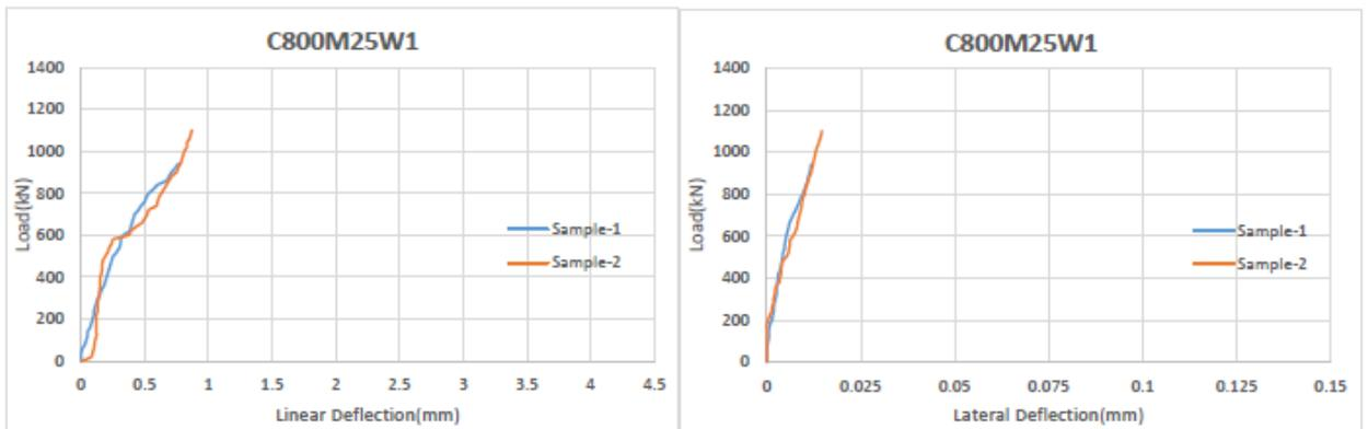
Figure 4.34: Linear and Lateral Deflection of column C800M25W1
