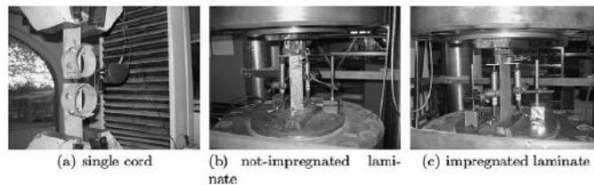
Figure 2.2: Tensile test on steel cord reinforcement
