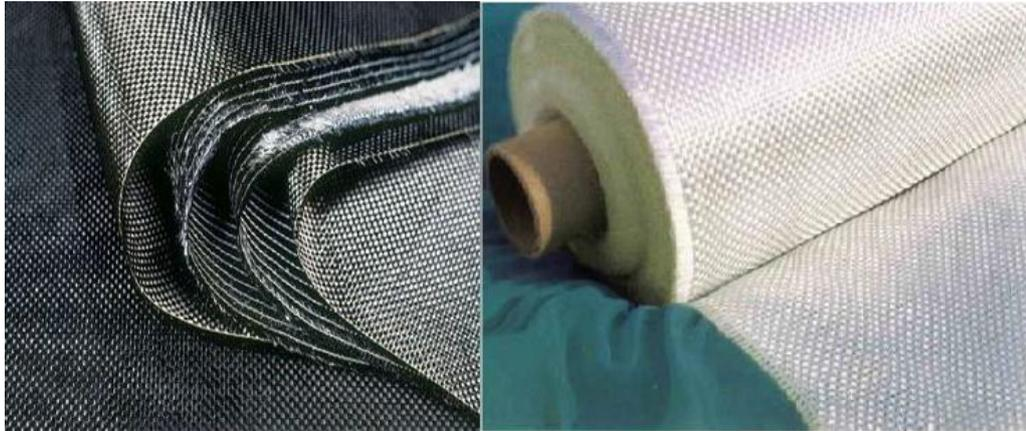
Figure 1.1: CFRP and GFRP sheet
