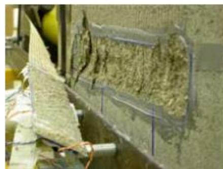
SRP Specimen - Concrete shearing
