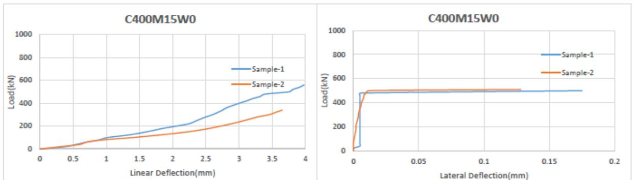
Figure 4.8: Linear and Lateral Deflection of column C400M15W0
