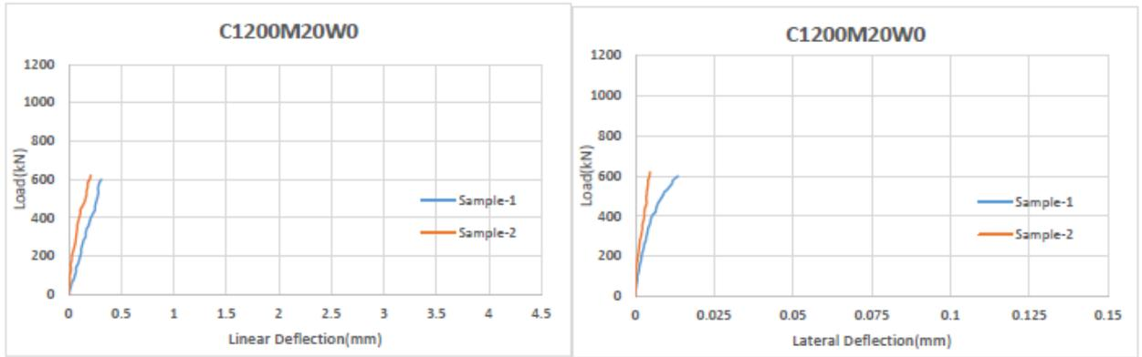
Figure 4.21: Linear and Lateral Deflection of column C1200M20W0
