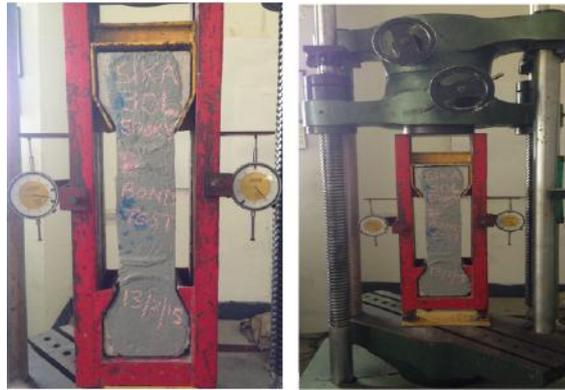
Figure 3.18: Dumbbell wrapped with Sikadur 30LP
