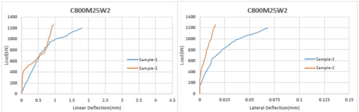
Figure 4.37: Linear and Lateral Deflection of column C800M25W2
