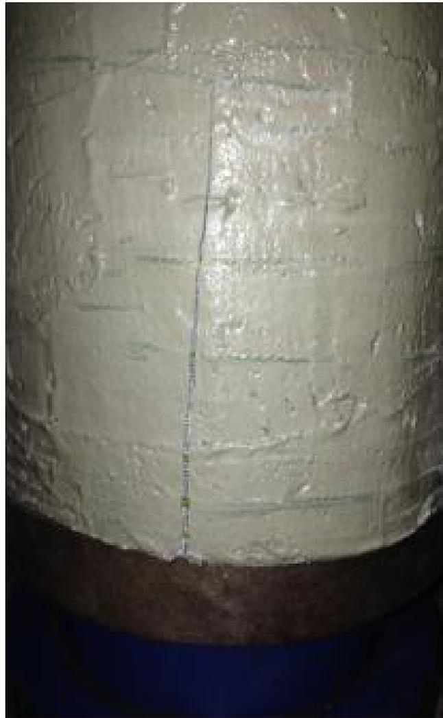
Figure 4.45: Crack Initiate in Column C1200M25W2
