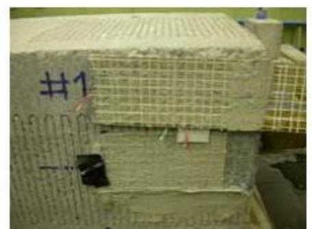
SRG Specimen - grout shearing
