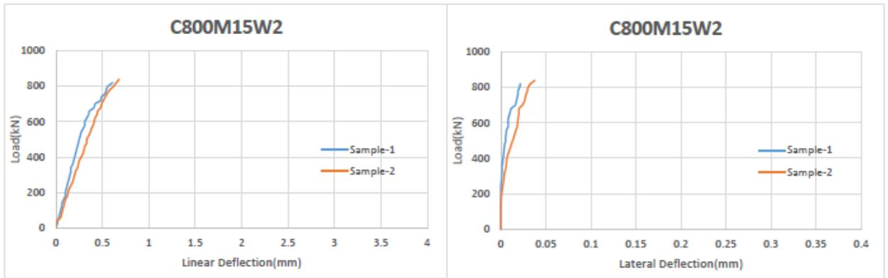
Figure 4.15: Linear and Lateral Deflection of column C800M15W2
