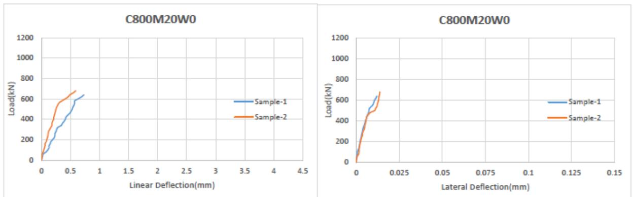
Figure 4.20: Linear and Lateral Deflection of column C800M20W0
