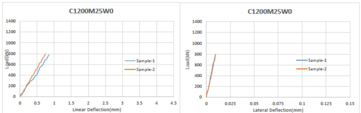
Figure 4.32: Linear and Lateral Deflection of column C1200M25W0
