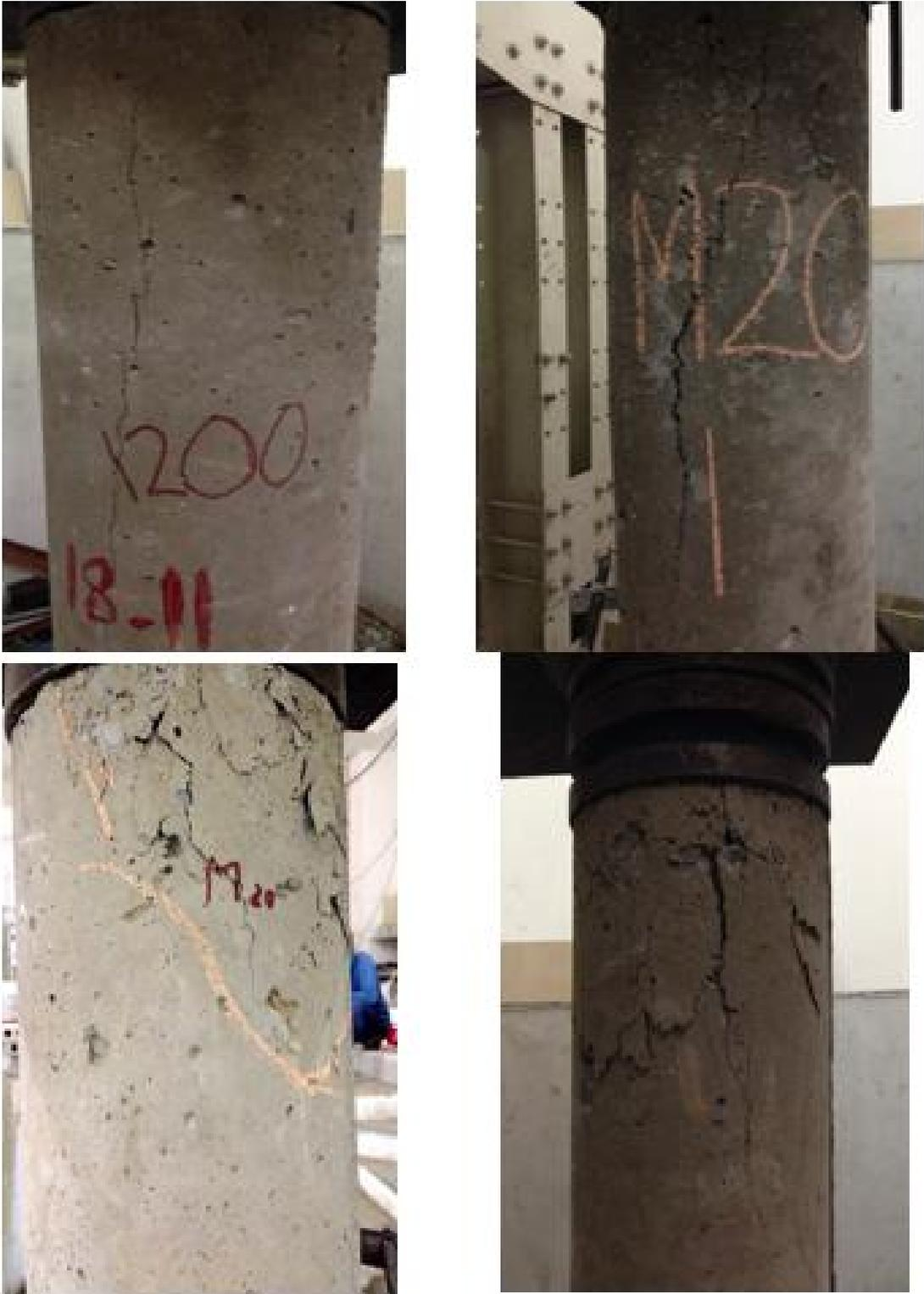
Figure 4.42: Shear Failure Pattern of Column C1200M20W0 and Shear Cracks from Top of Column C800M15W0
