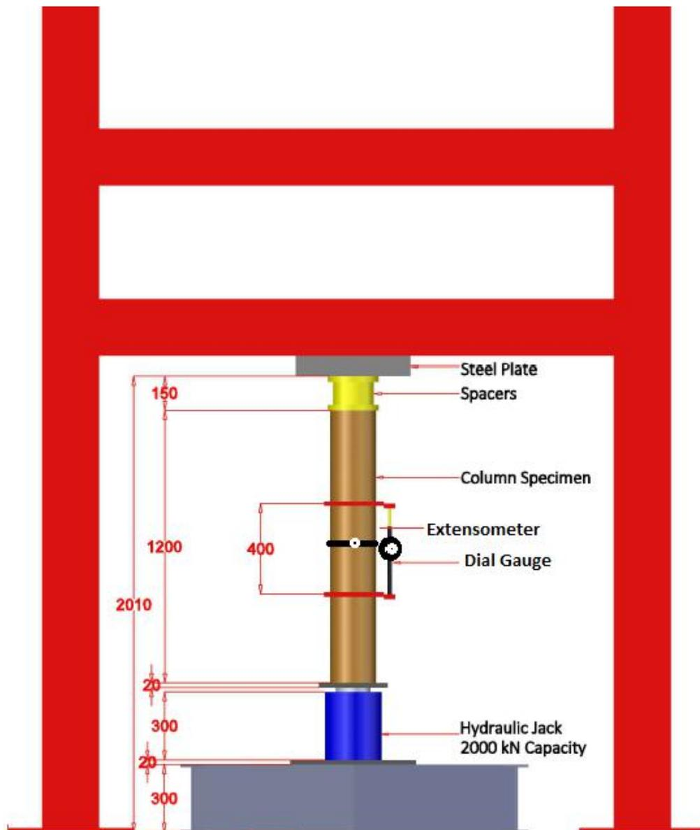
Figure 3.31: Test Setup
