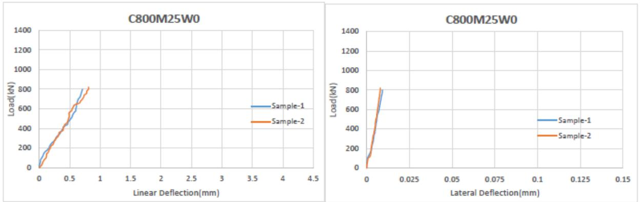
Figure 4.31: Linear and Lateral Deflection of column C800M25W0
