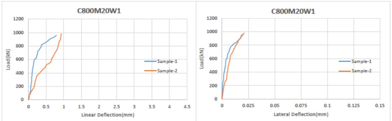
Figure 4.23: Linear and Lateral Deflection of column C800M20W1
