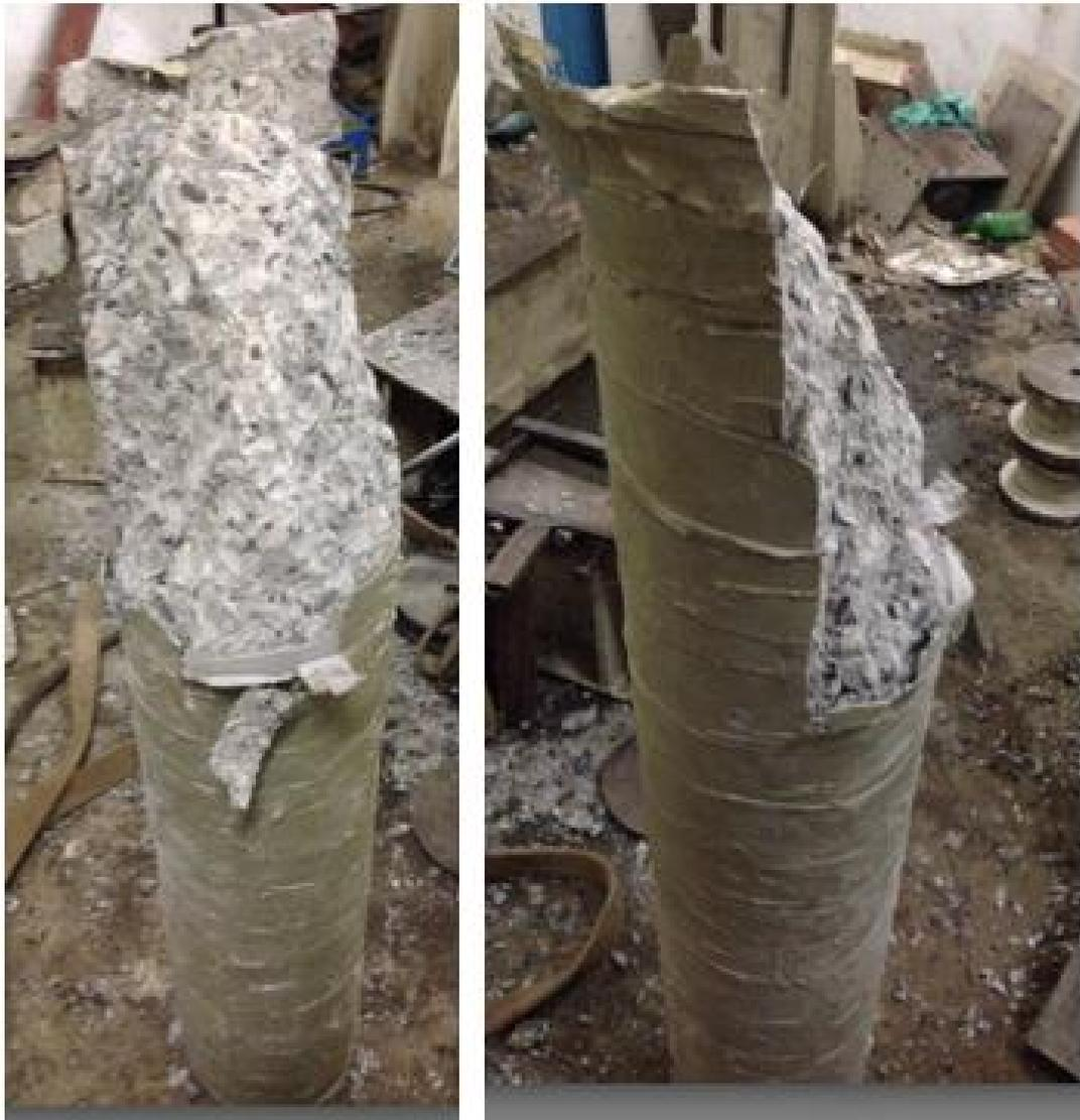
Figure 4.43: Shear Failure Pattern in Column C800M20W1
