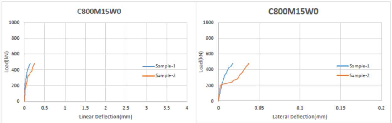
Figure 4.9: Linear and Lateral Deflection of column C800M15W0
