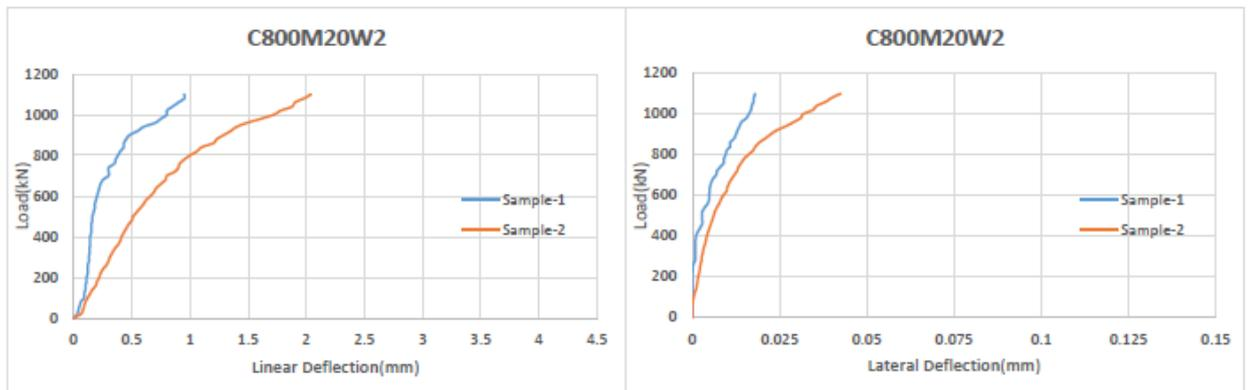
Figure 4.26: Linear and Lateral Deflection of column C800M20W2
