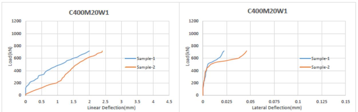
Figure 4.22: Linear and Lateral Deflection of column C400M20W1
