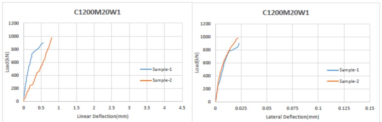
Figure 4.24: Linear and Lateral Deflection of column C1200M20W1
