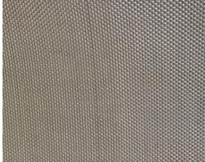
Figure 3.1: Wire mesh 40x32
