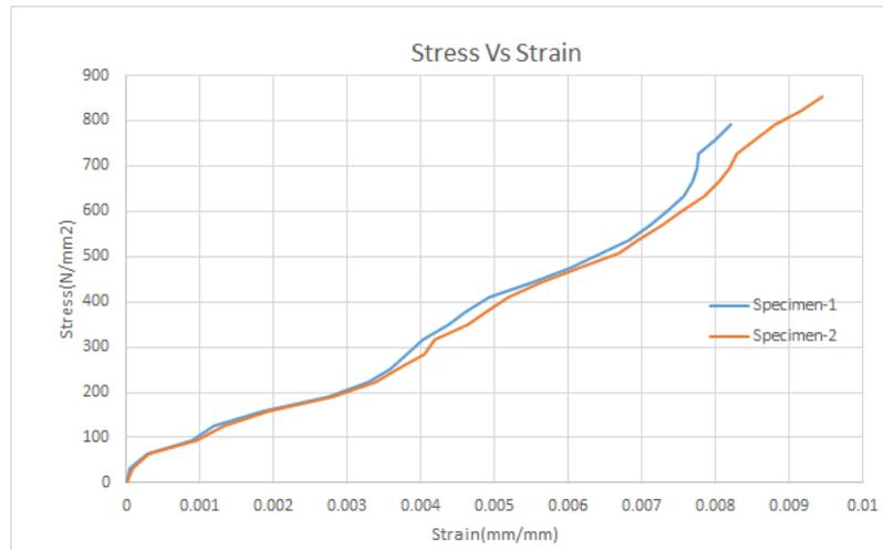
Figure 3.19: Stress Vs Strain (Bond Test)[Sikadur 30LP]
