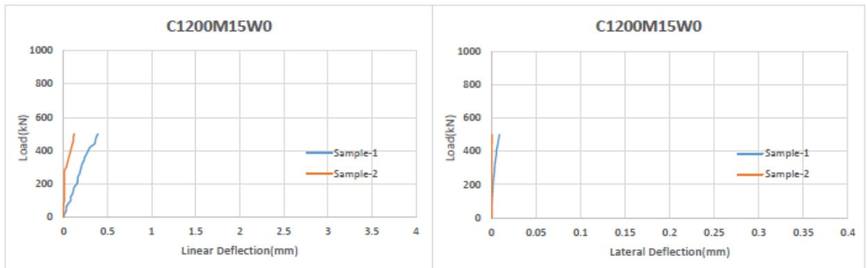
Figure 4.10: Linear and Lateral Deflection of column C1200M15W0
