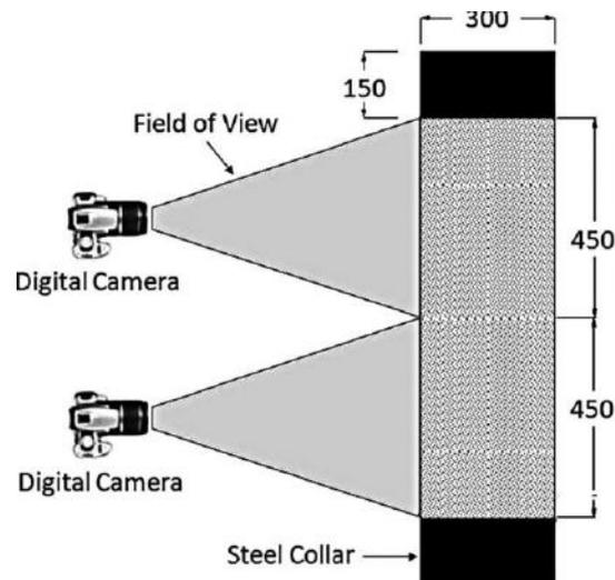
Figure 2.4: DICT test setup
