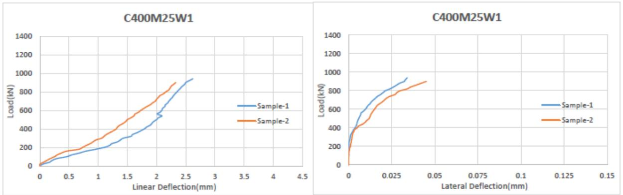
Figure 4.33: Linear and Lateral Deflection of column C400M25W1
