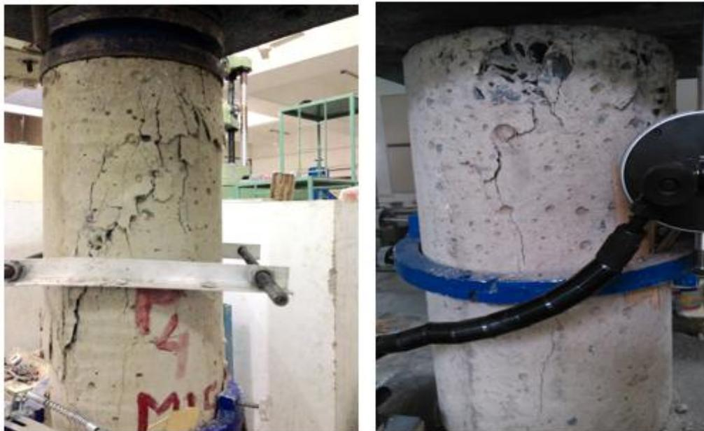
Figure 4.41: Spalling of Concrete and Crushing of Concrete Column C400M15W0
