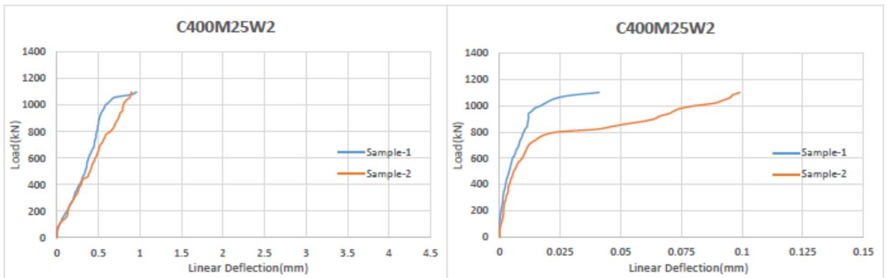
Figure 4.36: Linear and Lateral Deflection of column C400M25W2
