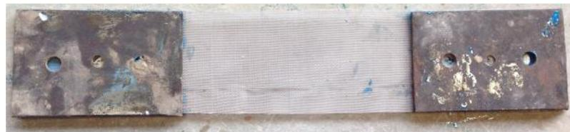
Figure 3.7: Tension test Sample
