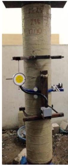
Figure 3.33: Dial gauge for vertical displacement
