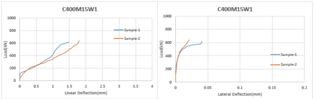
Figure 4.11: Linear and Lateral Deflection of column C400M15W1
