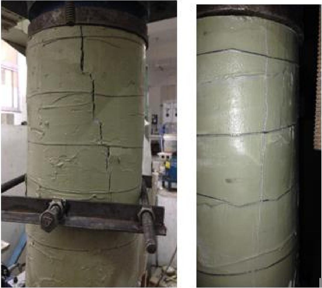
Figure 4.47: Crack Propagate in Vertical Direction in Column C1200M20W2
