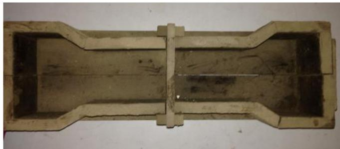
Figure 3.13: Dumbbell Shape Mould
