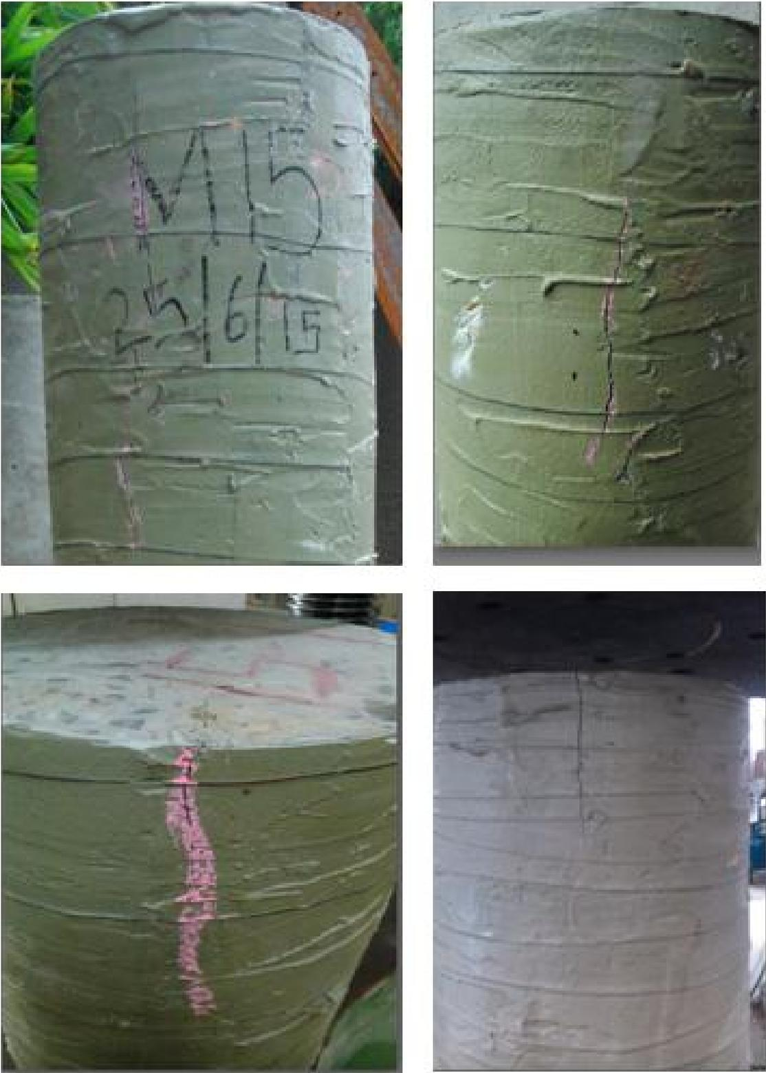
Figure 4.44: Crack generation in Column C800M15W1 and C400M25W1
