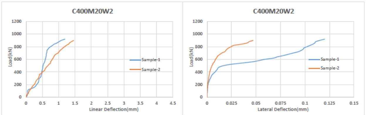
Figure 4.25: Linear and Lateral Deflection of column C400M20W2
