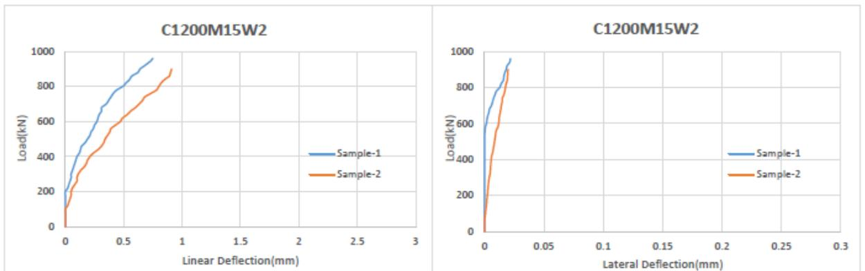
Figure 4.16: Linear and Lateral Deflection of column C1200M15W2
