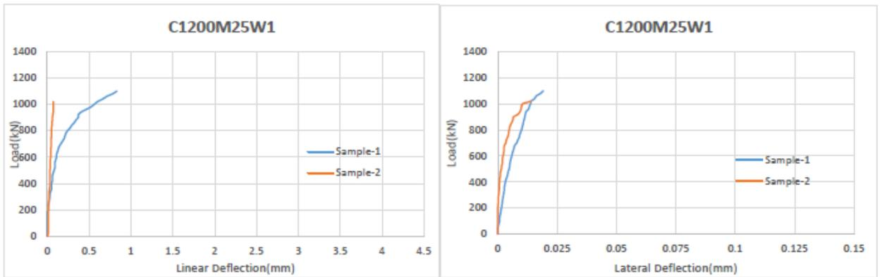
Figure 4.35: Linear and Lateral Deflection of column C1200M25W1
