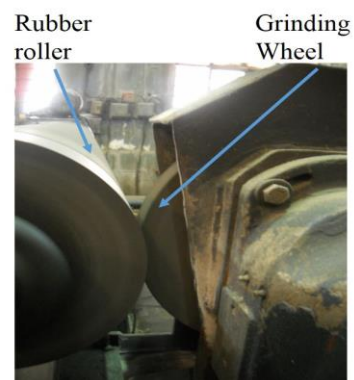
Figure 3. Face grinding of rubber roller on grinding machine
