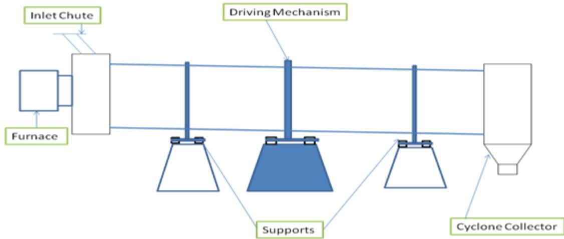
Fig.1 Concurrent Industrial Drum Dryer
