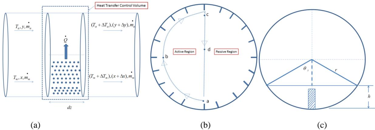
Fig 2 (a) CV for calculating Heat and Mass Transfer (b) Number of Flights taking part in drying (c) Geometry of a single Flight
