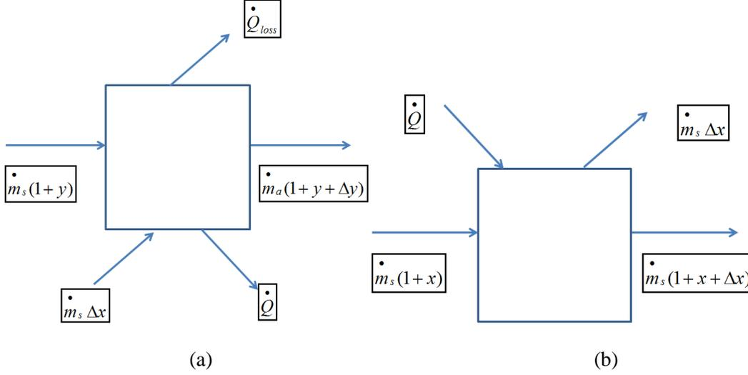
Fig. 2 (a) Gypsum Control Volume (b) Air Control Volume
