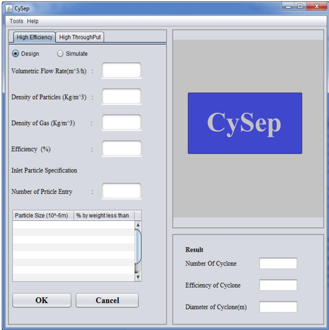
Figure 1. Snapshot of Graphic User Interface of 'CySep'.
