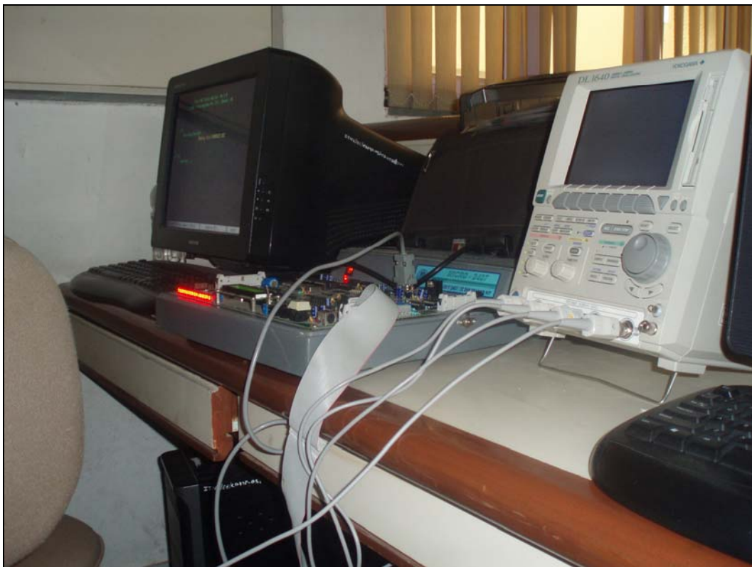
Fig. 10.8 Pictorial view of setup for generation of PWM signals from MICRO-2407 kit
