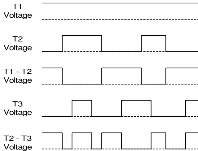
Figure 4.2: Pulse Width Modulation waveforms for hoist
