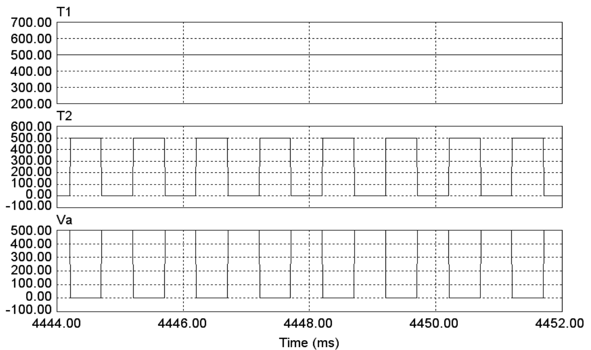
Figure 5.16: (a) T1 Terminal voltage (b) T2 Terminal voltage (c) Armature across voltage
