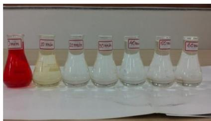
Figure 5.8.4a % Color removal for RR2 using Ti/Ceo-RuO<sub>2</sub>
