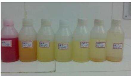
Figure 5.8.4 b %Color removal for RR195 using Ti/Ceo-RuO<sub>2</sub>
