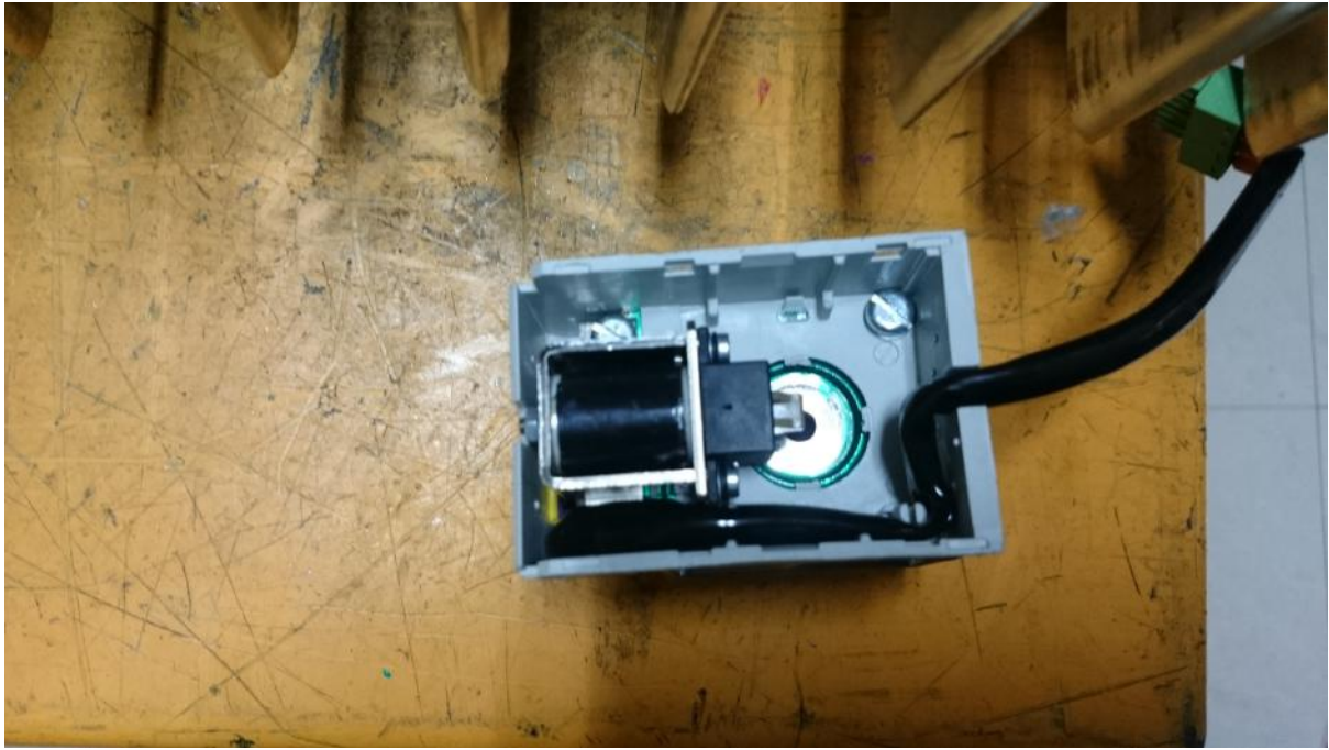
Figure 4.5: Clutch Coil of single phase UVR
