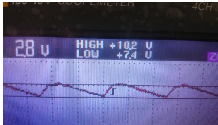
Figure 6.10: Rectifier output with ripples
