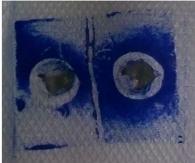
Figure 7.11: Carbon paper testing for cleaned joint with slot
