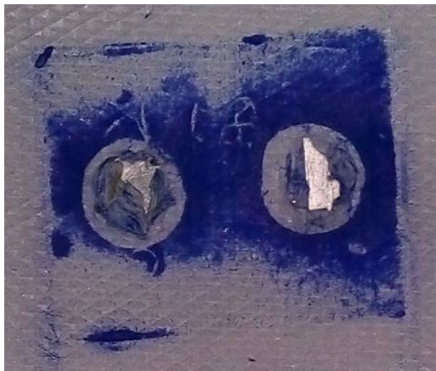
Figure 7.10: Carbon paper testing for cleaned joint without slot
