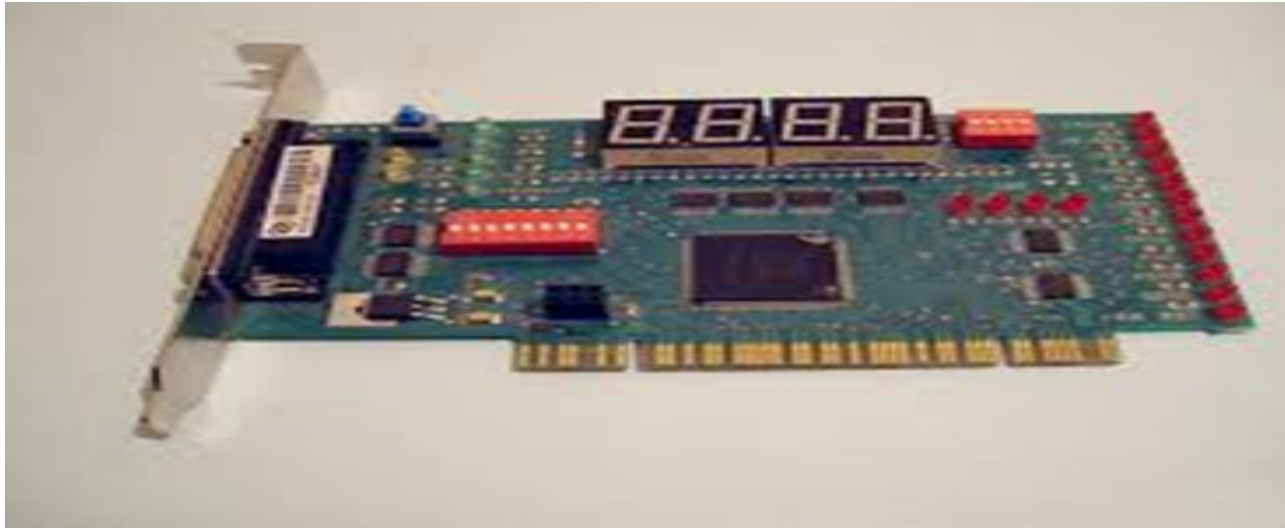
Fig. 4.1: BIOS POST Code in Board [6]
