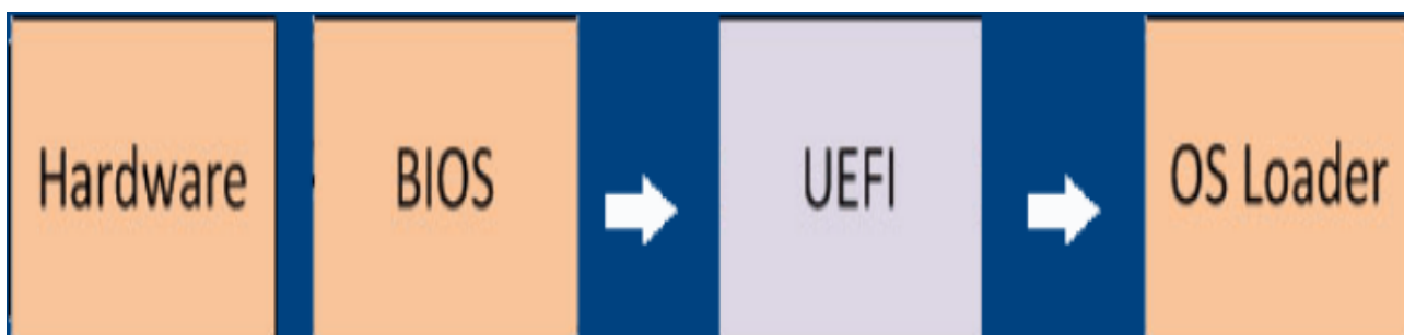
Fig. 2.3: UEFI Interface between BIOS and OS Loader [4]
