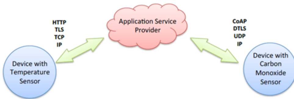
Figure 2.4: Device-to-cloud communication model diagram.
