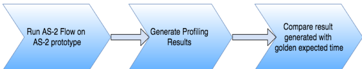
Figure 4.11: Test for Performance Checking of AS-2 prototype[2]
