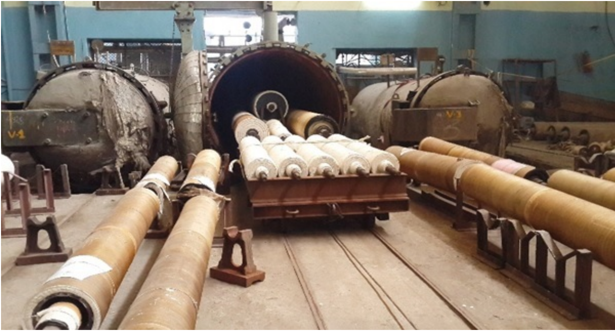
Figure 1.2: View of a loaded autoclave
