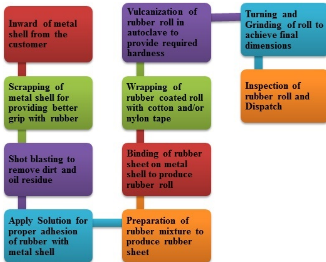
Figure 1.3: Process flow of rubber roll manufacturing industry
