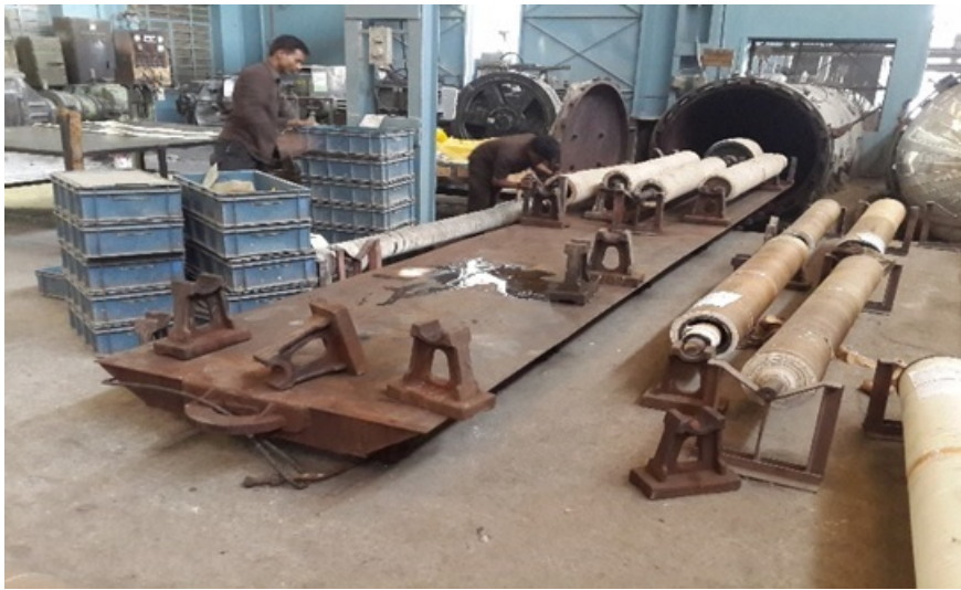
Figure 1.4: Existing trolley for putting rubber rolls inside autoclave
