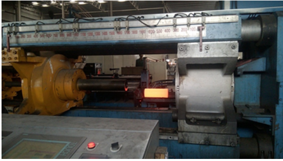
Figure 3.20: Hot extrusion process photo courtesy shera industry
