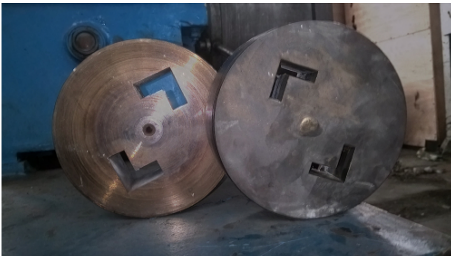
Figure 5.4: Extrusion Die alloy steel H-13 at 0 degree entry angle
