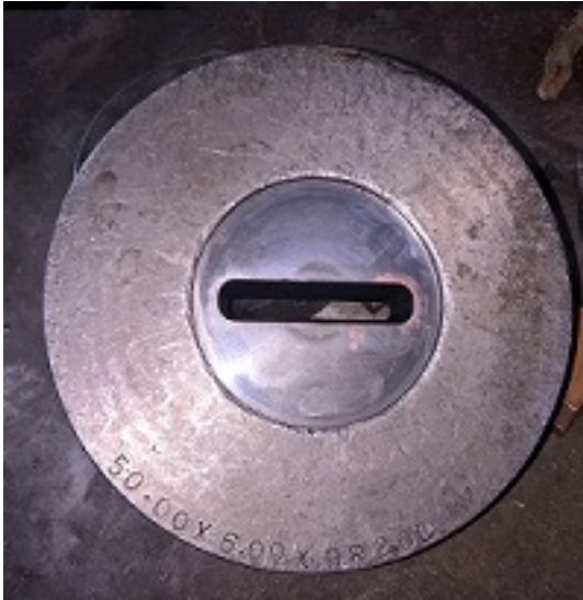
Figure 3.15: Cold drawing H-13 Alloy steel die photo courtesy shera industry
