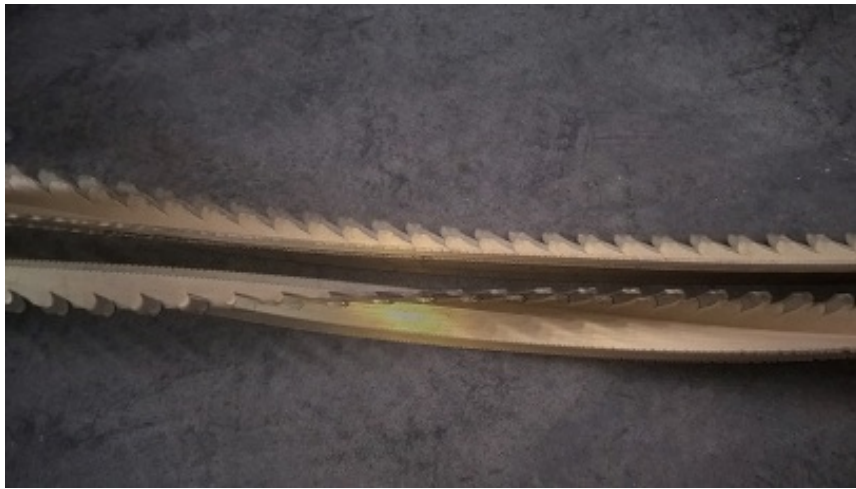
Figure 5.2: Cracked product 0 degree at entry angle
