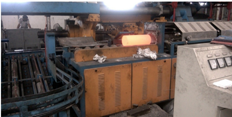
Figure 3.19: Hot extrusion process photo courtesy shera industry
