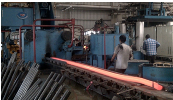
Figure 3.22: Hot extrusion process photo courtesy shera industry
