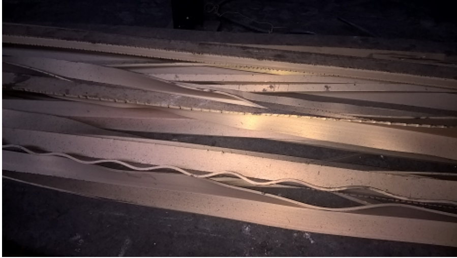
Figure 5.5: Cracked product at 5 degree entry angle
