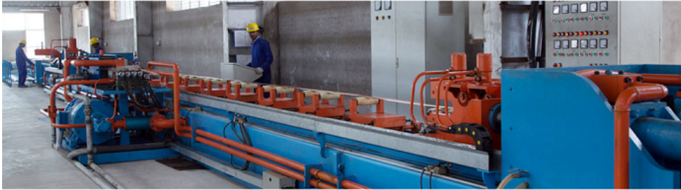
Figure 3.7: Double cylinder heavy duty hydraulic draw bench machine photo courtesy shera industry
