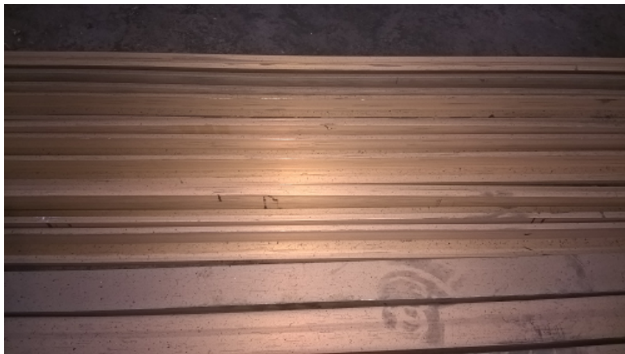
Figure 5.7: Finished product at 9 degree entry angle
