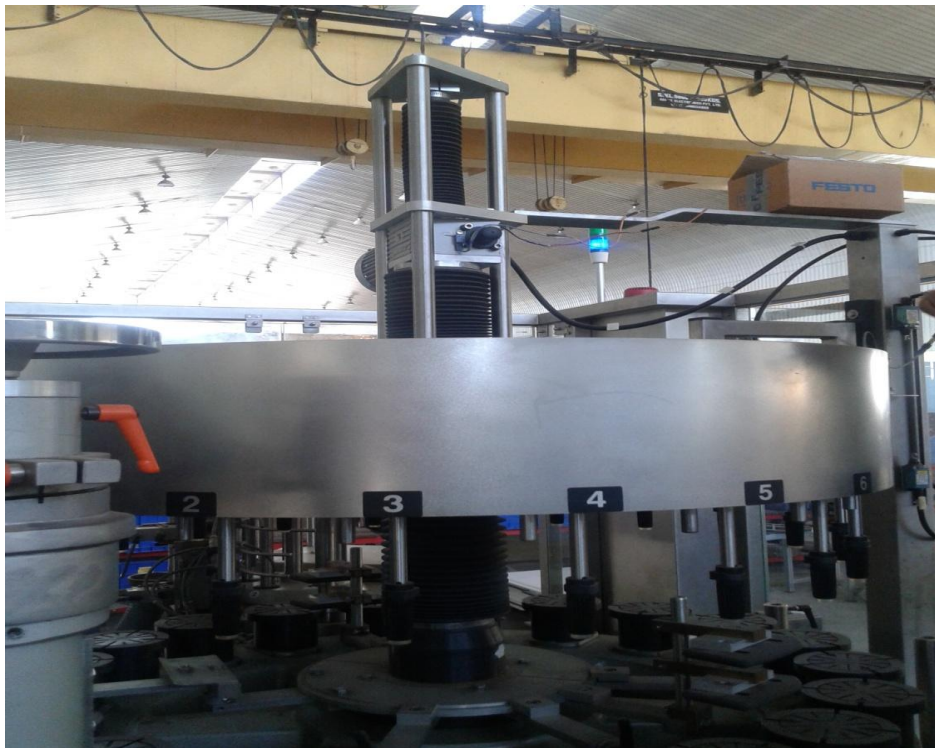
Figure 3.15 Mounting of Accelerometer on Carousel shaft
