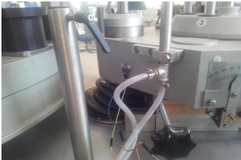
Figure 3.14 Mounting of Accelerometer on Aggregate
