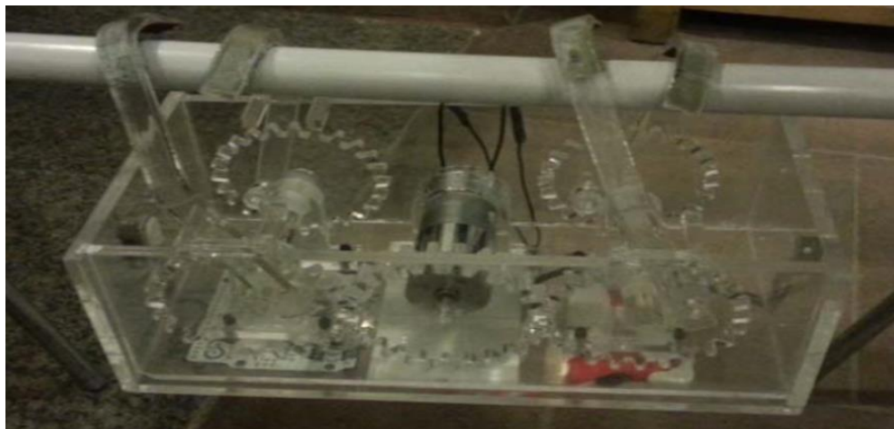
Figure 4: Robot inspired from sloth's walking style [4]
