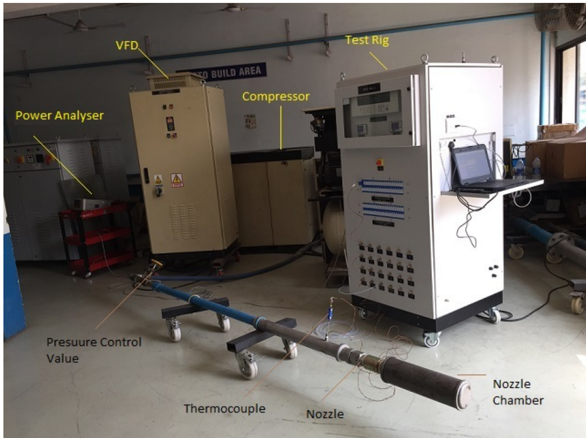
Figure 3.11: Experimental setup for performance of screw compressor
