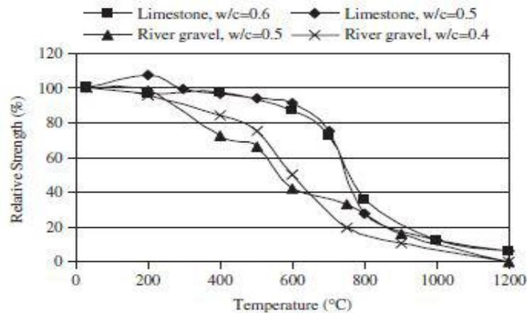
Figure 2.8: Relative Compressive Strength of Concrete Mixes after Exposed to Elevated Temperatures
