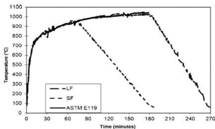
Figure 2.10: Different Time-Temperature Curves Adopted for Experimental Study
