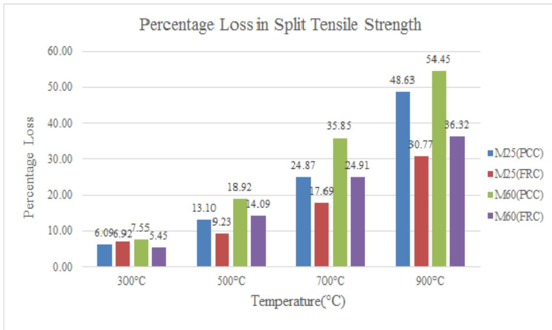
Figure 4.11: % Loss in Split Tensile Strength at Different Elevated Temperatures as Compared to Unheated Specimens
