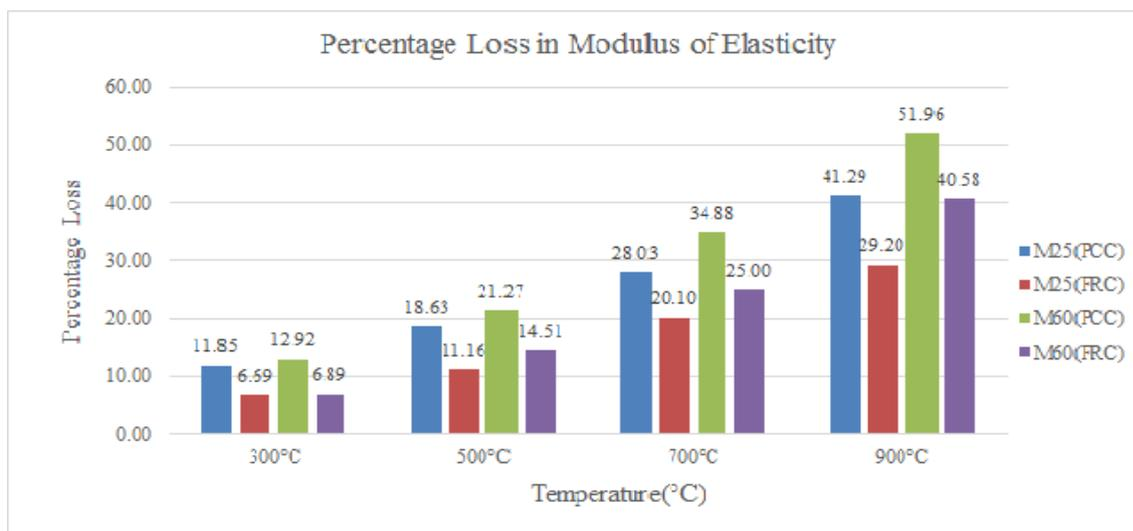
Figure 4.14: % Loss in Modulus of Elasticity at Different Elevated Temperatures as Compared to Unheated Specimens
