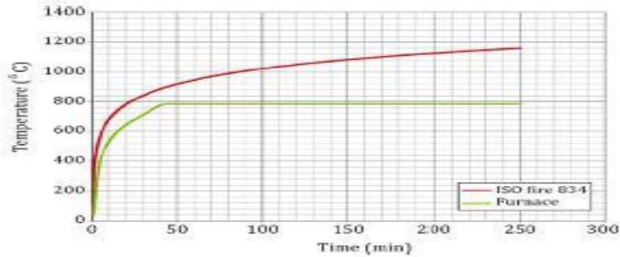
Figure 2.5: Graphical Representation of Experimental Curve & ISO-834 Curve
