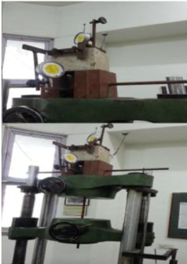
Figure 3.19: Bond Strength Test of Reinforced Concrete
