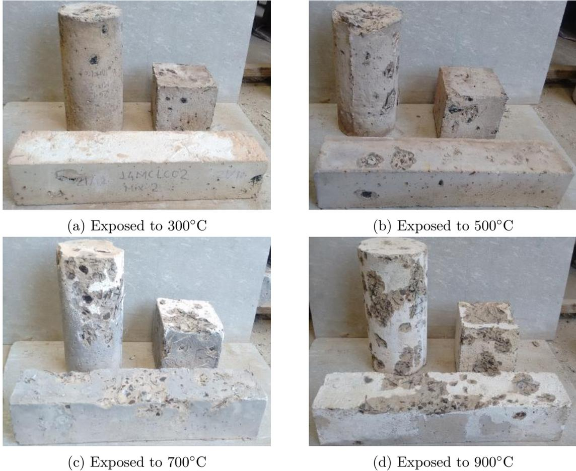
Figure 4.2: M25(FRC) Subjected to Different Elevated Temperatures
