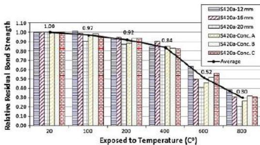
(c) Bond strength degradation for S420a Bars
