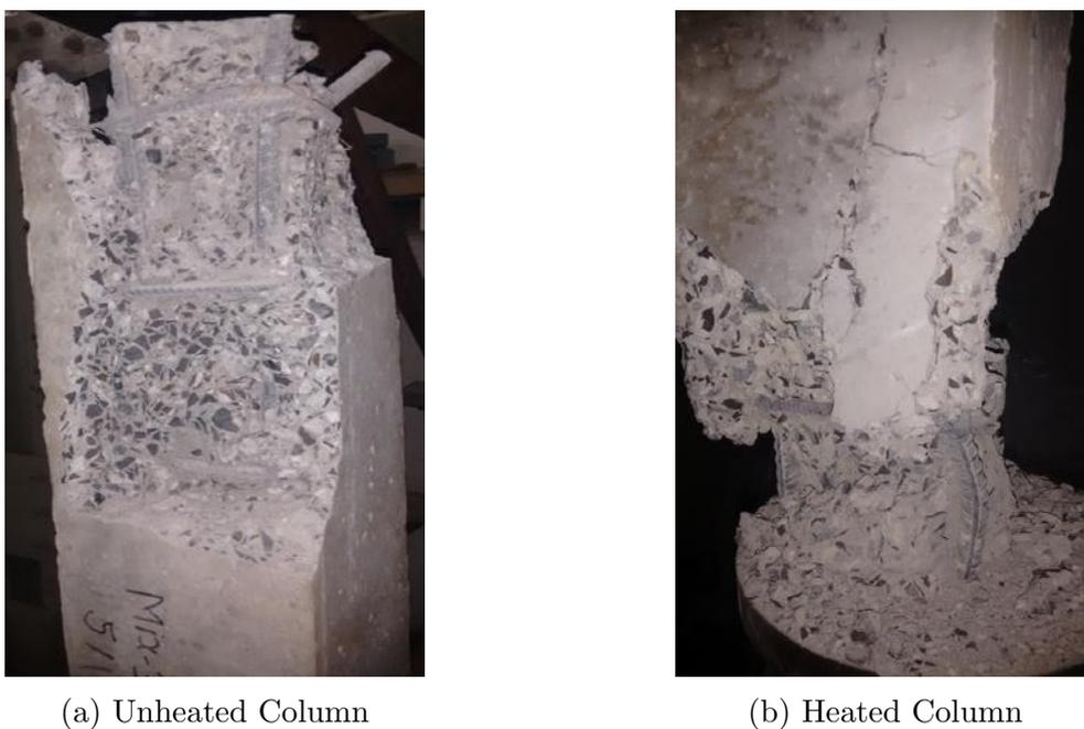
Figure 5.9: Failure of M60(PCC) Mix Column
