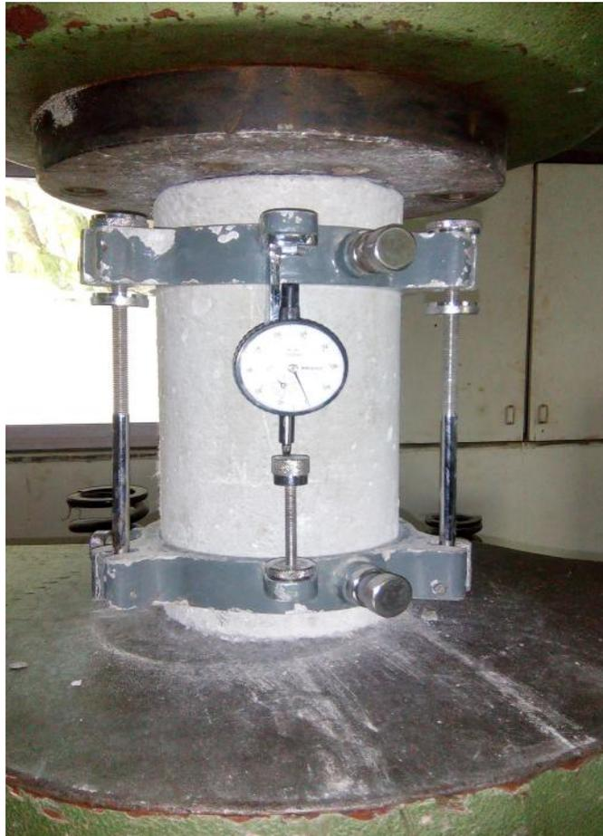
Figure 3.17: Test Setup for Modulus of Elasticity of Concrete
