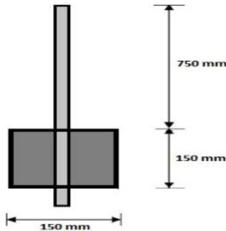
Figure 3.18: Bond Test Concrete Specimens
