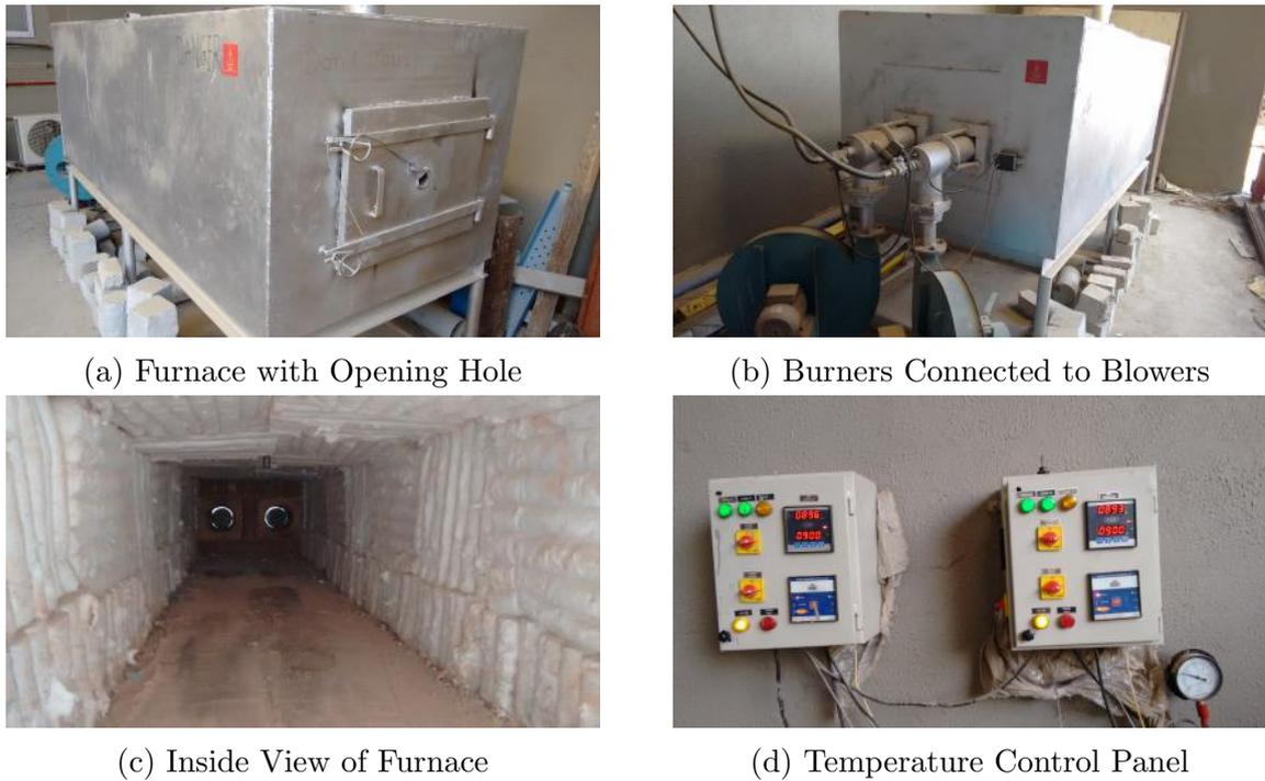
Figure 3.6: Various Elements of Gas Fired Furnace
