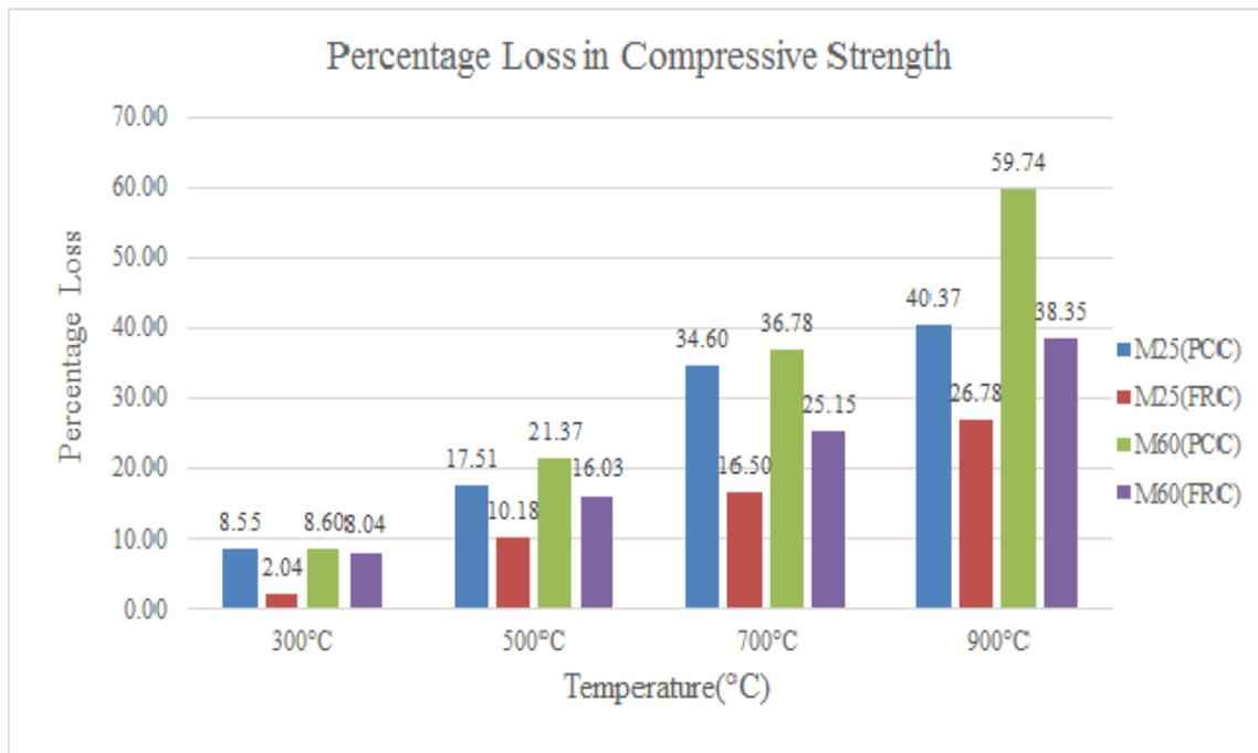
Figure 4.10: % Loss in Compressive Strength at Different Elevated Temperatures as Compared to Unheated Specimens
