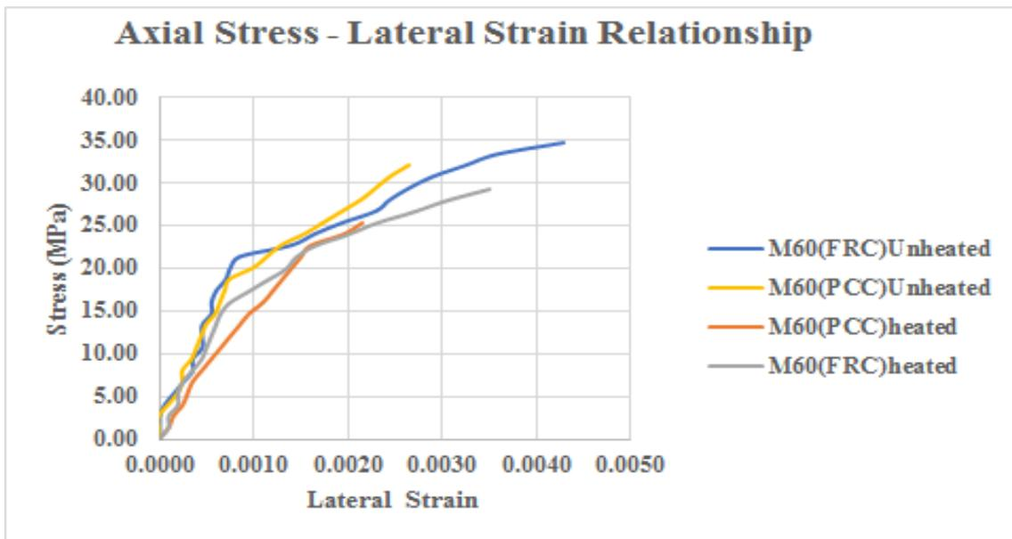
Figure 5.6: Axial Stress v/s Lateral Strain Relationship(M60)
