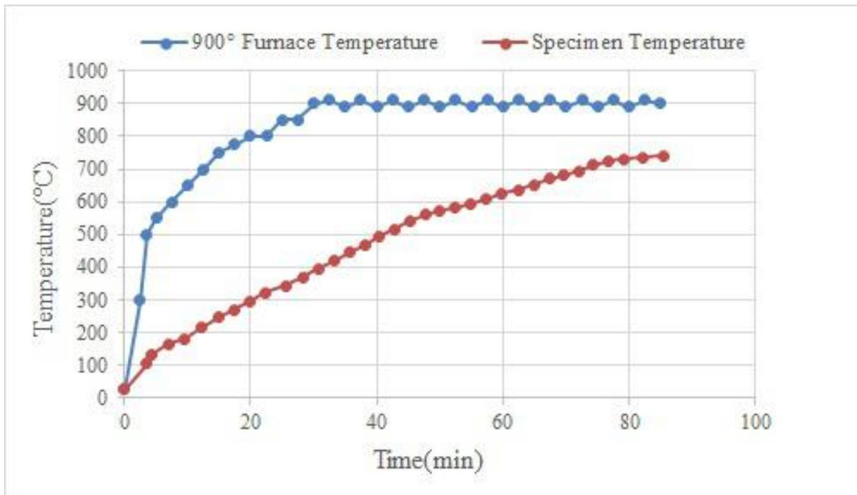
Figure 3.12: Rise in Specimens Temperature for 900°C Heating Regime
