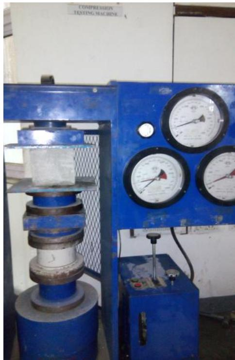
Figure 3.13: Plain Concrete Cube in Compression Testing Machine
