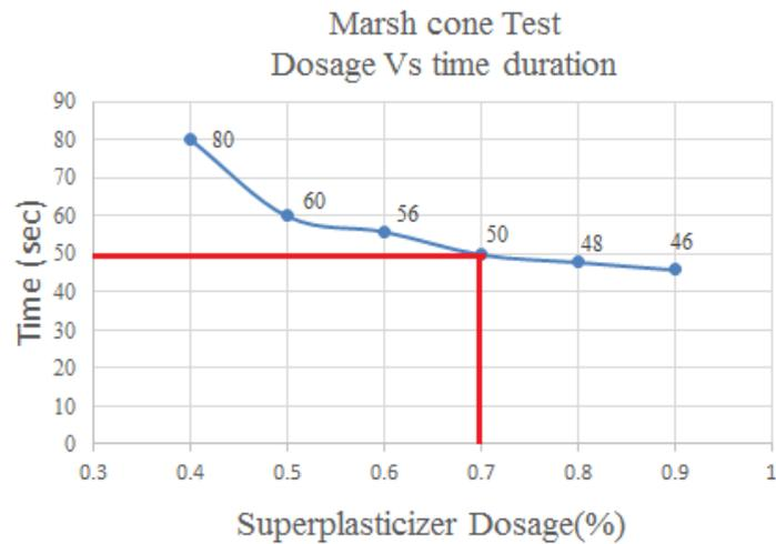
Figure 3.2: Marsh Cone Test
