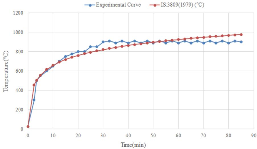
Figure 3.8: Graphical Representation of Experimental Curve & IS:3809(1979)[15] Recommended Curve
