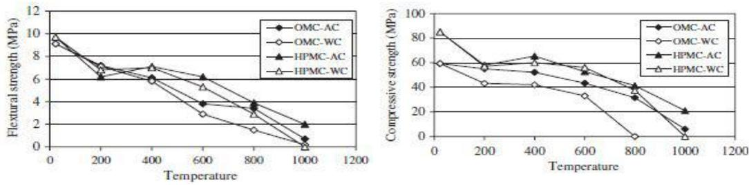
(a) Loss in Flexural Strength with Increase in Temperature (b) Loss in Compressive Strength with Increase in Temperature
