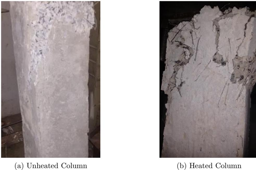
Figure 5.8: Failure of M25(FRC) Mix Column
