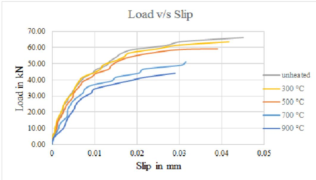
Figure 4.15: Load-Slip Curve for M25(PCC) Subjected to Different Elevated Temperatures
