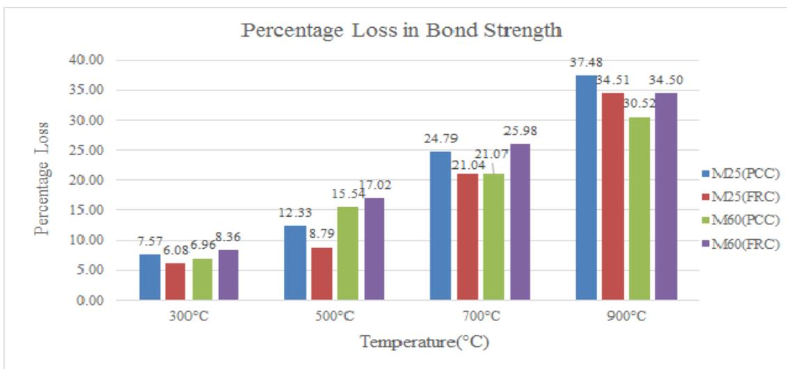
Figure 4.16: % Loss in Bond Strength at Different Elevated Temperatures as Compared to Unheated Specimens
