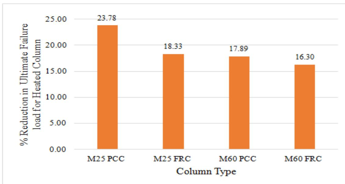
Figure 5.1: Percentage Reduction in Ultimate Failure Load for Heated Columns
