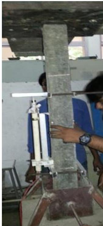
Figure 3.22: LVDT Attached on Column Specimen
