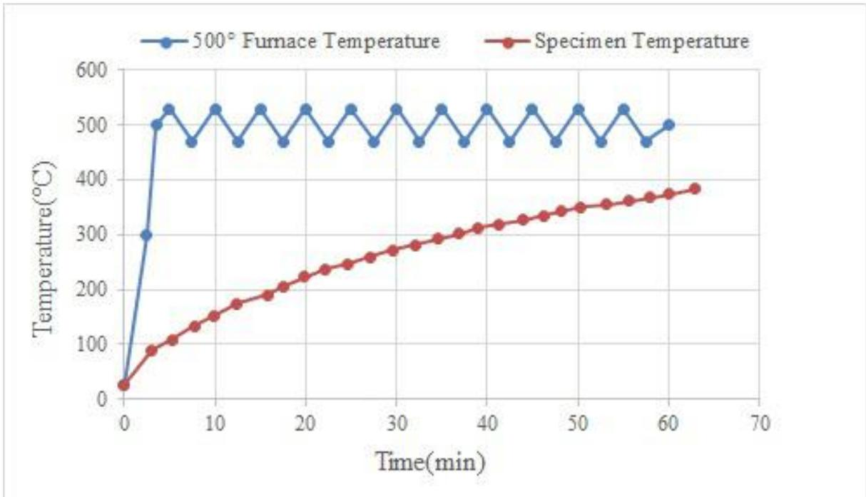
Figure 3.10: Rise in Specimens Temperature for 500°C Heating Regime
