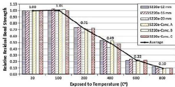
(b) Bond Strength Degradation for S220a Bars
