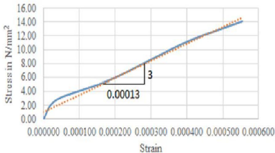
Figure 4.13: Graphical Representation of Stress v/s Strain Relation for M25(PCC) at 28 Days
