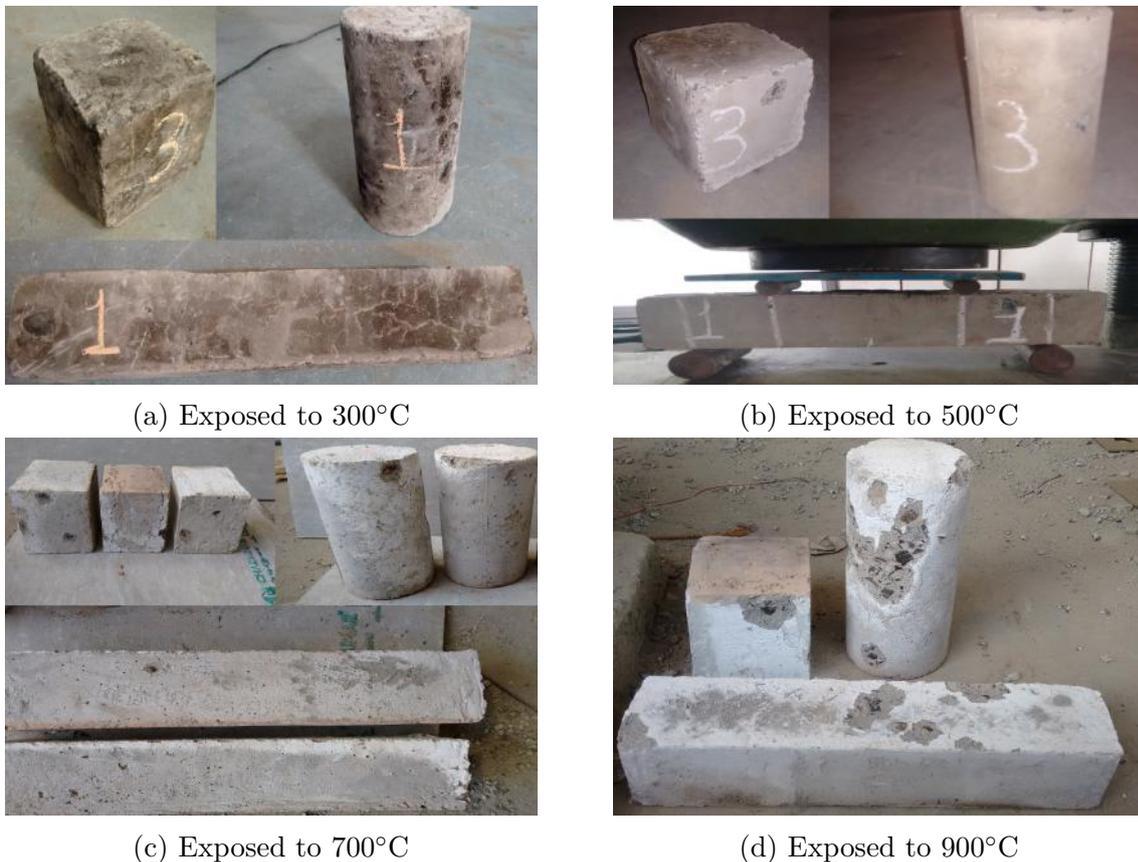
Figure 4.1: M25(PCC) Subjected to Different Elevated Temperatures
