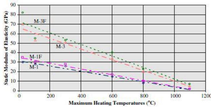
Figure 2.3: Loss in Modulus of Elasticity for Different Mixes at Elevated Temperatures
