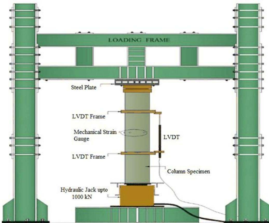
Figure 3.20: Test Set-up for RC Column
