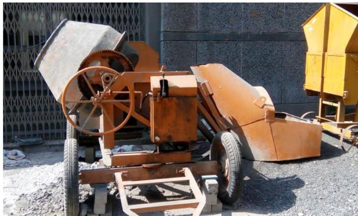
Figure 3.4: Concrete Drum Mixture
