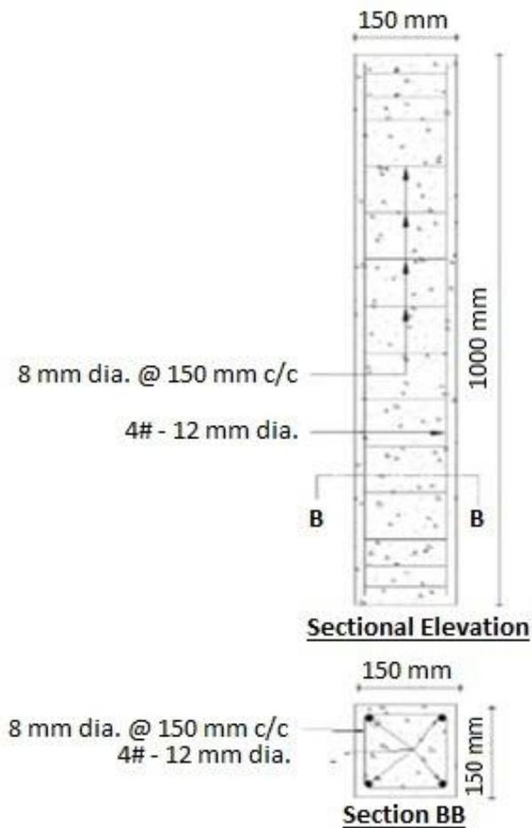
Figure 3.3: Reinforcement Detailing of Column
