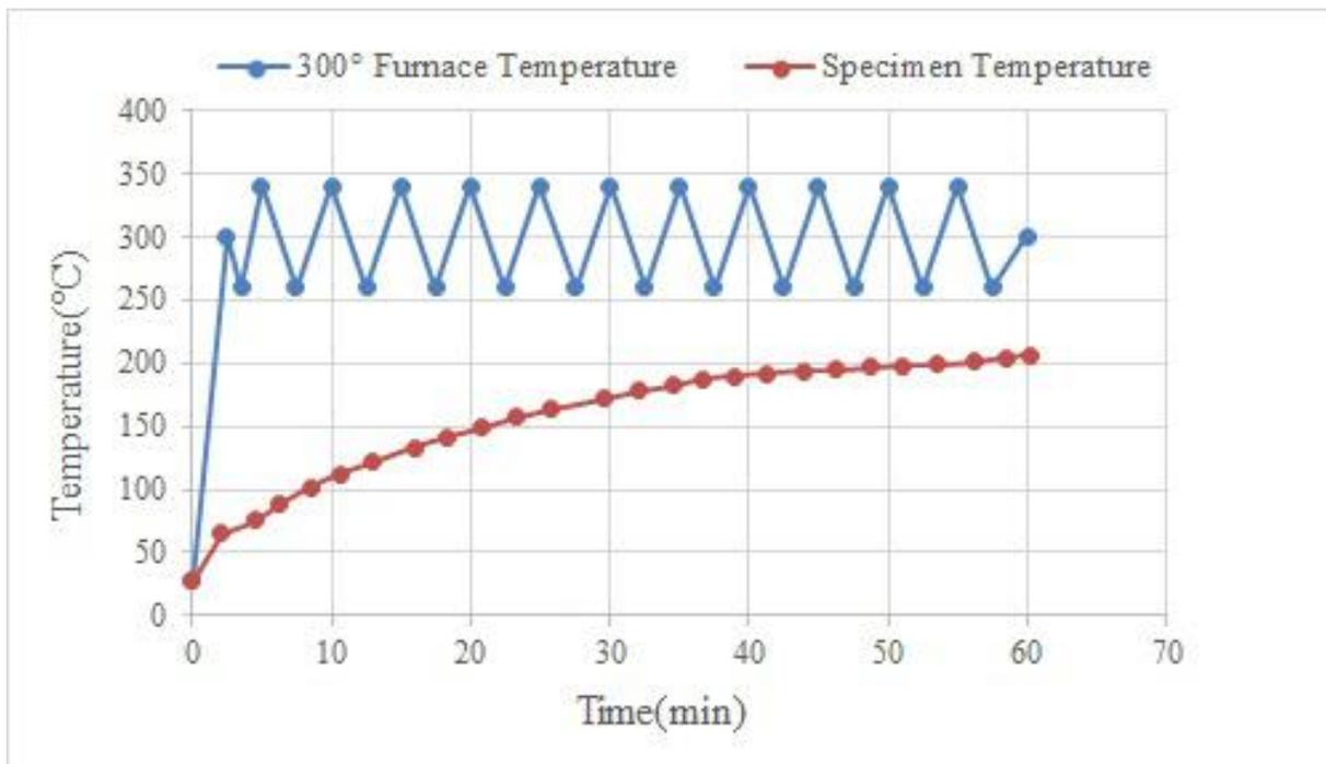
Figure 3.9: Rise in Specimens Temperature for 300°C Heating Regime
