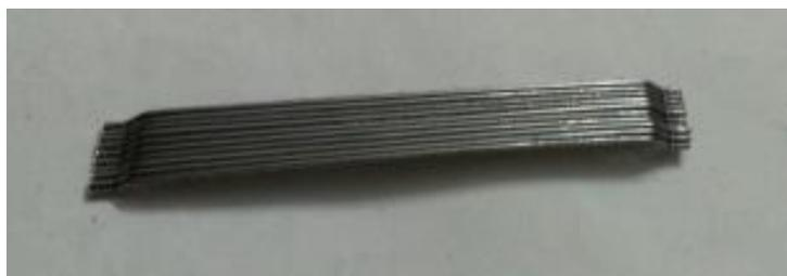
Figure 3.1: Close View of Steel Fibres
