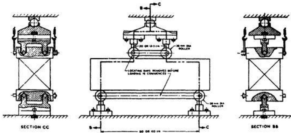
Figure 3.14: Flexure Test Setup
