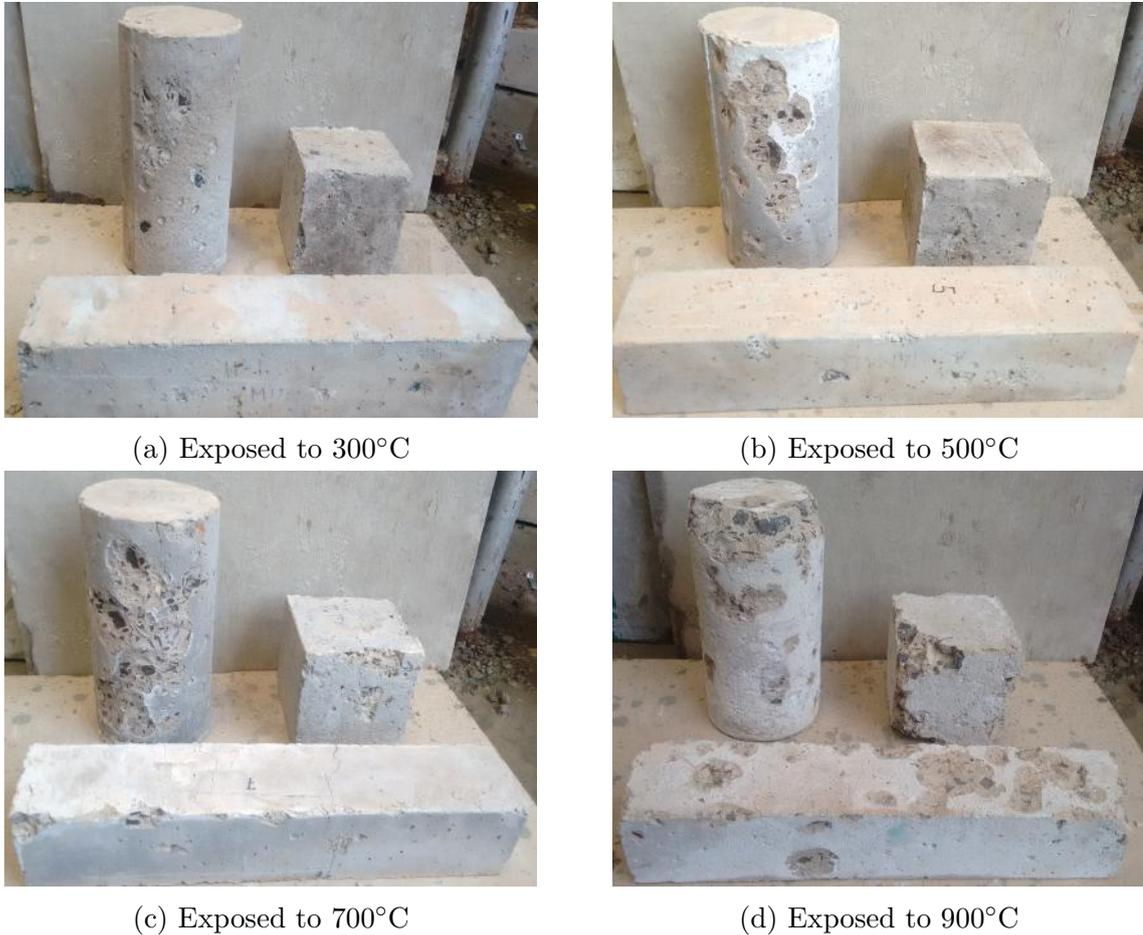
Figure 4.4: M60(PCC) Subjected to Different Elevated Temperatures
