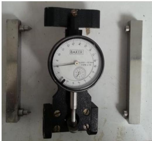
Figure 3.23: Mechanical Strain Gauge
