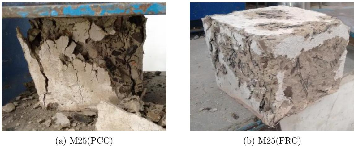
Figure 4.3: Compressive Failure Pattern M25(PCC) & M25(FRC) after Exposed to 900°C
