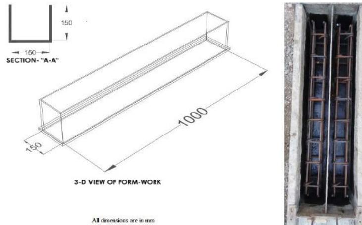
Figure 3.5: Steel Formwork with Reinforcement Cage
