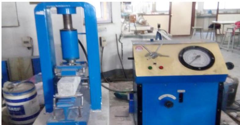
Figure 3.15: Plain Concrete Beam in Flexure Testing Machine
