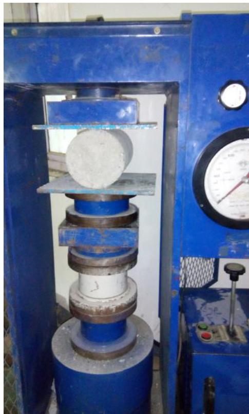
Figure 3.16: Test Setup for Split Tensile Strength of Concrete
