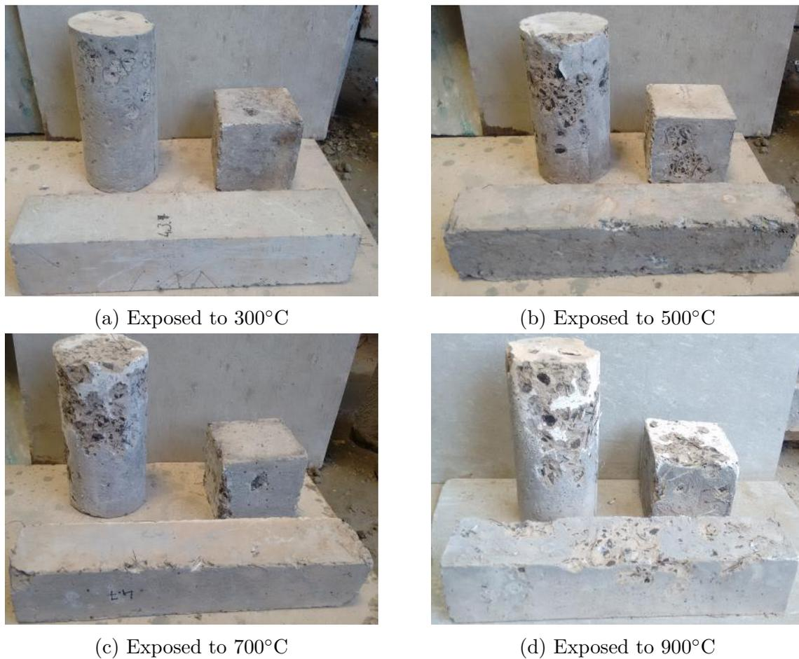
Figure 4.5: M60(FRC) Subjected to Different Elevated Temperatures
