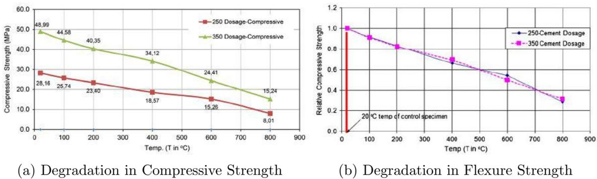
(a) Degradation in Compressive Strength
