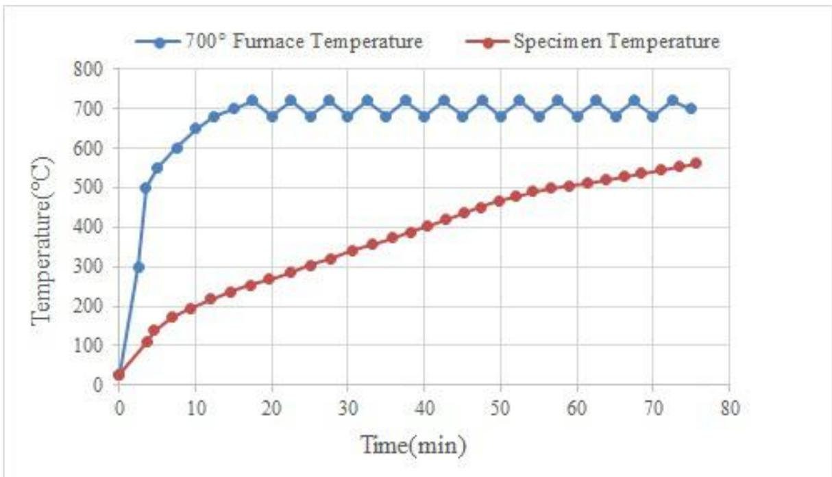
Figure 3.11: Rise in Specimens Temperature for 700°C Heating Regime
