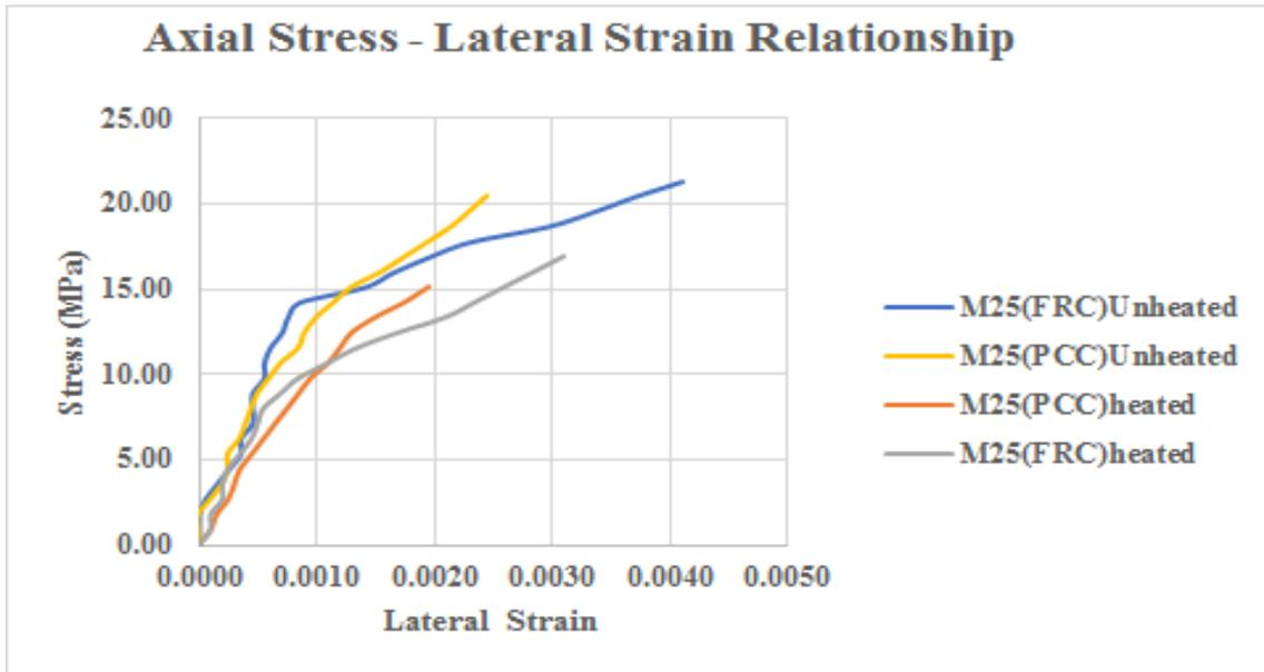
Figure 5.5: Axial Stress v/s Lateral Strain Relationship(M25)
