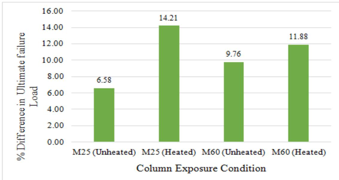
Figure 5.2: Percentage Difference in Ultimate Failure Load of FRC Column to that of Plain Concrete Column
