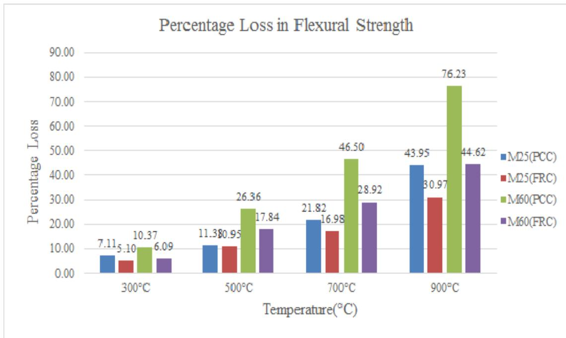
Figure 4.12: % Loss in Flexural Strength at Different Elevated Temperatures as Compared to Unheated Specimens
