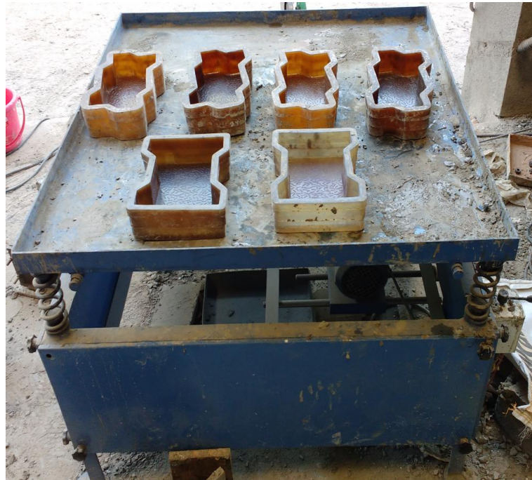
Figure 4.9: Table vibrator for compaction of specimen
