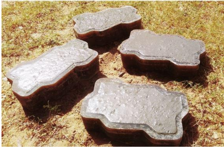
Figure 4.11: Setting of fresh alkali activated paver blocks
