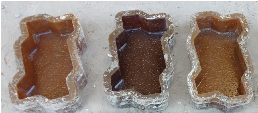
Figure 4.6: Preparation of rubber moulds
