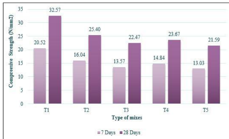
Figure 5.4: Compressive Strength of trial mixes
