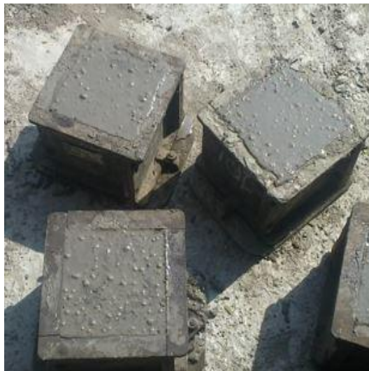
Figure 4.10: Setting of fresh alkali activated cubes
