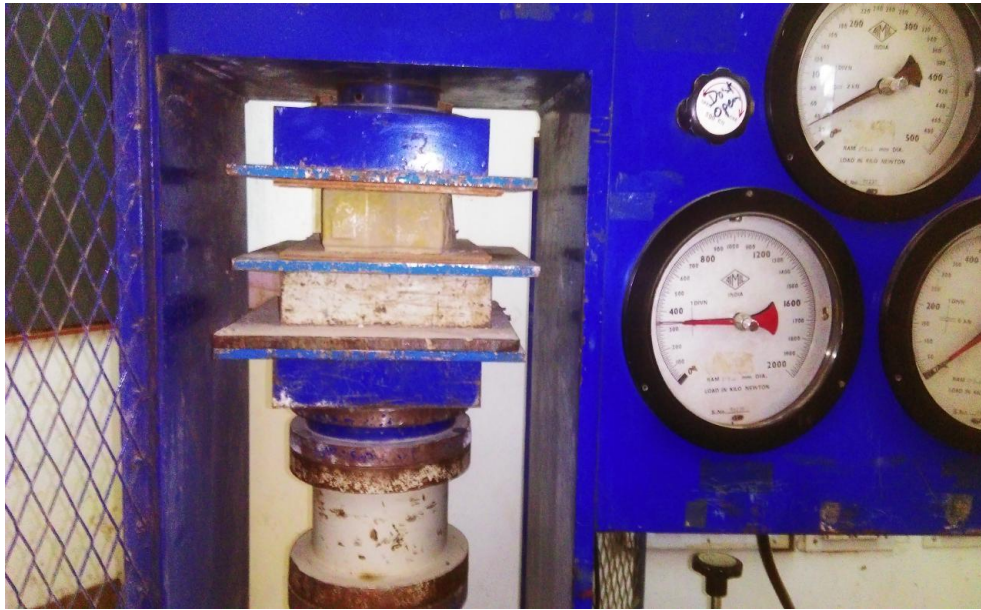
Figure 4.14: Paver block in Compression Testing Machine
