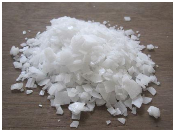
Figure 4.3: Sodium Hydroxide in Flakes
