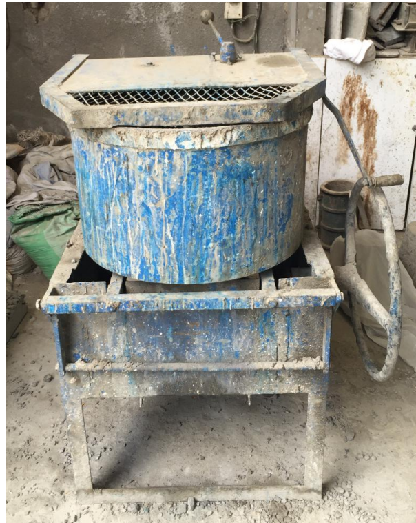
Figure 4.7: Pan mixture for casting of paver blocks
