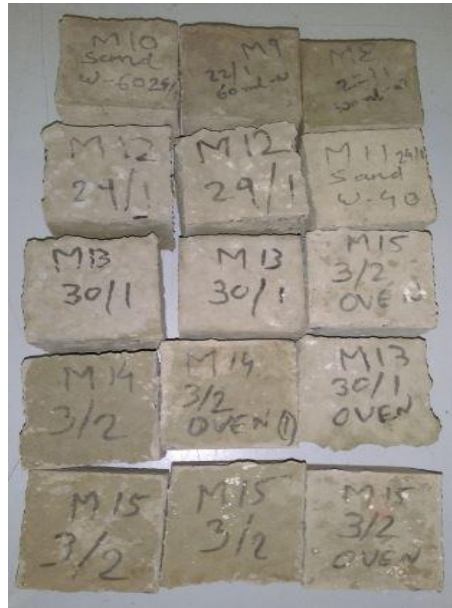
Figure 4.13: Ambient curing of alkali activated cubes
