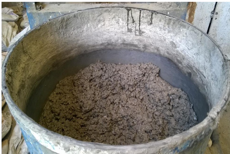
Figure 4.8: View of alkali activated binders
