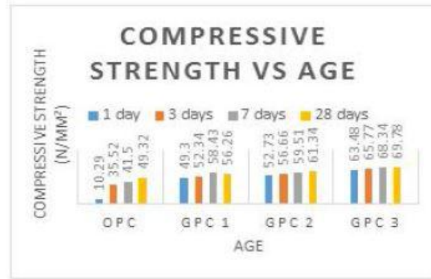
Figure 2.3: Compressive strength of paver blocks with respect to ages
