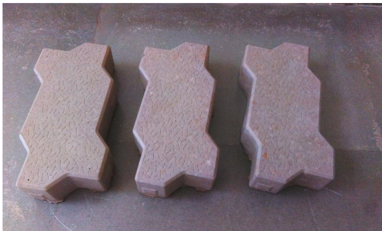
Figure 4.12: Ambient curing of alkali activated paver block
