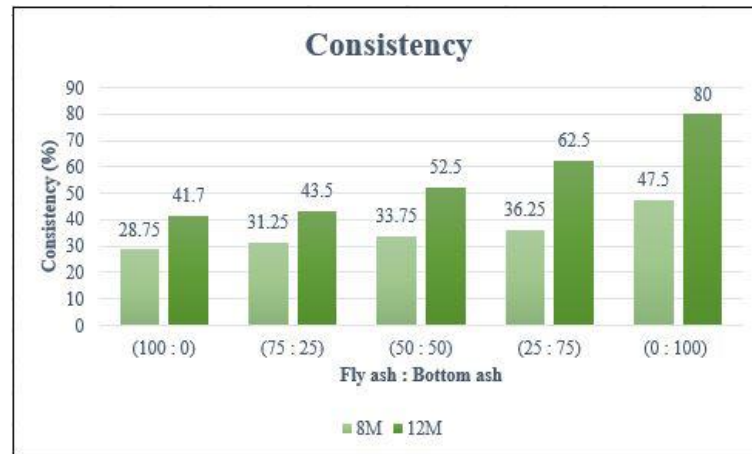
Figure 5.1: Consistency of alkali activated mortar
