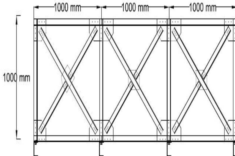
Figure 4.11: Elevation of Truss type Pedestrian bridge
