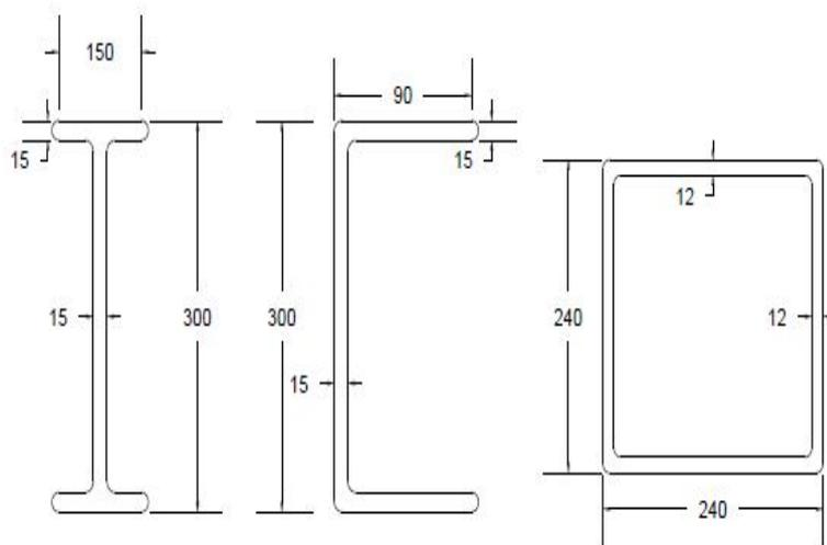
Figure 5.4: Sections Considered for 5m span Girder
