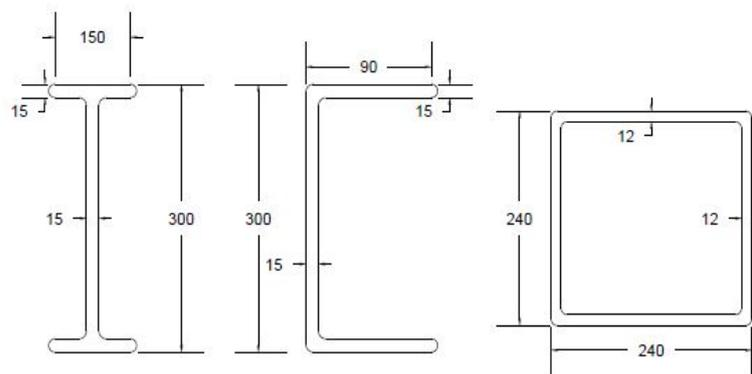
Figure 5.10: Sections Considered for 15m span Girder
