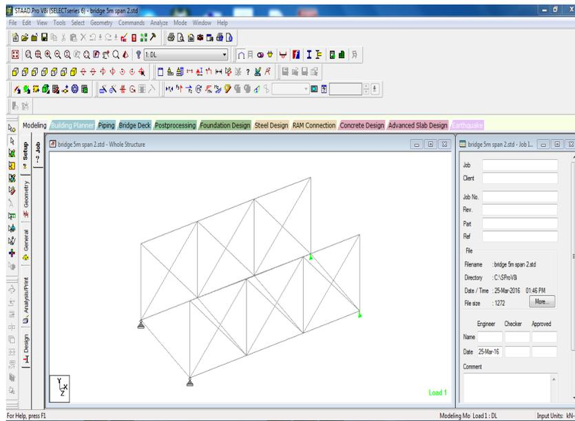
Figure 4.12: Staad model of truss type bridge
