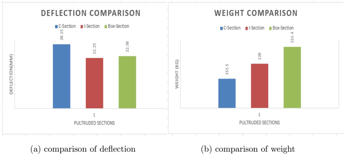
Figure 5.15: Comparison of deflection and weight for 20m span
