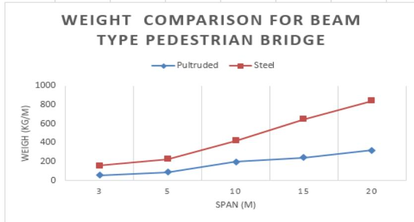
Figure 6.1: Weight Comparison for Beam Type Pedestrian Bridge
