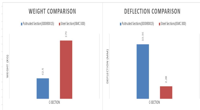
Figure 5.43: Comparison of weight and deflection for 3m span
