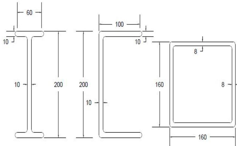
Figure 4.8: Sections Considered for 3m span Girder
