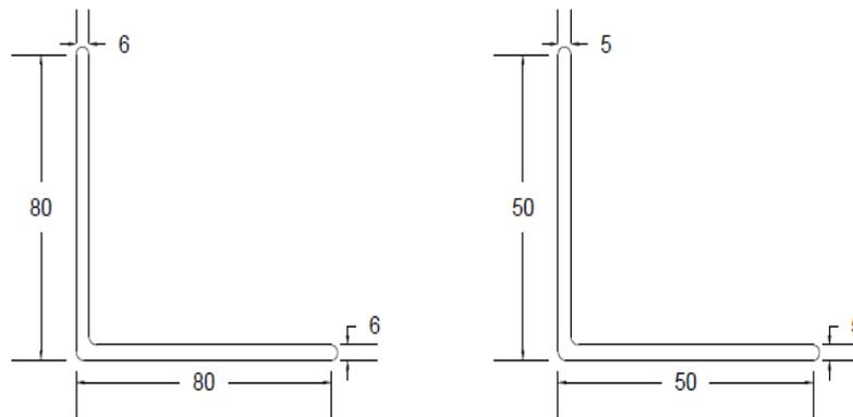
Figure 5.69: Sections used for 10m span girder
