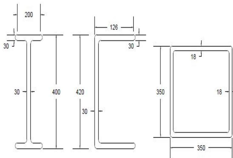
Figure 5.7: Sections Considered for 10m span Girder
