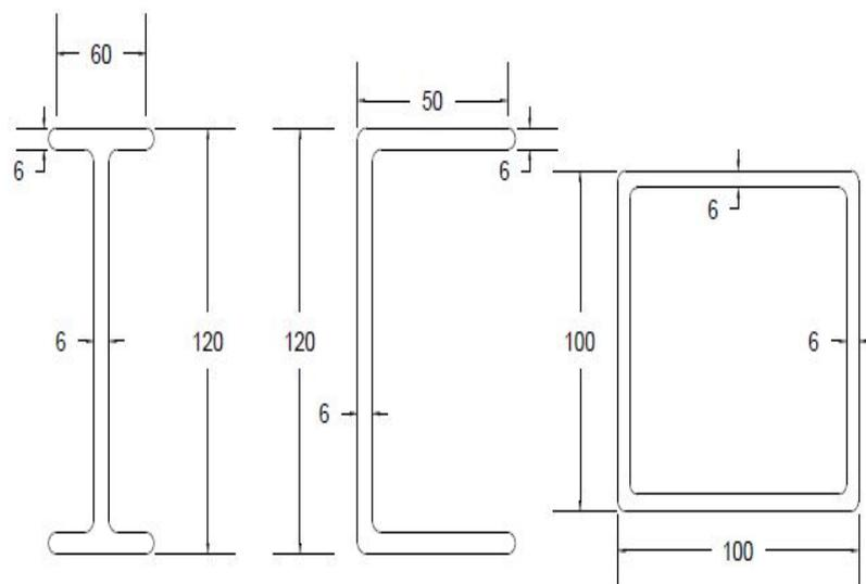
Figure 5.16: Sections Considered for 3m span Cross Girder
