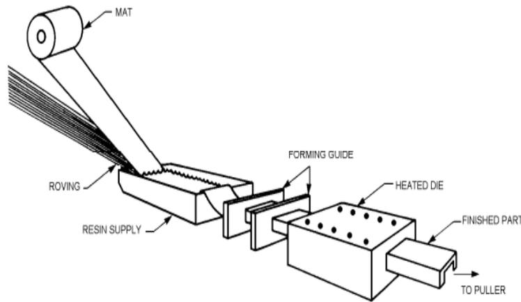
Figure 1.1: Pultrusion Process
