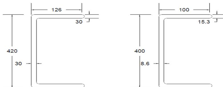
Figure 5.47: Sections used for 10m span girder
