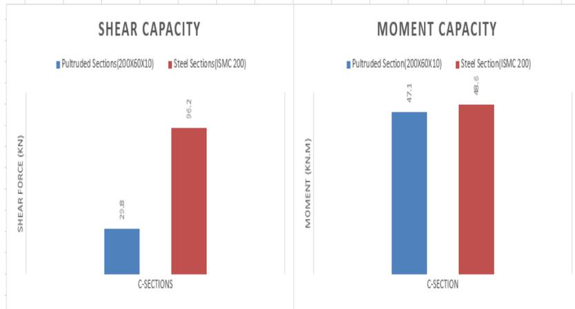
Figure 5.36: Comparison of Moment and Shear capacity for 3m span
