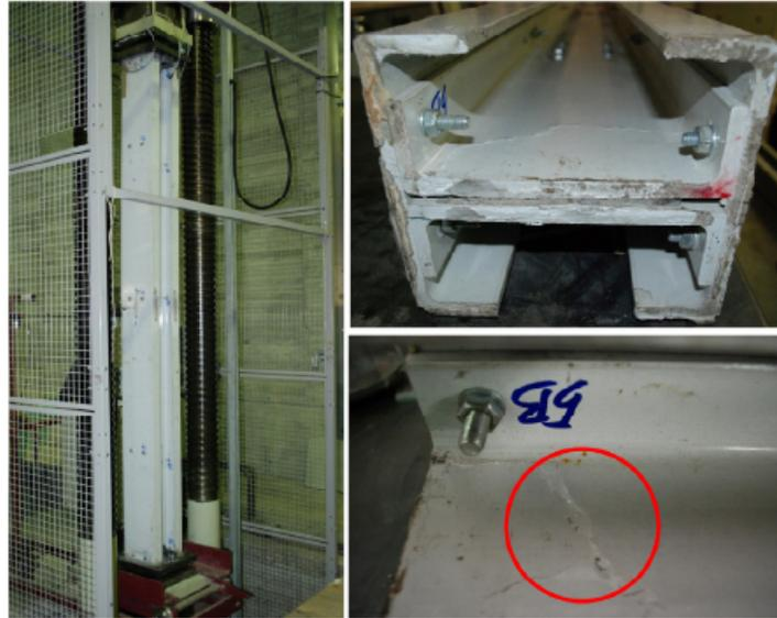
Figure 2.7: Collapse damage of column 200
