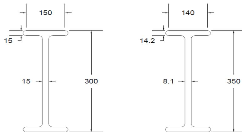
Figure 5.56: Sections used for 10m span girder
