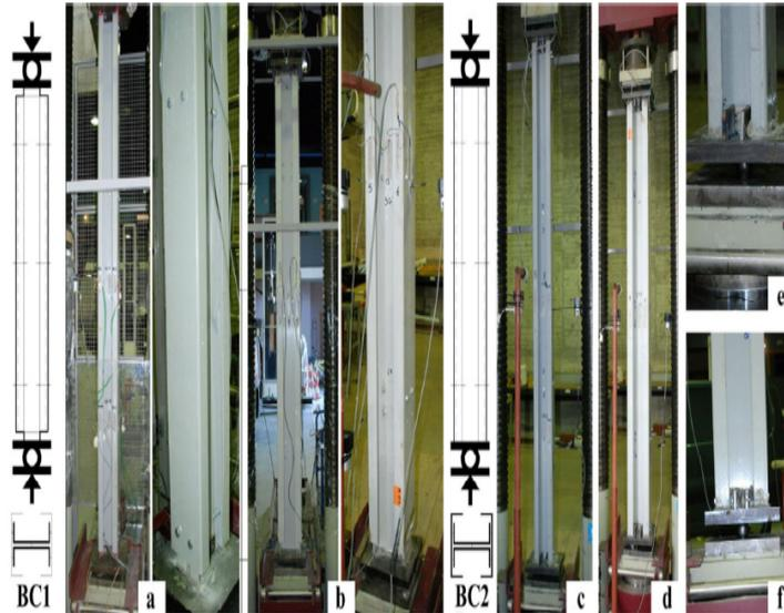
Figure 2.5: Test setup for build-up columns
