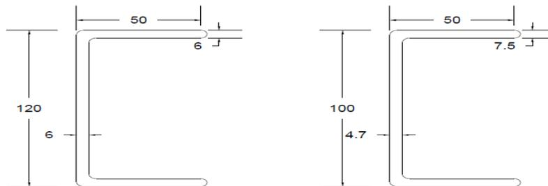
Figure 5.65: Sections considered for cross girder
