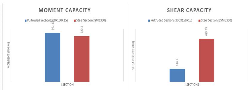
Figure 5.51: Comparison of Moment and Shear capacity for 3m span
