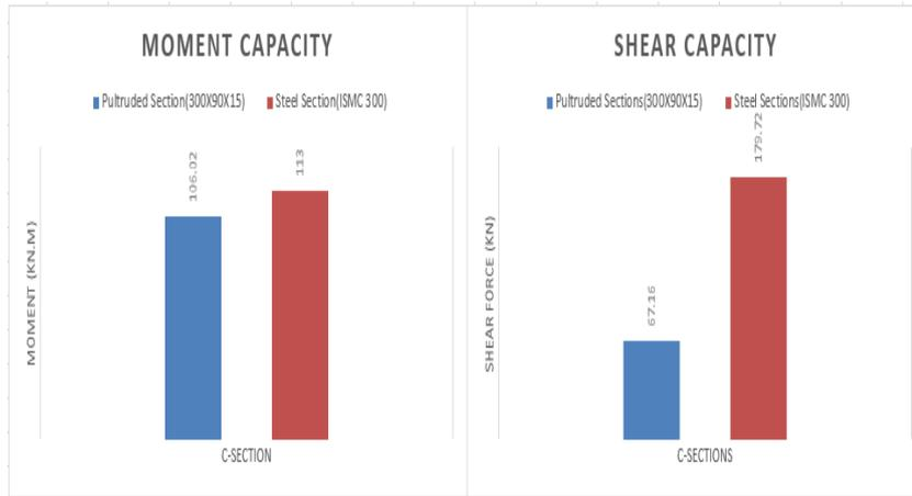
Figure 5.42: Comparison of Moment and Shear capacity for 3m span
