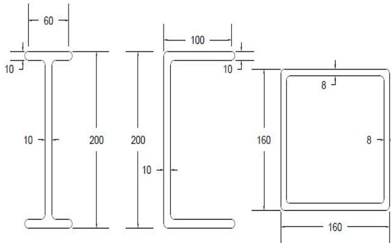
Figure 5.1: Sections Considered for 3m span Girder
