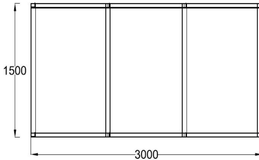
Figure 4.10: Plan of 3m span Truss Type Pedestrian Bridge
