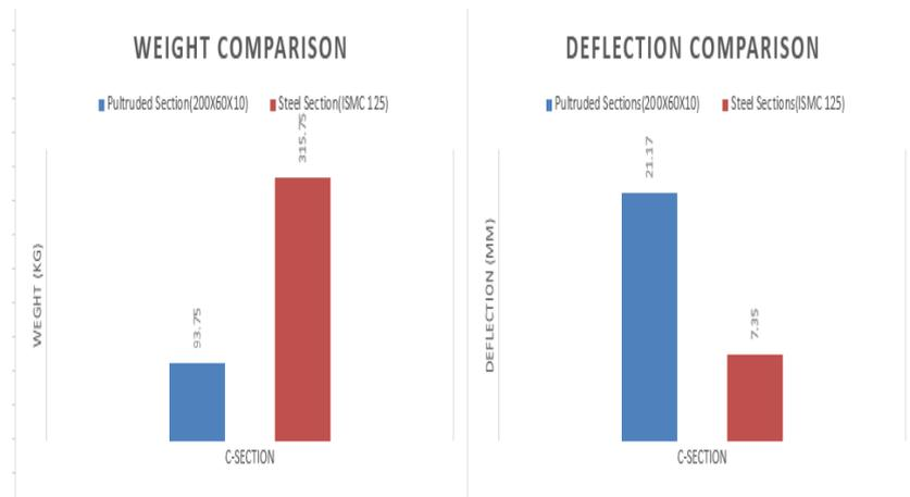
Figure 5.55: Comparison of weight and deflection for 3m span
