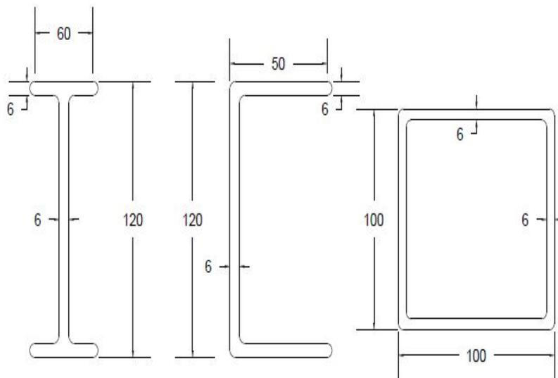
Figure 4.14: Sections Considered for 3m span Cross Girder
