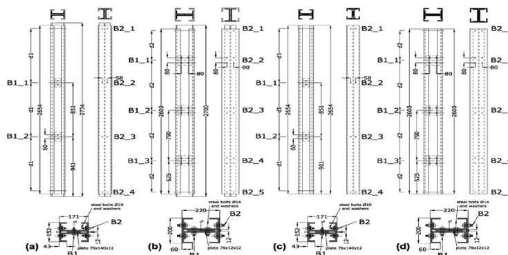
Figure 2.2: Different configurations for Build-up column
