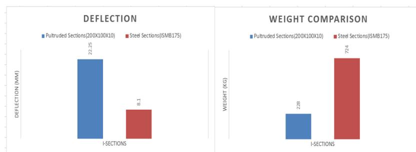
Figure 5.64: Comparison of weight and deflection for 3m span
