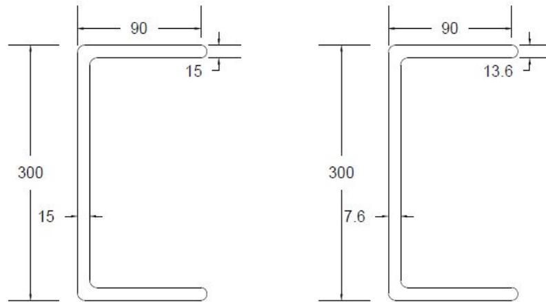
Figure 5.41: Sections used for 5m span girder
