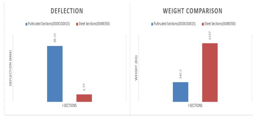
Figure 5.52: Comparison of weight and deflection for 3m span
