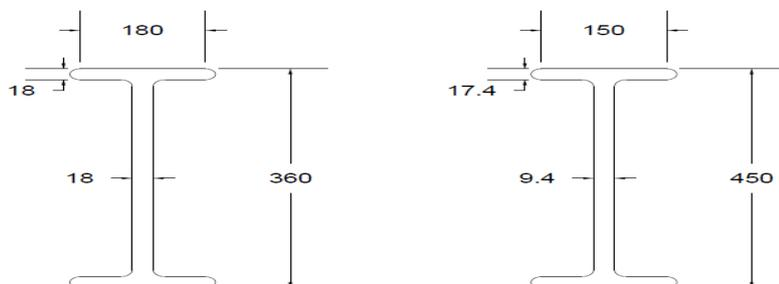
Figure 5.62: Sections used for 10m span girder
