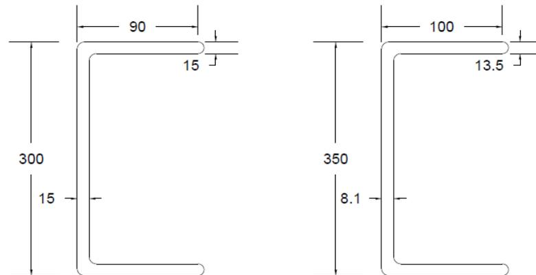
Figure 5.53: Sections used for 10m span girder
