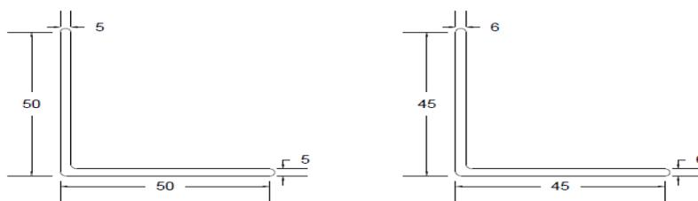
Figure 5.68: Sections used for 10m span girder
