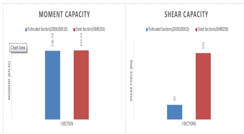
Figure 5.39: Comparison of Moment and Shear capacity for 3m span
