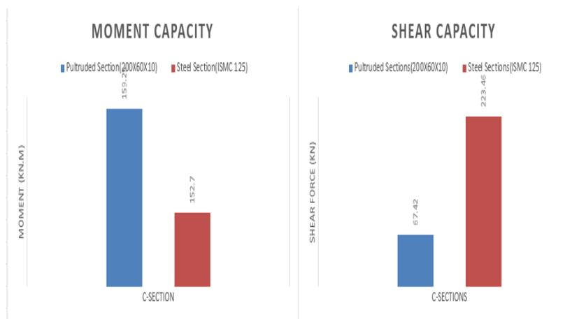
Figure 5.54: Comparison of Moment and Shear capacity for 3m span
