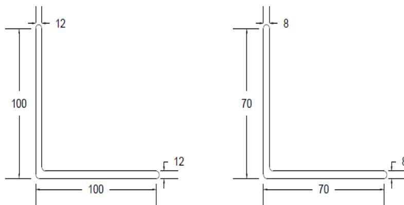
Figure 5.71: Sections used for 10m span girder
