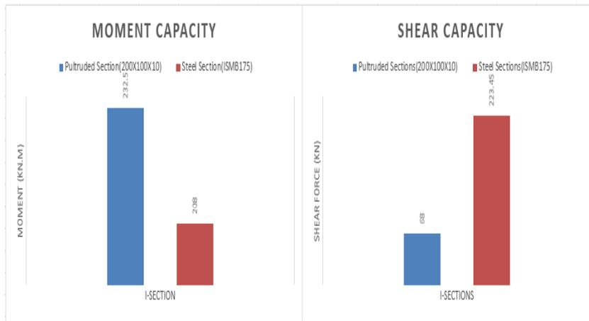
Figure 5.57: Comparison of Moment and Shear capacity for 3m span
