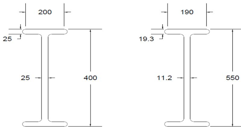
Figure 5.50: Sections used for 10m span girder
