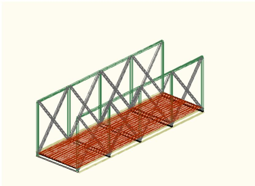
Figure 4.9: Truss type Pedestrian Bridge
