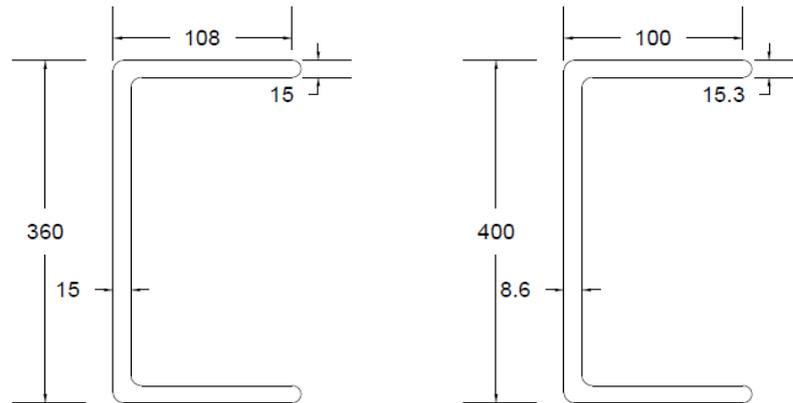
Figure 5.59: Sections used for 10m span girder
