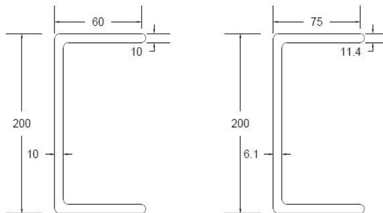
Figure 5.35: Sections used for 3m span girder
