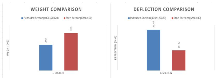
Figure 5.49: Comparison of weight and deflection for 3m span
