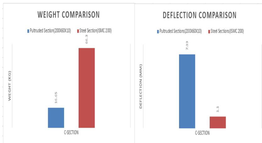
Figure 5.37: Comparison of weight and deflection for 3m span
