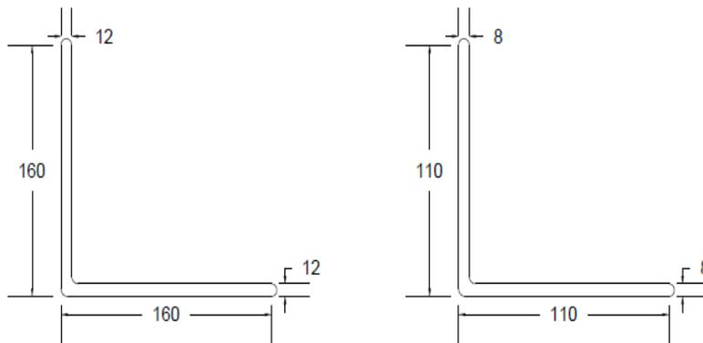
Figure 5.72: Sections used for 10m span girder
