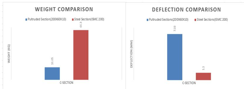
Figure 5.58: Comparison of weight and deflection for 3m span
