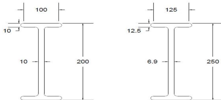
Figure 5.38: Sections used for 3m span girder
