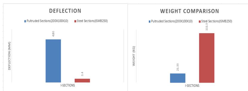
Figure 5.40: Comparison of weight and deflection for 3m span
