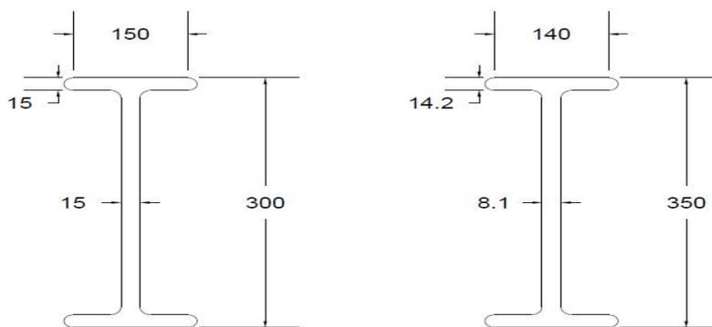
Figure 5.44: Sections used for 5m span girder
