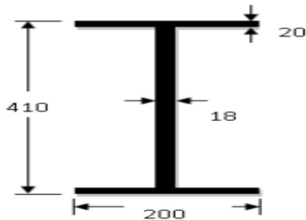
Figure 2.9: Section Used for Girders
