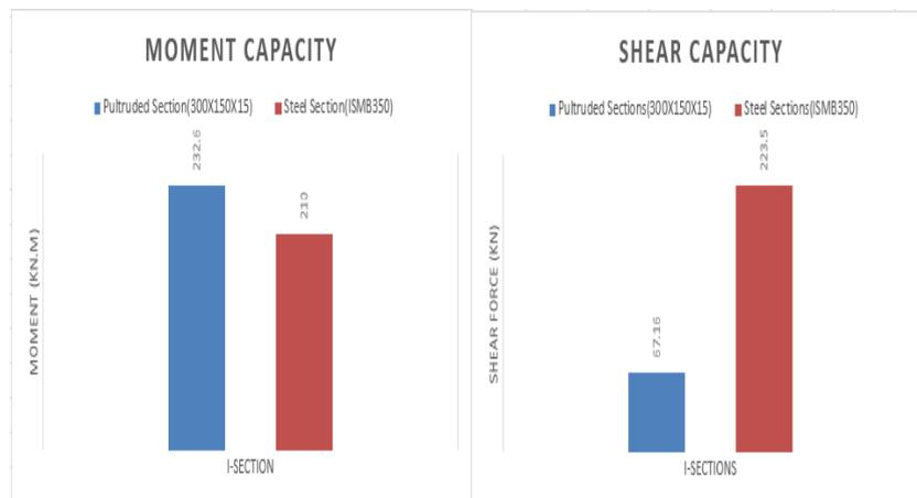
Figure 5.45: Comparison of Moment and Shear capacity for 3m span
