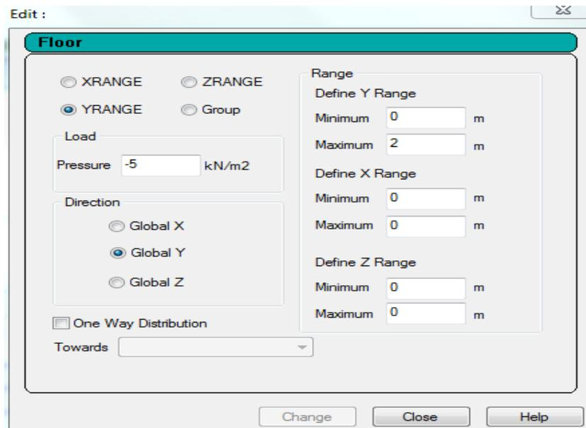
Figure 4.7: Live load of  $5 \text{ kN/m}^2$
