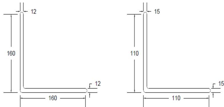
Figure 5.73: Sections used for 10m span girder
