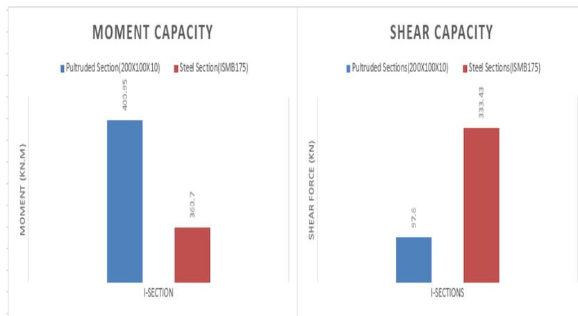
Figure 5.63: Comparison of Moment and Shear capacity for 3m span
