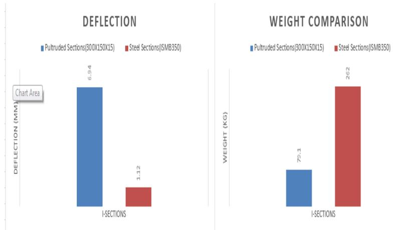
Figure 5.46: Comparison of weight and deflection for 3m span
