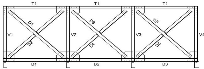
Figure 4.13: Member mark of 3m span bridge
