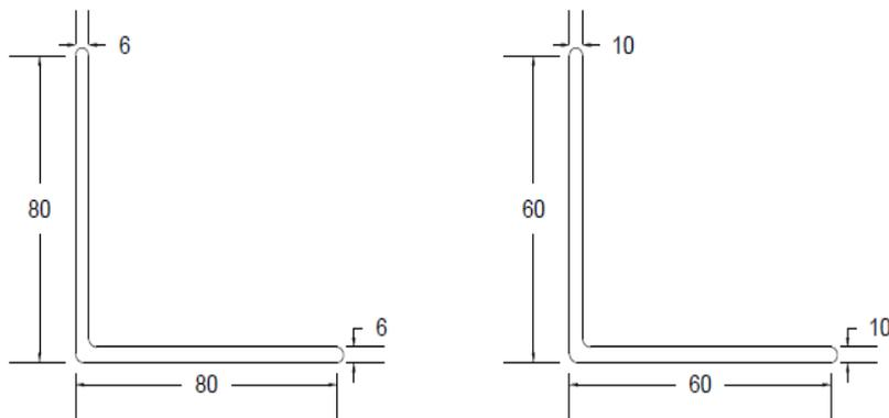
Figure 5.70: Sections used for 10m span girder
