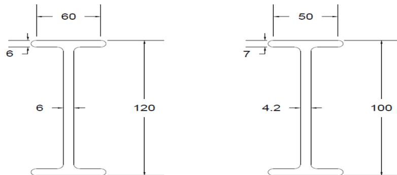
Figure 5.66: Sections considered for cross girder
