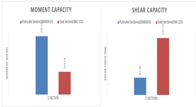
Figure 5.60: Comparison of Moment and Shear capacity for 3m span
