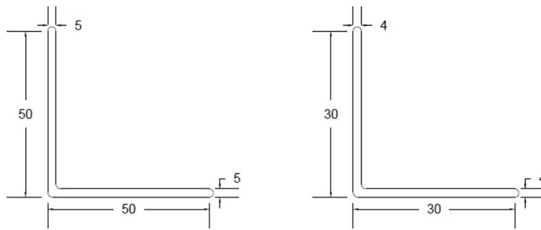
Figure 5.67: Sections used for 10m span girder
