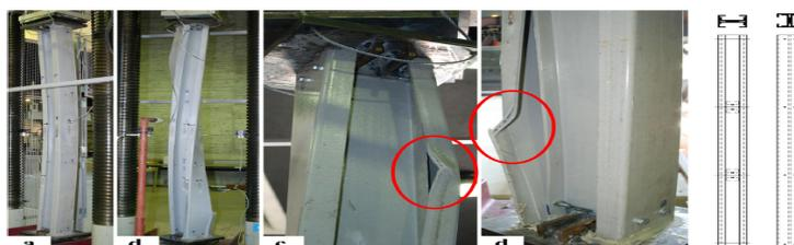
Figure 2.6: Collapse damage of column 152
