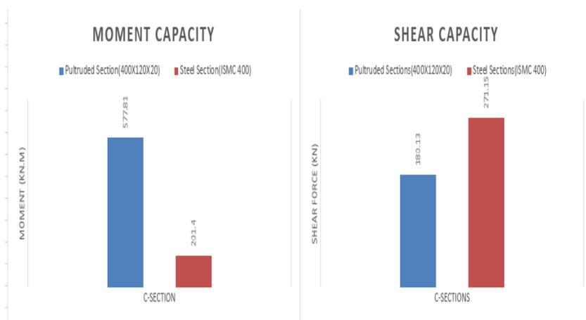
Figure 5.48: Comparison of Moment and Shear capacity for 3m span
