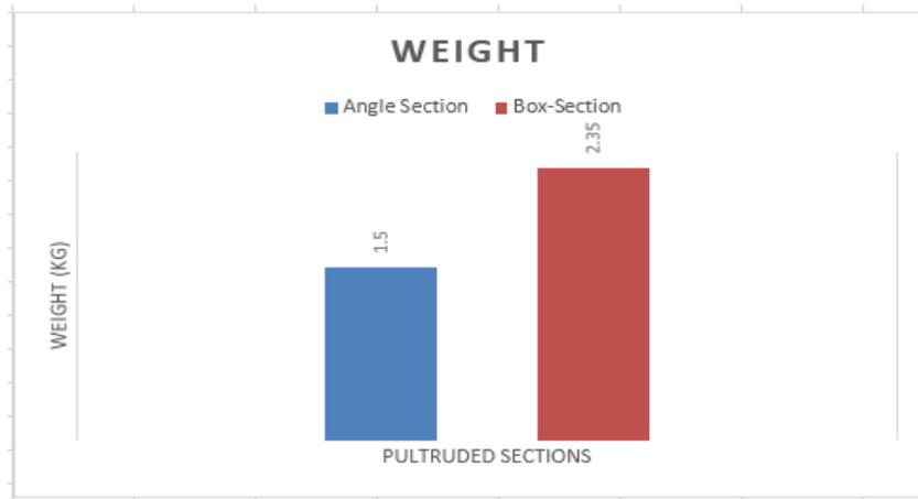
Figure 5.22: Comparison of weight for Diagonal Member
