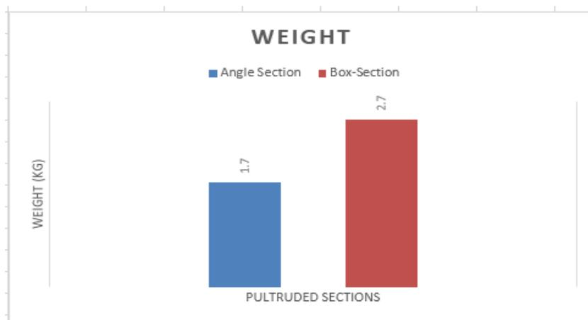
Figure 5.26: Comparison of weight for 10m span
