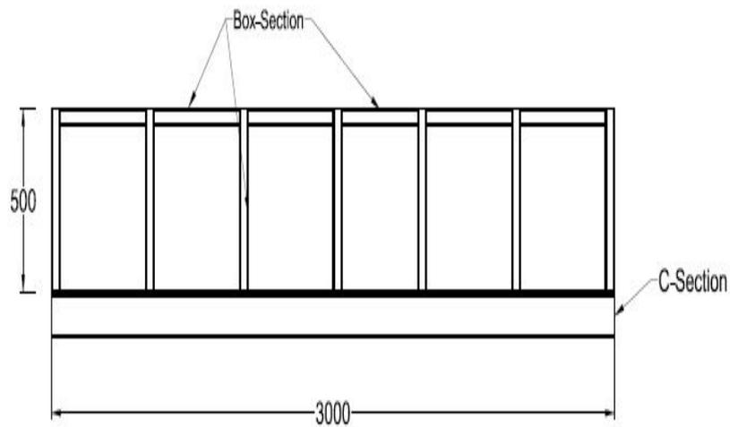
Figure 4.3: Elevation of 3m span beam type pedestrian bridge
