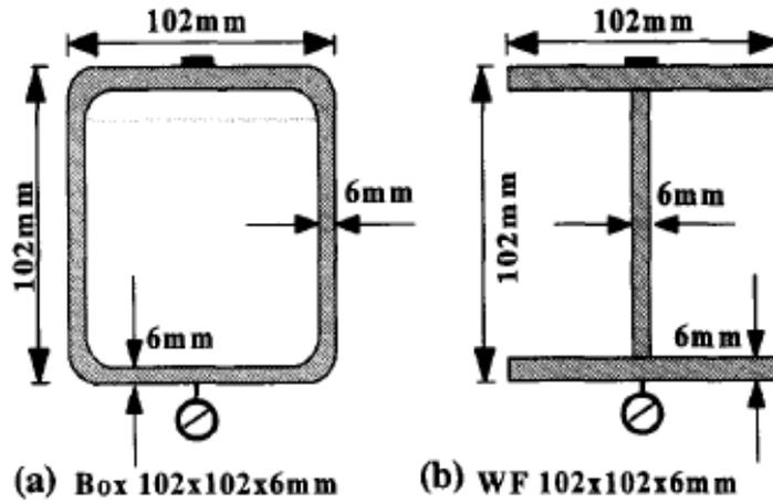
Figure 2.1: GFRP sections
