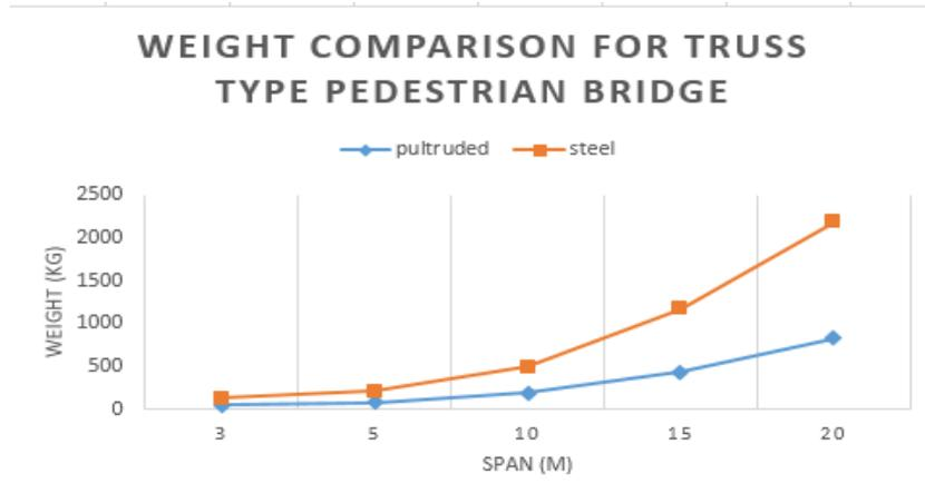
Figure 6.3: Weight Comparison for Truss Type Pedestrian Bridge
