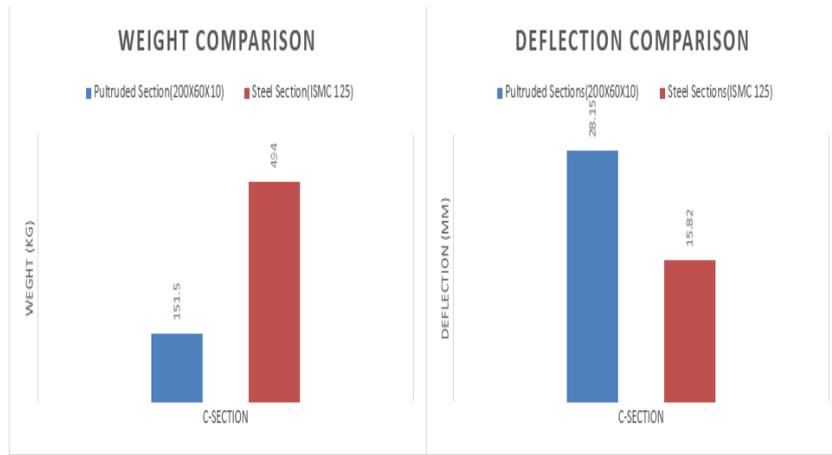
Figure 5.61: Comparison of weight and deflection for 3m span
