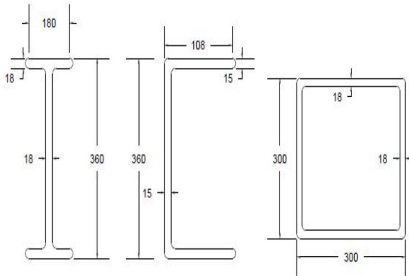
Figure 5.13: Sections Considered for 20m span Girder
