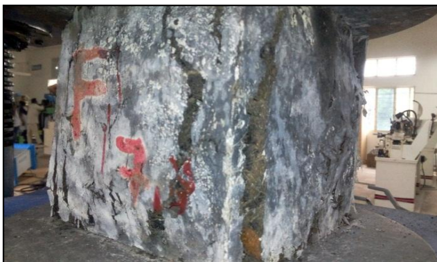
Fig. 3.2 (C) Cube specimen BFRC showing bridging of cracks by fiber
