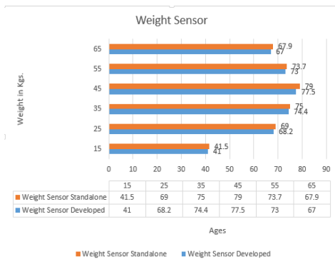
Fig. 13. Weight Sensor data for sensor developed vs. actual sensor
