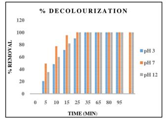
Fig. 3 Effect of pH on % color removal
