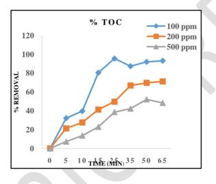
Fig. 8Effect of Dye Concentration on % TOC Removal
