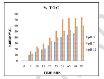
Fig. 4 Effect of pH on % TOC removal
