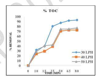
Fig.10 Effect of Ozone Flow rate on % TOC Removal
