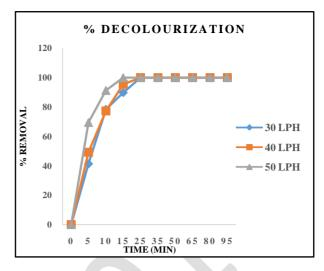
Fig. 9 Effect of Ozone Flow rate on % Decolourization
