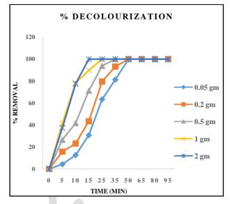
Fig. 5 Effect of Catalyst Dosage on % Color Removal
