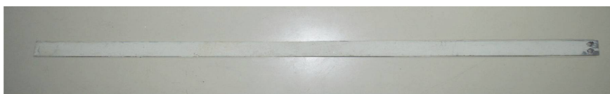
Figure 4. SP-5 A Coated aluminum cantilever beam.
