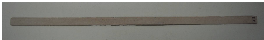
Figure 3. SP-4 Coated aluminum cantilever beam.
