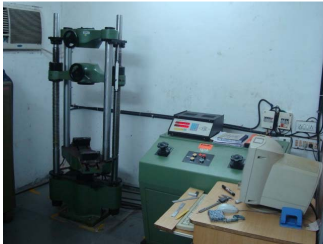
Fig 6.11 Experimental Set up for Tensile Test
