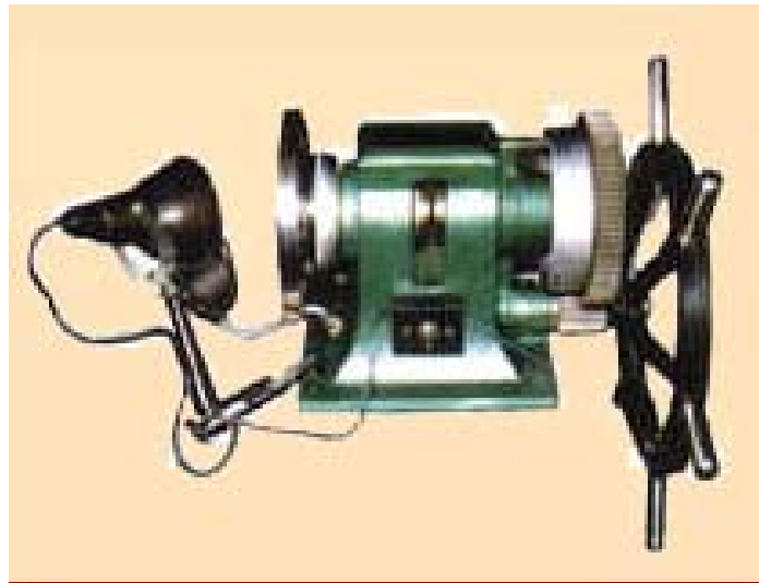
Fig .6.6 Experimental Set Up for Erichson test
