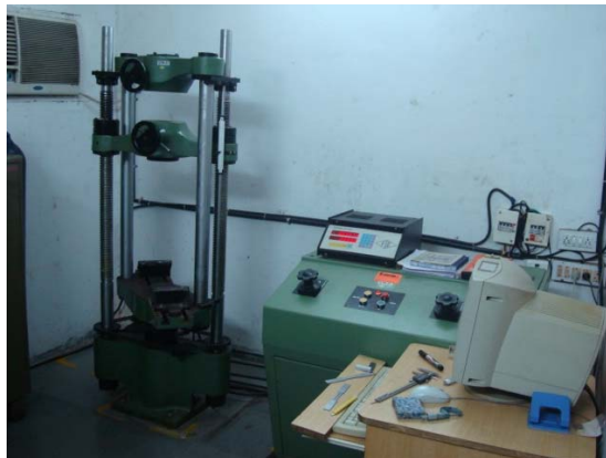
Fig 3.1 Experimental Set up for Uniaxial Tensile Test
