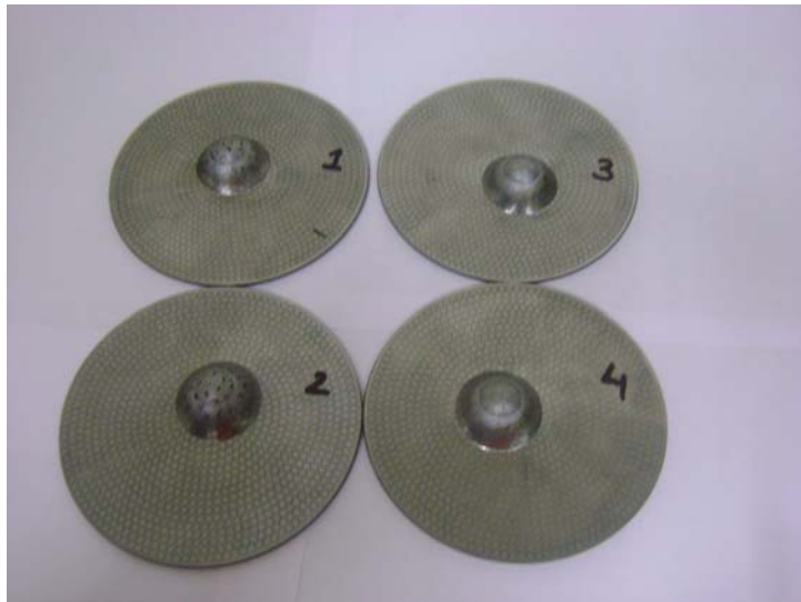
Fig 6.8 Deformed Specimen of Erichson Test
