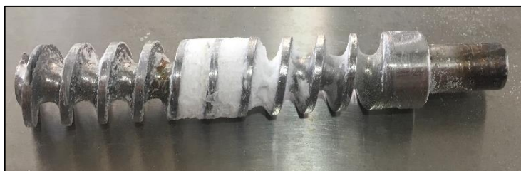
Fig. 1.2(b): Solid polymer blocking the channel in the HME screw
