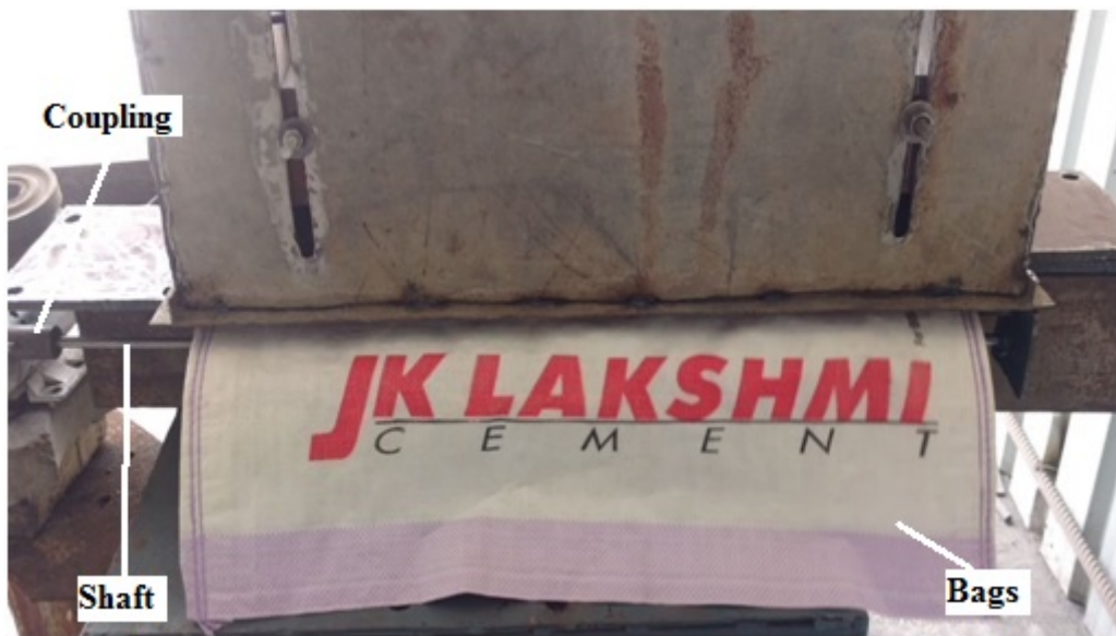
Figure 4.6: Phase - II testing of testing of fabricated structure of modified bucket mechanism-II [ Courtesy: JK Lakshmi Cement Ltd. ]
