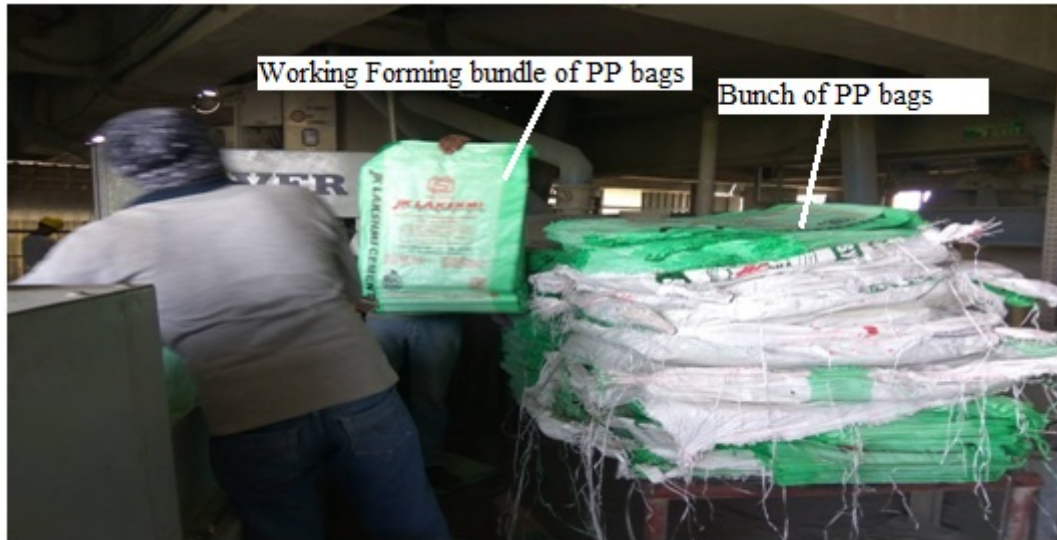
Figure 1.5: Manual filling of bags [ Courtesy: JK Lakshmi Cement ]
