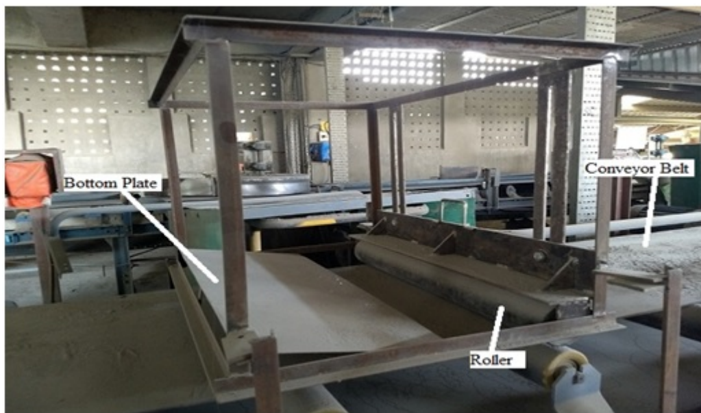
Figure 4.4: Phase - I testing of fabricated structure of modified bucket mechanism-I [ Courtesy: JK Lakshmi Cement Ltd. ]
