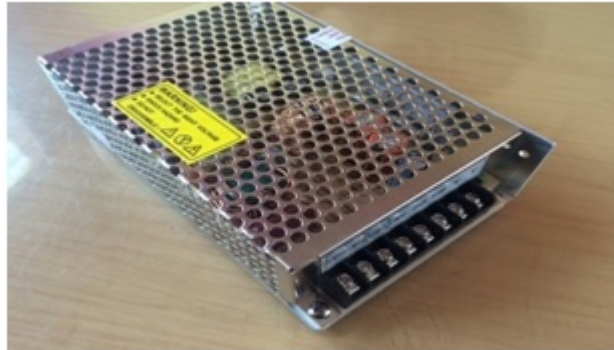
Figure 3.12: 12V DC SMPS
