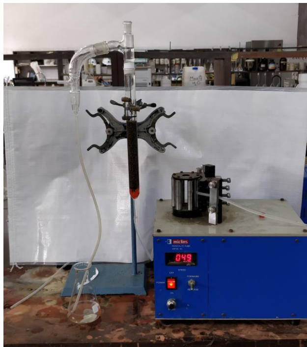
Figure 3 Experimental set-up for column adsorption study
