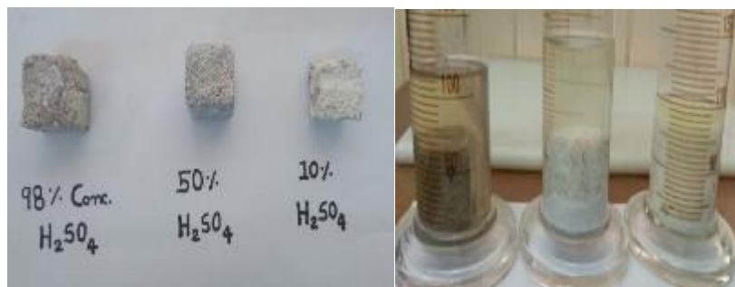
Figure 26 Portland cement Concrete after immersion
