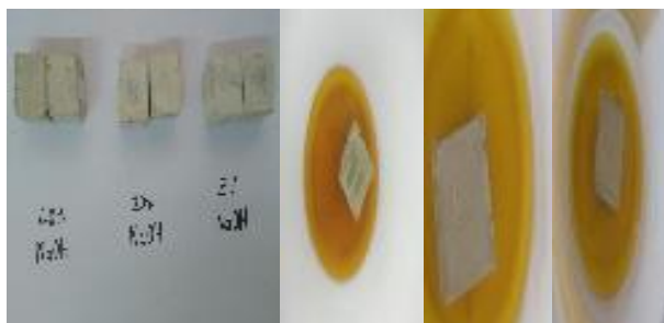
Figure 39 SPC Trans, trans-1,4 Diphenyl-1,3-Butadiene sulfur blocks after immersion in alkaline medium
