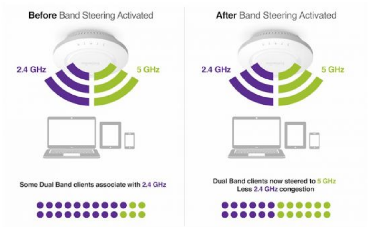
Figure 3.11: Reduce Wi-Fi Congestion With Band Steering[10]
