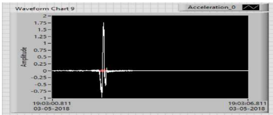
Figure 7.30: Acceleration Response of SDOF system with T Planar asymmetry with Double Pneumatic Damper
