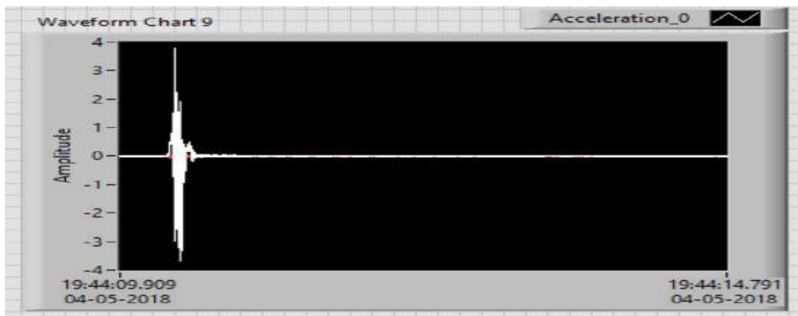
Figure 7.14: Acceleration Response of SDOF system with material Irregularity with Double Pneumatic Damper
