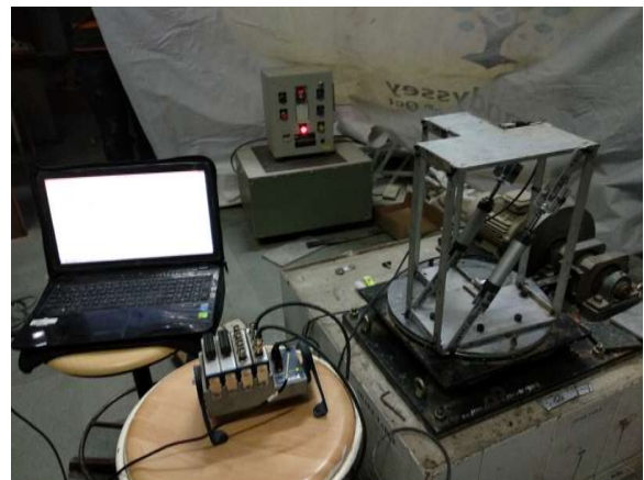
(b) Experimental setup of SDOF building model with Planar Asymmetry T Shape having double Pneumatic Damper
