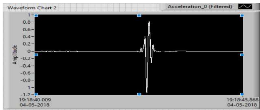
Figure 7.11: Extracted Acceleration Response of SDOF system with material Irregularity with single Pneumatic Damper
