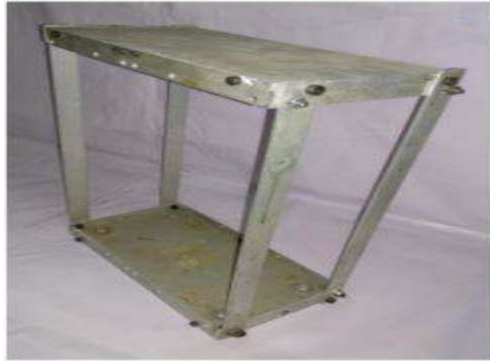
Figure 5.3: Photograph of SDOF model
