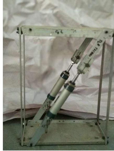
(b) Experimental setup of SDOF building model with material irregularity having double Pneumatic Damper
