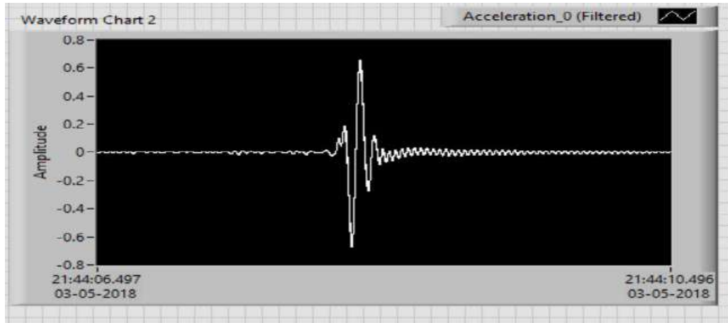
Figure 7.19: Extracted Acceleration Response of SDOF system with L Planar Asymmetry with single Pneumatic Damper
