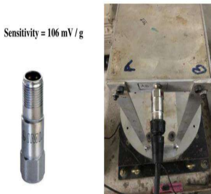
Figure 4.3: IMI Accelerometer attached to the Mass of SDOF System
