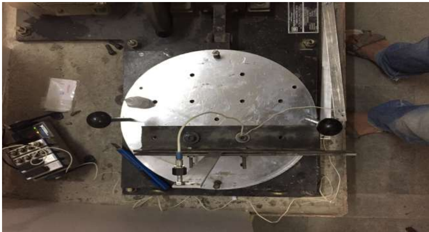
Figure 5.6: Uni-axial Accelerometer attached to aluminum column strip
