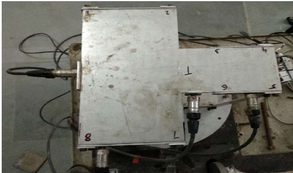
Figure 5.48: Experimental Setup of Building model having planar irregularity T-Shape
