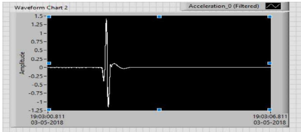
Figure 7.31: Extracted Acceleration Response of SDOF system with T Planar asymmetry with Double Pneumatic Damper
