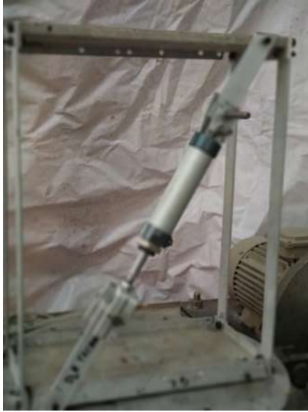
(a) Experimental setup of SDOF building model with material irregularity having single Pneumatic Damper
