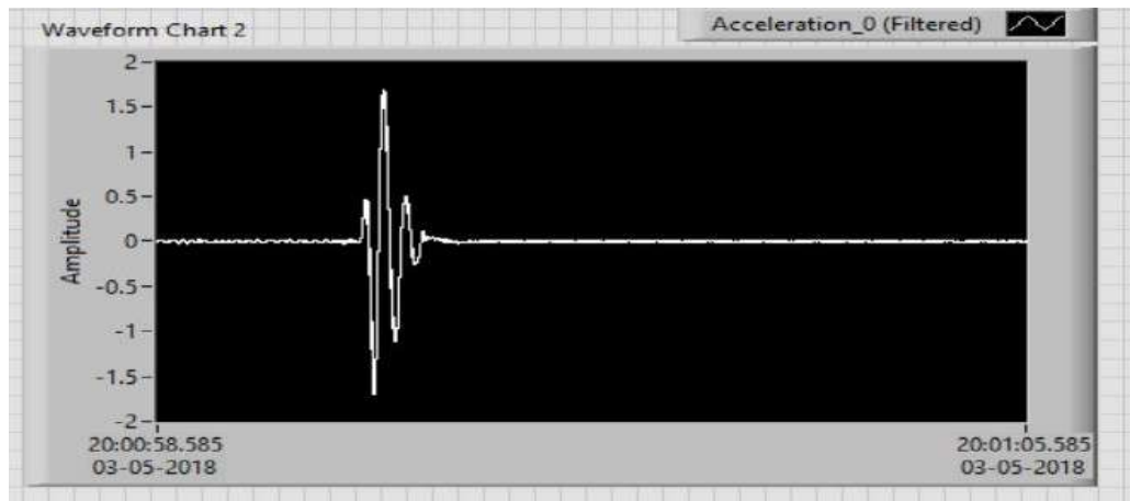
Figure 7.27: Extracted Acceleration Response of SDOF system with T Planar Asymmetry with single Pneumatic Damper
