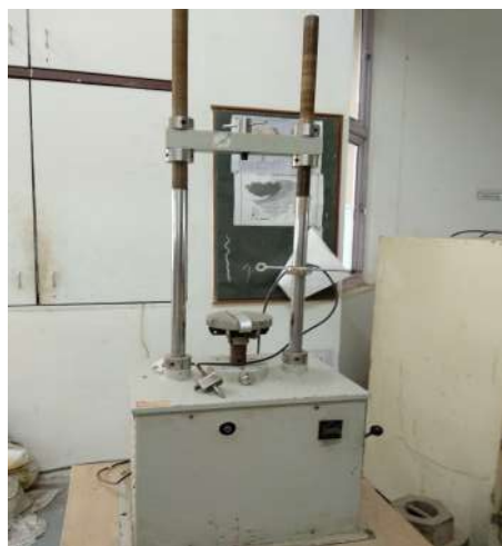
Figure 4.9: Unconfined Compression Testing Machine
