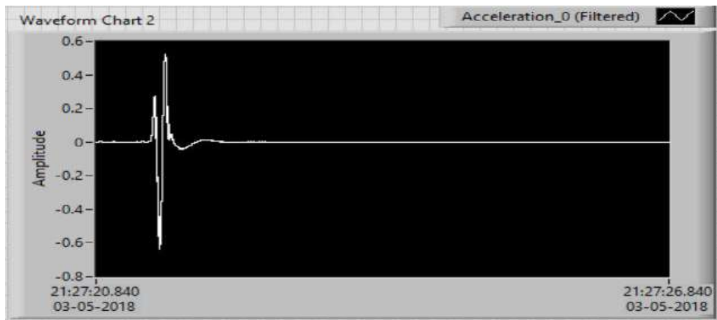
Figure 7.23: Extracted Acceleration Response of SDOF system with L Planar asymmetry with Double Pneumatic Damper
