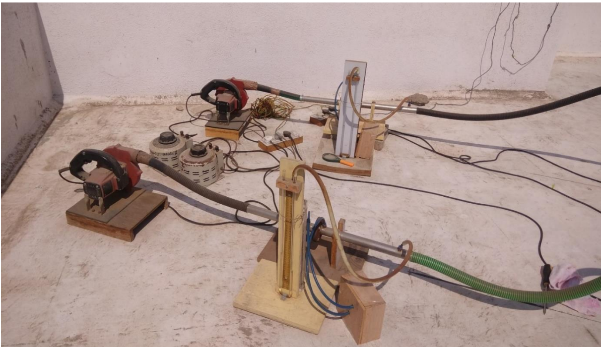
Fig 5.6 Photograph of experimental set up (arrangement of air flow circulation and measurement)
