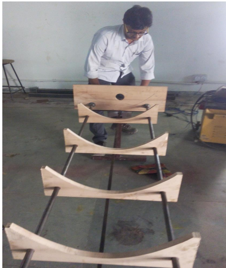
Fig 5.4 Fabrication work of solar collector structure
