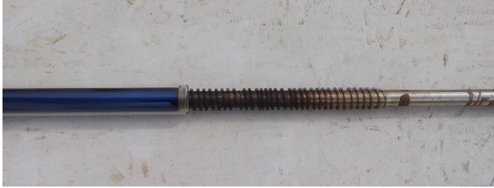
Fig 5.3 ETC with turbulator and air tube
