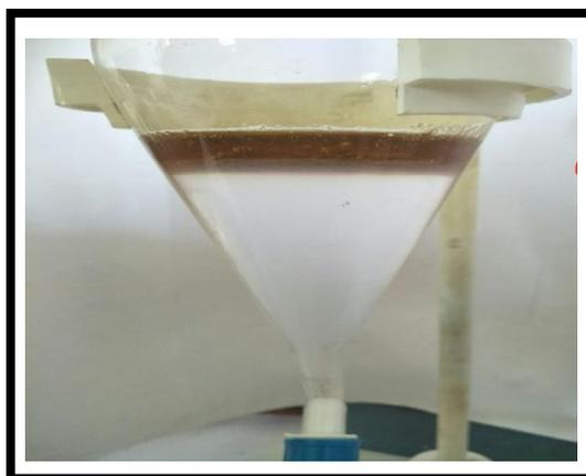
Figure 18: Extraction of crude oil with the help of hexane
