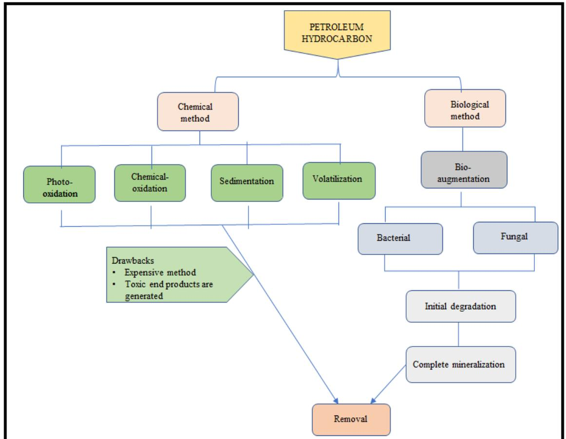
Figure 5: Methods of PAH degradation
