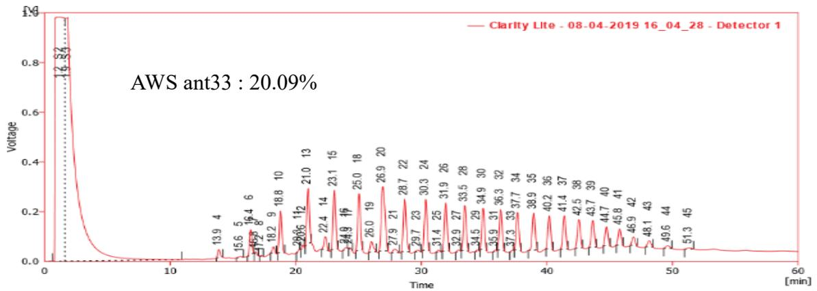
(b) Chromatogram of crude oil treated with AWS ant33
