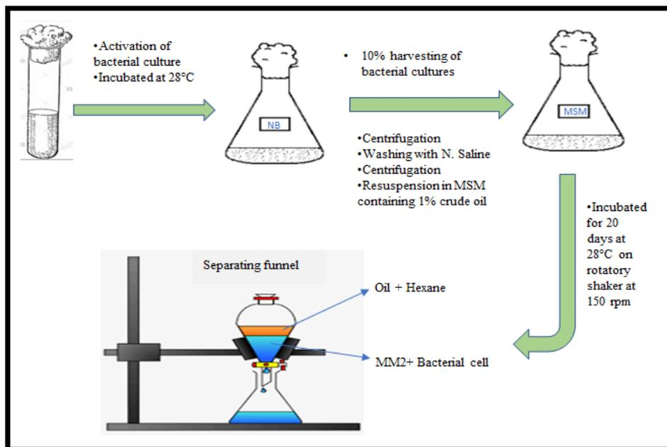
Figure 11: Crude oil biodegradation assay and its extraction process
