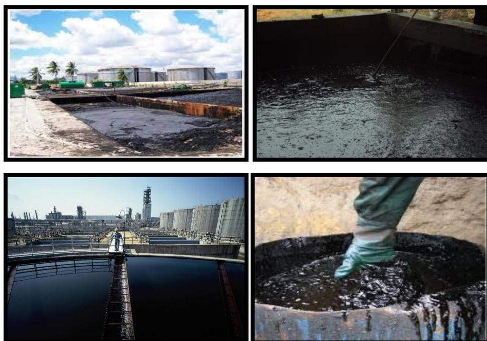
Figure 2: Petroleum oil sludge generated from petrochemical industries
