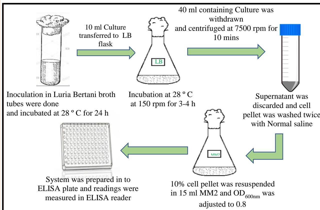
Figure 10: DCPIP assay to rapidly screen hydrocarbon degrading bacteria
