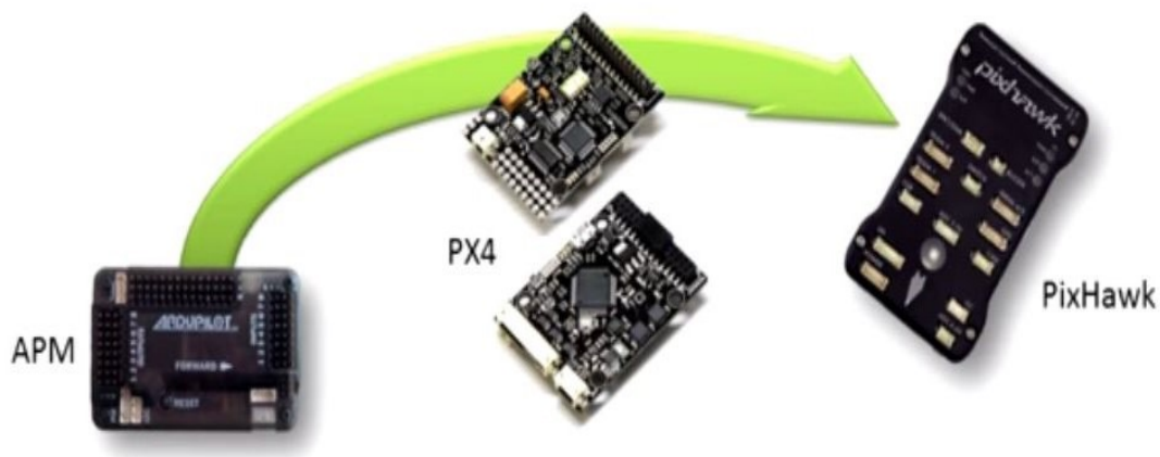
Figure 3.1: Evolution of Pixhawk from APM
