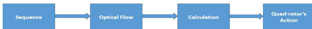
Figure 6.1: Block level design of obstacle avoidance algorithm using optical flow for quadrotors
