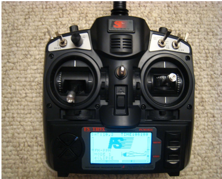
Figure 3.7: Flysky TH 9X 9 CH TX + 8CH RX, High Range, Fully Programmable Radio Transmitter and Receiver
