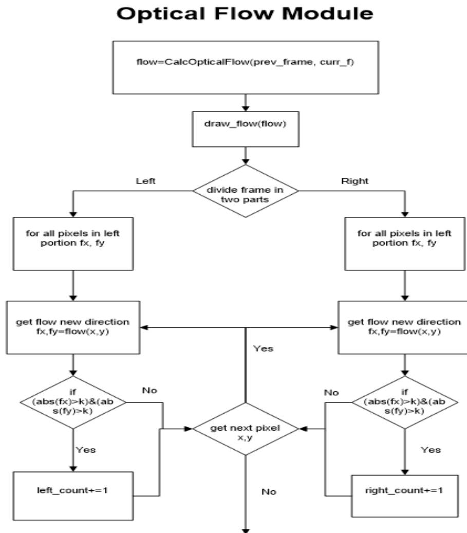
Figure 6.4: Block level design of obstacle avoidance algorithm using optical flow for quadrotors
