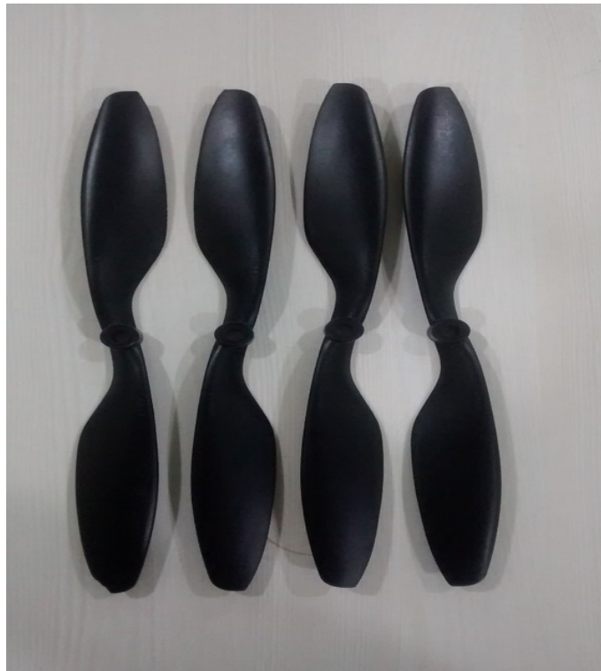
Figure 3.2: Counter Rotating Propeller 1045/1045R for Quadrotor
