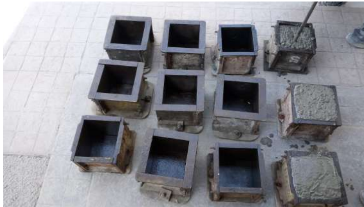
Figure 3.4: Pouring and Compaction of Concrete
