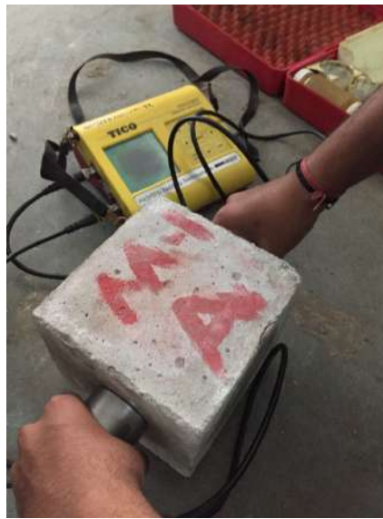
Figure 3.8: Taking Velocity of Cubes By UPV
