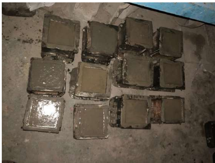
Figure 3.2: Casting of Cube Specimens
