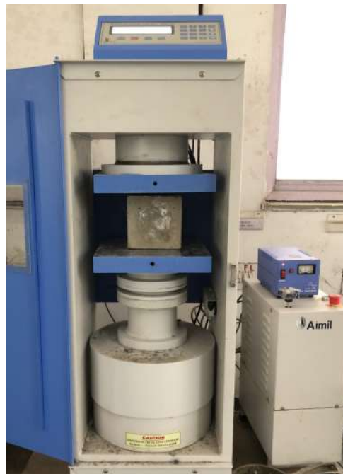
Figure 3.6: Cube Test In Compression Testing Machine
