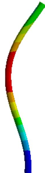
Figure 4.31: Buckled geometrical configuration of (8,8) BNNT
