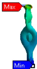
Figure 4.36: Buckled geometrical deformations after FEM eigen buckling analysis of (13,0) CNT
